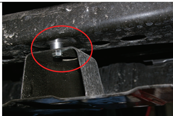
Install (2) skid plate spacers with new hardware
