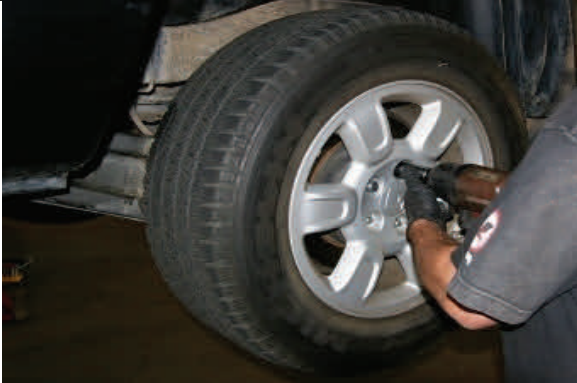
Raise and support vehicle frame on stands, remove wheels
