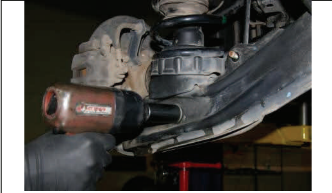
Unbolt lower strut mounting hardware
