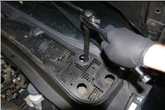
Under the hood remove upper strut mount access holes (3)
