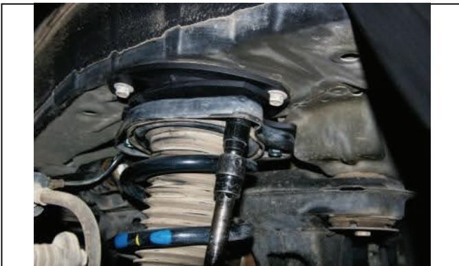
Reinstall strut into vehicle and attach with new nuts
