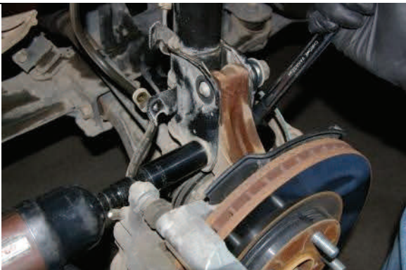
Support suspension with jack and unbolt strut from spindle
