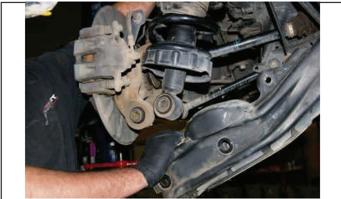
Push down lower control arm, lift strut up and out
