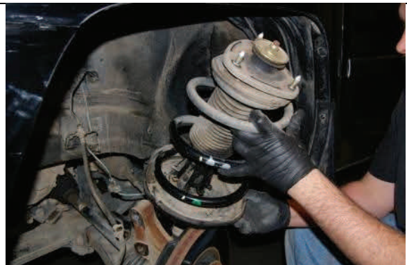
Lower suspension and remove strut. Caution: CV boot
