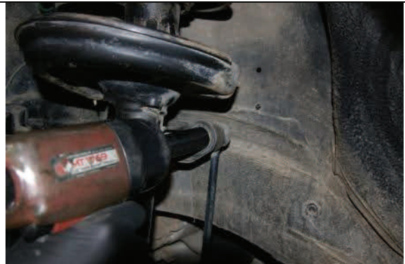
Disconnect and remove front sway bar end links
