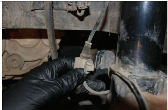
Unclip all ABS lines mounts on strut and at the frame
