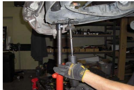
18. Reuse OE bushings and hardware top and bottom.
