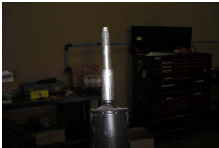
17. Install and tighten new upper shock extension.
