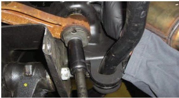
Remove passenger side differential mounting bracket
