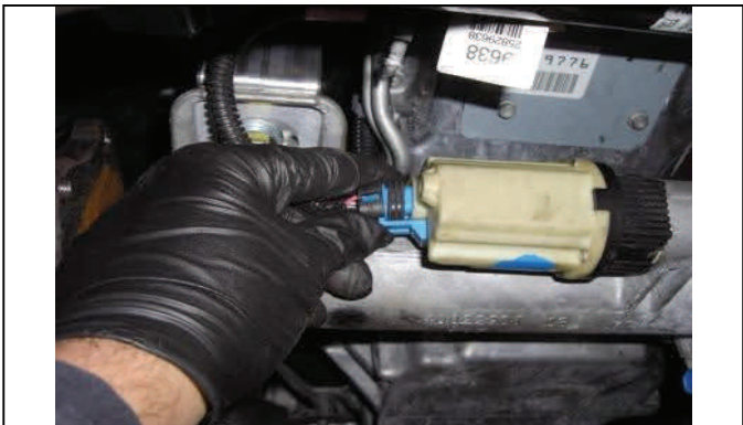
Reconnect differential solenoid
