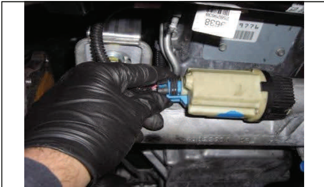
Unplug differential solenoid
