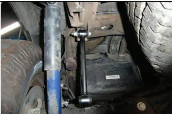
Install new longer sway bar end links and tighten
