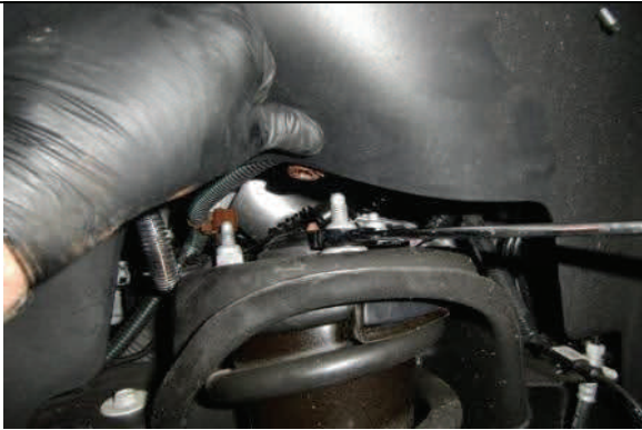
Remove upper mounting nuts
