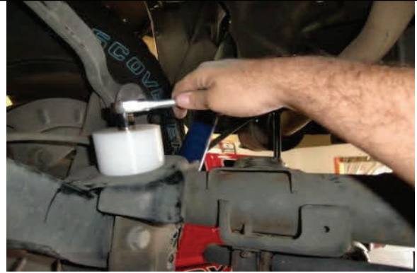
Use self-tapping bolt and attach bump stop extension
