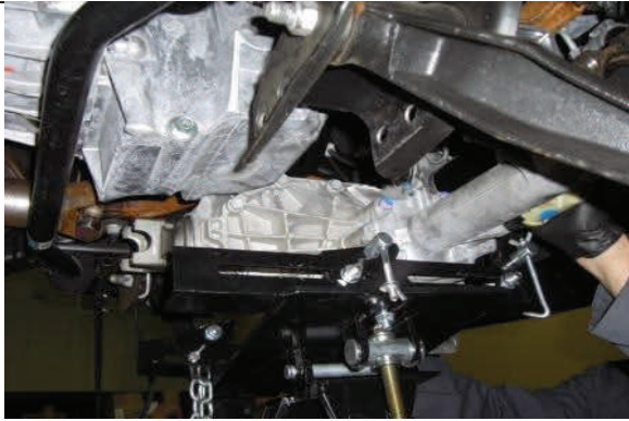
Carefully lower differential from vehicle
