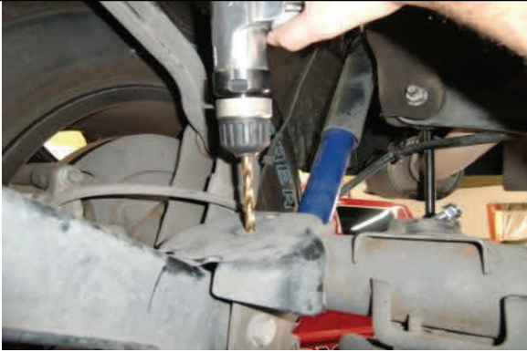
Mark center of bump stop pad and drill 11/32 hole
