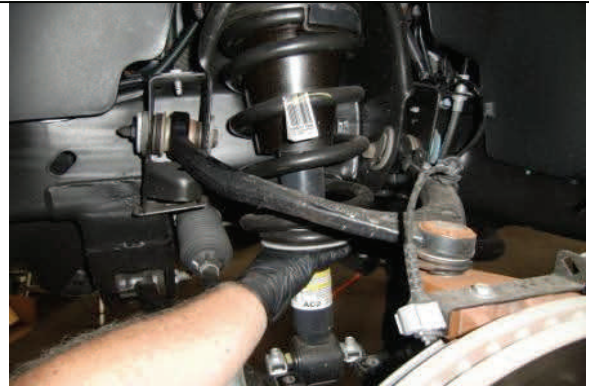
Remove strut assembly from vehicle.
