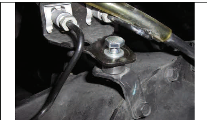
At the differential, install spacer and hardware as shown
