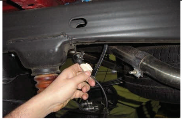
Unclips ABS/traction control lines at the frame
