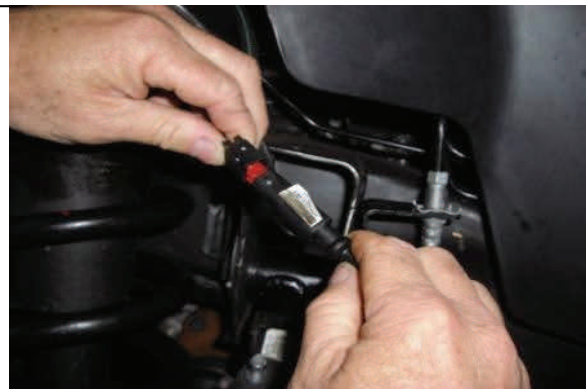
Reconnect ABS plug near frame
