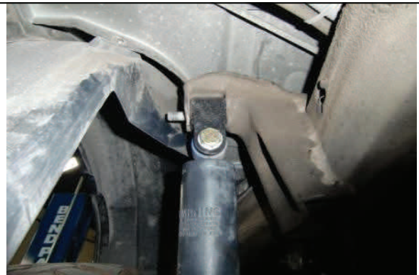
Reinstall shocks with extensions as shown and tighten
