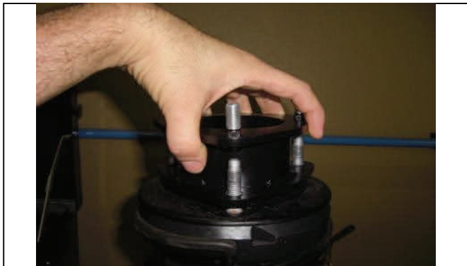
Place new strut extension spacer onto strut
