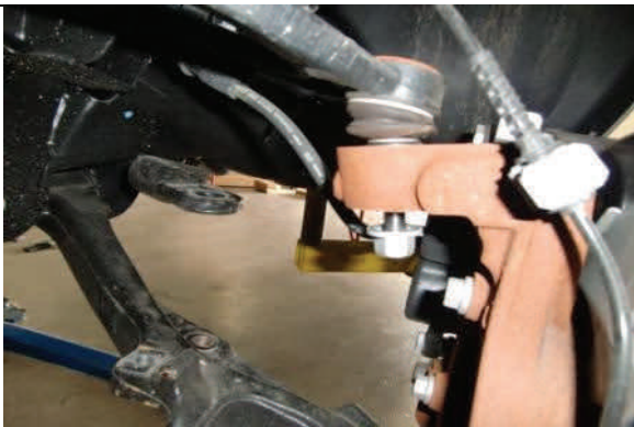
Loosen but do not remove upper ball joint nut
