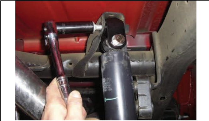
Reinstall shock with extension attached and tighten
