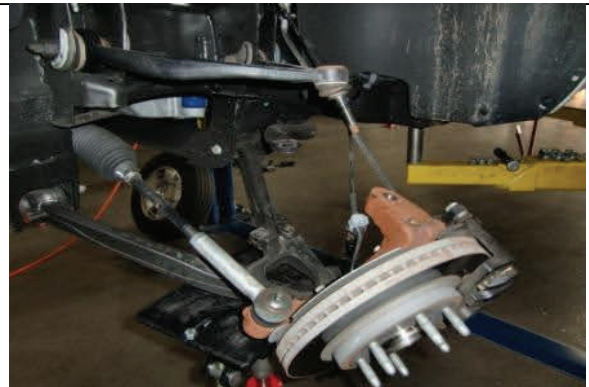
Carefully separate ball joint from spindle
