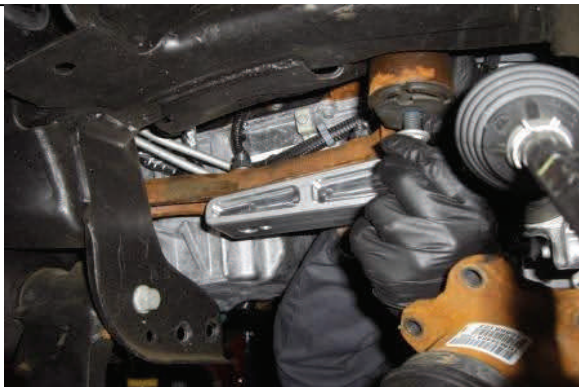
Reinstall bracket and attach billet spacer as shown
