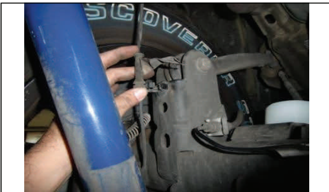
Disconnect ABS/TC line at the axle to avoid damage.
