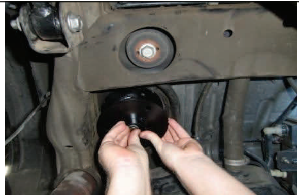
Attach coil spring spacer to nut plate and tighten
