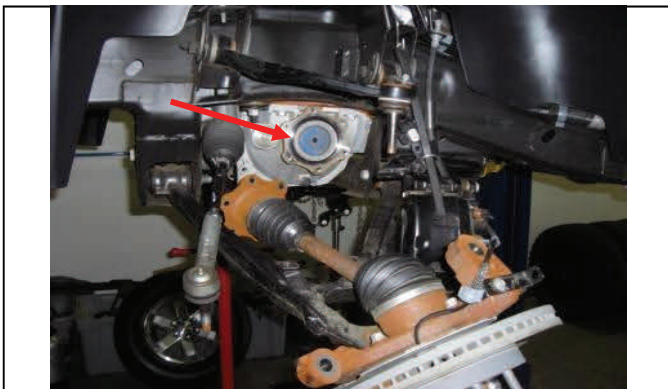
Unbolt CV axles (6) bolts at the differential
