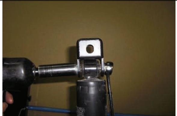
Install shock extensions to upper shock mount as shown
