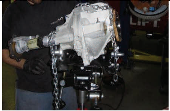
Secure differential to perform modification
