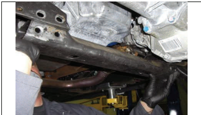
Reinstall rear cross member as original
