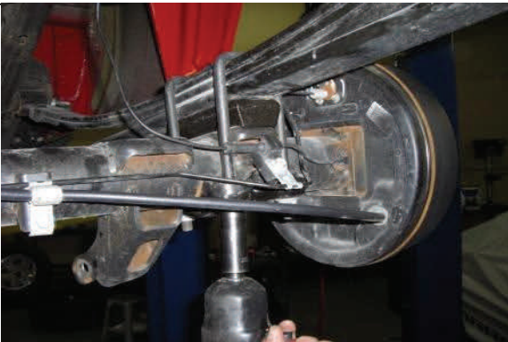
With axle supported remove u-bolts from axle
