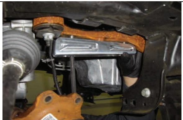
Attach passenger/driver side with socket head hardware
