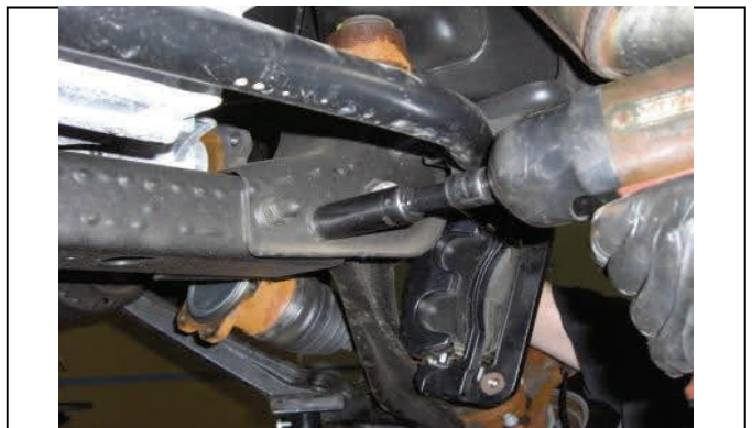
Unbolt rear cross member (4) bolts and remove
