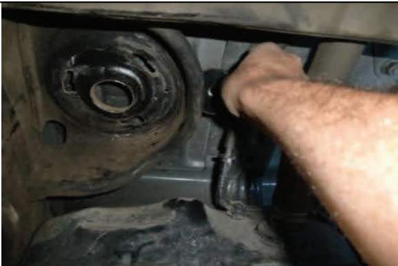
Place Upper coil spacer nut plate above coil housing
