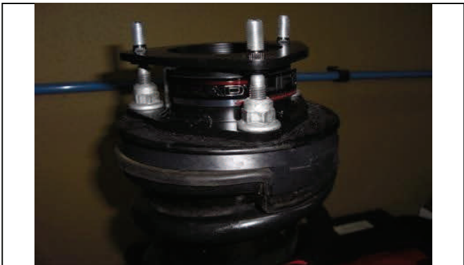
Attach and tighten with OE hardware
