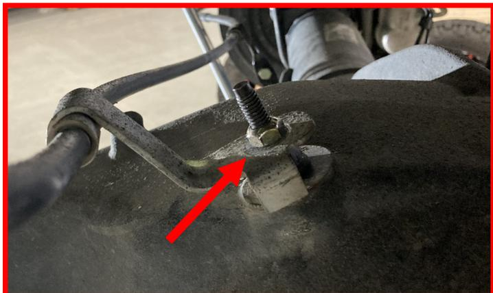
Install the **provided e-brake bracket extension** to the factory bracket with the **provided hardware**.
