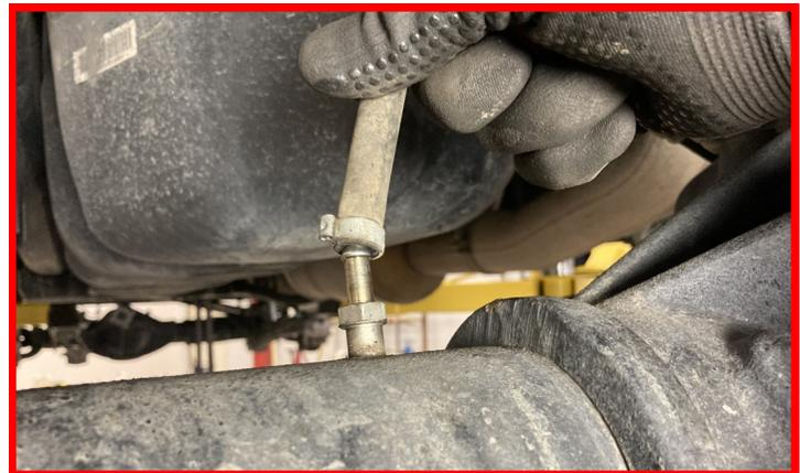
Remove the **e-brake cable stud** located on top of the differential housing. Once the cable is free re-install the stud.
