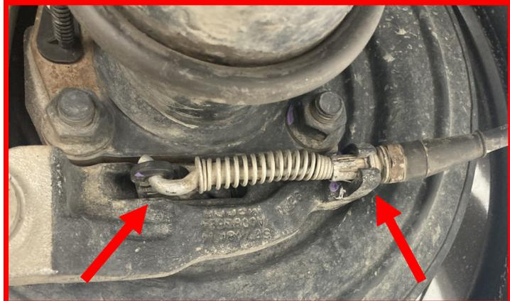
Tighten the e-brake adjustment bolt until you have the correct tension on the cable.
