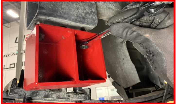
Install the bump stops using the **provided hardware**.
