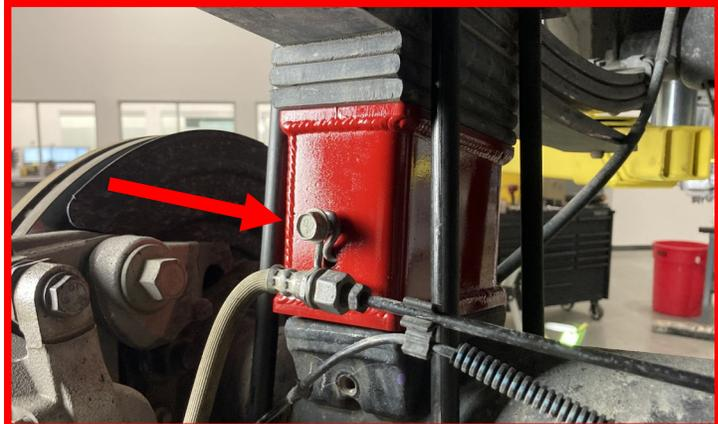
Install the **e-brake bracket** on top of the differential stud using the **provided hardware** to secure it down.
