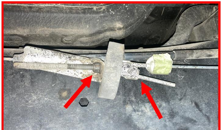
Remove the e-brake cable setup from the back of the rear driver side hub. You will need to unhook the cable hook attachment and also undo the clip that retains the cable housing itself.
