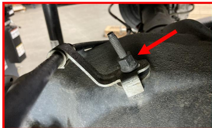
Remove the **e-brake cable bracket** near the passenger lower shock mount.
