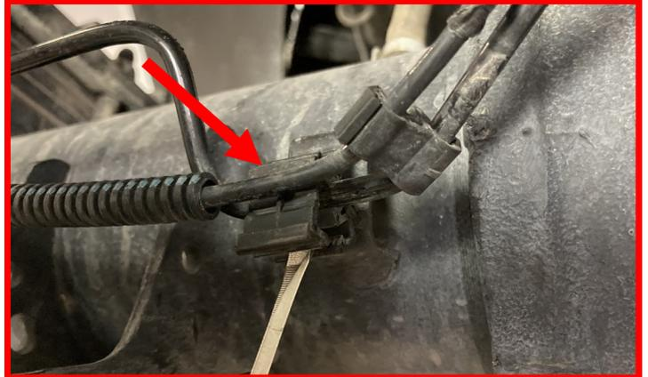
Remove the rear brake line/ wheel speed sensor bracket.
