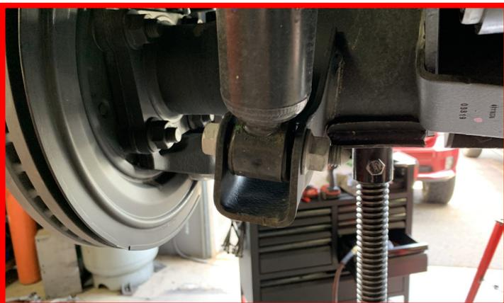
**Make sure the axle is properly supported before removing U-bolt nuts.**
