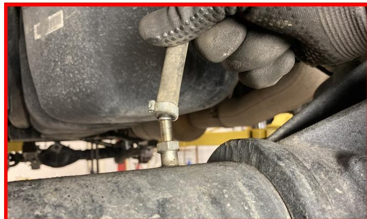
Remove the **e-brake cable stud** located on top of the differential housing. Once the cable is free re-install the stud.
