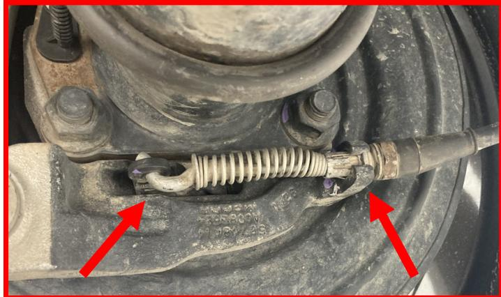
Tighten the e-brake adjustment bolt until you have the correct tension on the cable.
