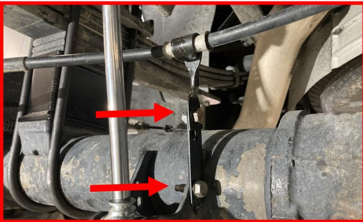
Install the now extended bracket to the factory location using the factory hardware.
