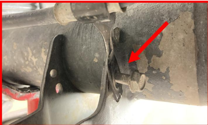
Remove both frame and axle **shock mounting bolts**. Remove shock from vehicle.
