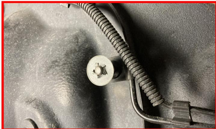
Remove the **brake line brackets** under each leaf spring.
