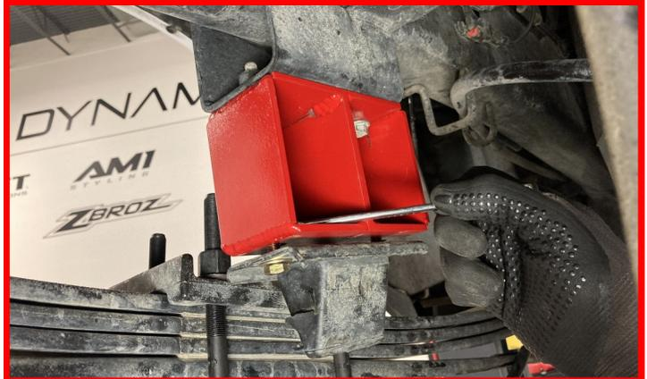
Loosen the **e-brake cable nut** located on the drivers side frame rail towards the rear of the vehicle.
