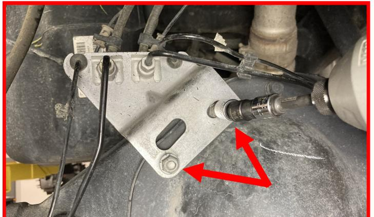
Remove the **brake line twist retainer** on the backside of the differential cover.
