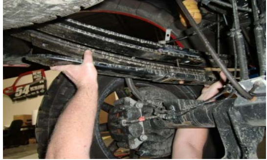
13. Install assembled leaves below main leaf pack.
