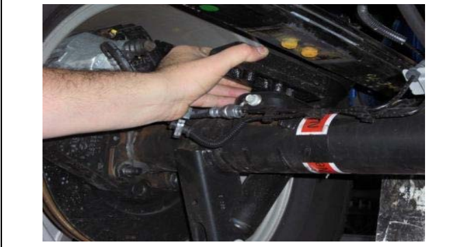
7. 4WD: Lower axle enough to remove factory block.
