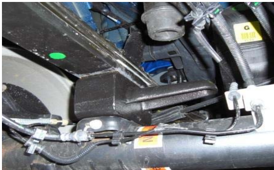
16. Raise axle and center on locating pins in leaf spring.
