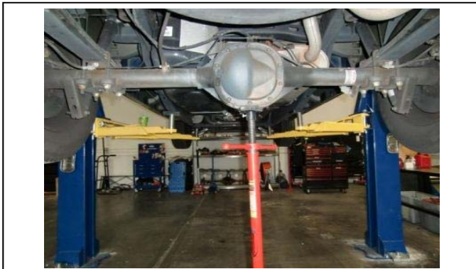
1. Raise vehicle at frame and support axle with jack.
