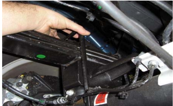
17. Place new longer u-bolts over leaf spring and axle.
