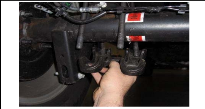
6. Remove lower u-bolt axle plate.
