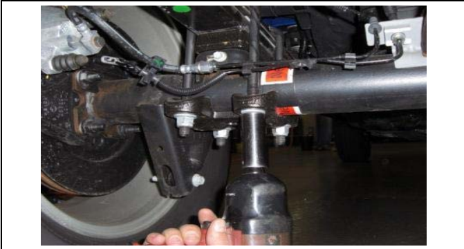
5. Loosen and remove factory u-bolt hardware.
