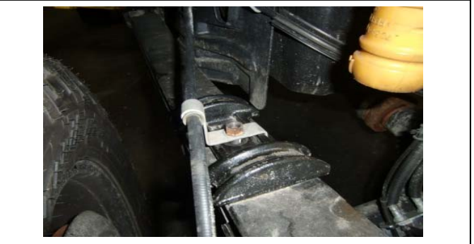
9. Remove e-brake bracket from upper u-bolt plate.
