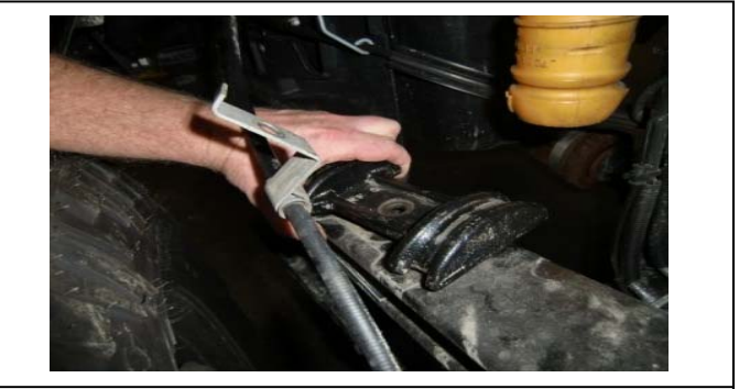
11. Remove upper u-bolt mounting plate and overload spring.
