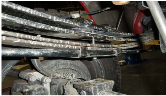
14. Clamp leaves together and torque centering pin(s).
