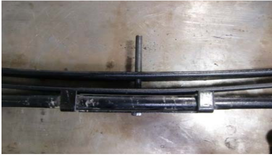
12. Place Add-A-Leaf above the overload spring, install new pin(s).
