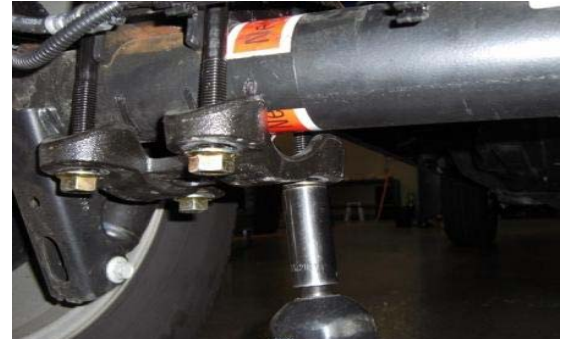
19. Snug hardware, lower vehicle on ground and torque.
