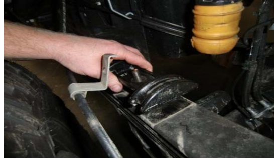
15. Place upper mounting plate on top of centering pin(s).
