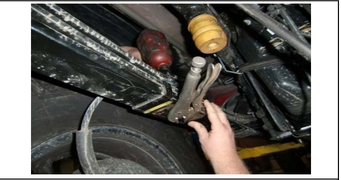
10. Clamp centering pin(s), loosen bolt supporting lower leaf.
