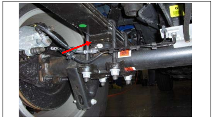
4. View of 4WD rear axle and leaf spring, note factory block.
