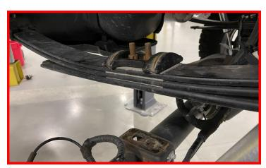
Install the provided lift block making sure the bump tang is facing inboard of the vehicle. Raise the axle and the block up to the spring while aligning the center pins.
