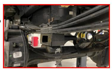
Install the provided u-bolts, and nuts. Snug the u-bolt nuts but do not fully tighten at this time.
