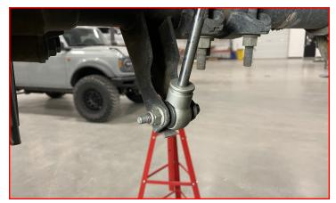
Prior to installing wheels, complete all installation steps on the opposite side. Install the wheels and lower the vehicle to the ground. Torque the lug nuts to the wheel manufacturers specs. Jounce the vehicle to settle the suspension to the new ride height. Torque the u-bolts to 110-ft/lbs and all shock hardware to 75-ft/lbs.
