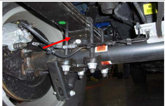
4. View of 4WD rear axle and leaf spring, note factory block.
