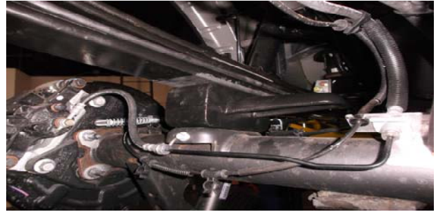
14. Raise axle up to engage lift block.
