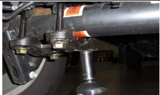
18. Snug hardware, lower vehicle on ground and torque.
