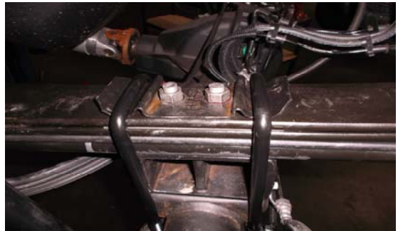
16. Be sure to locate the U-Bolts properly on top of Leaf Pack
