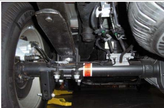
3. View of 2WD rear axle and leaf springs.
