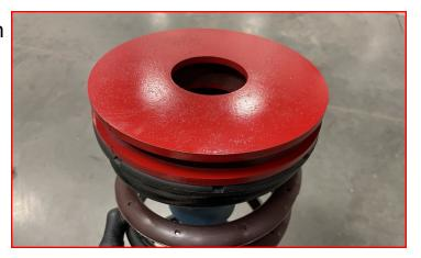
Insert the spring onto the axle.
