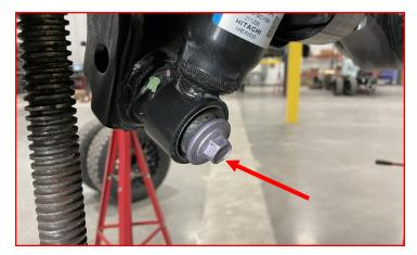
Remove the upper shock nut and bushing.
