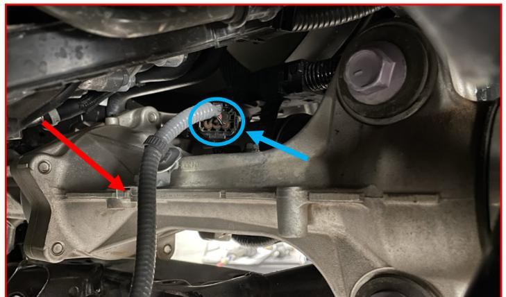
From the driver side wheel well, disconnect the **front differential vent hose** from the differential.
