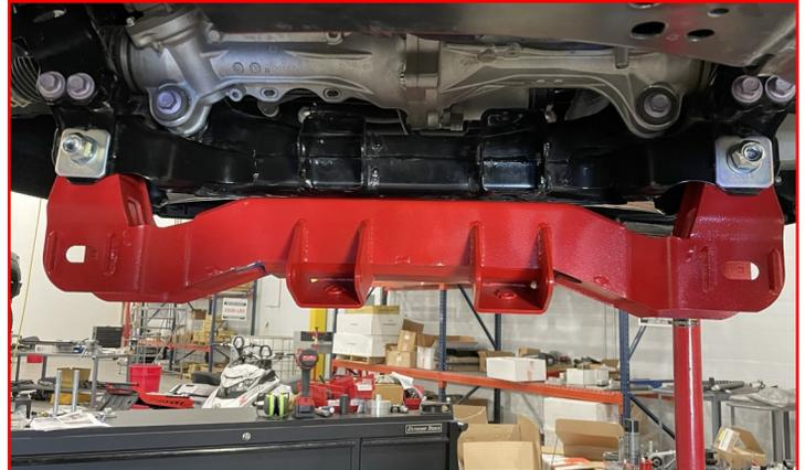
Raise the **front differential** and install the to the front crossmember using the **factory front differential mounting brackets** and **hardware**.
