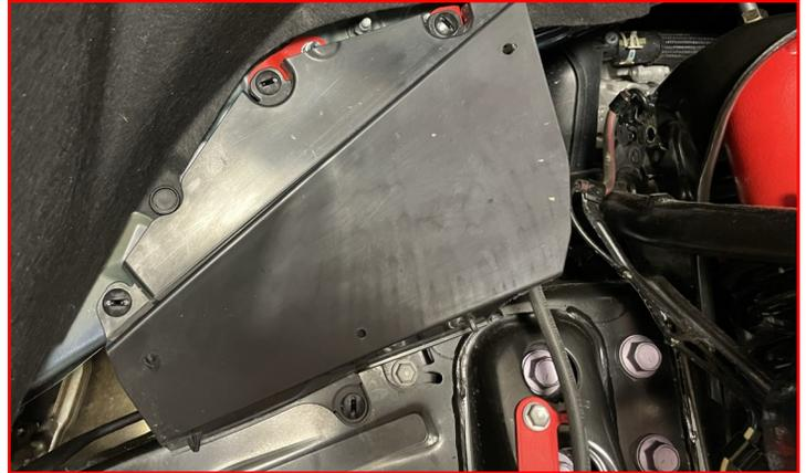
Using factory hardware, install the front sway bar drop brackets. Note that they are handed with the pockets facing inboard and the smaller mating faces towards the front of the vehicle.
