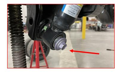
Remove the upper shock nut and bushing.
