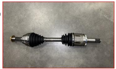
Insert the axle into the diff housing, be sure the splines are aligned prior to driving the axle in to place.
