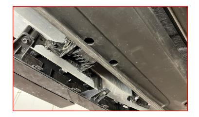
Using factory hardware, attach the front air dam to the chassis.
