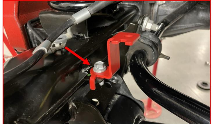
Using the supplied **M8-1.25 X 20mm hex head bolt**, **M8-1.25 locking nut**, and **two (2) M8 washers** attach the brake line to the **supplied bracket**.
