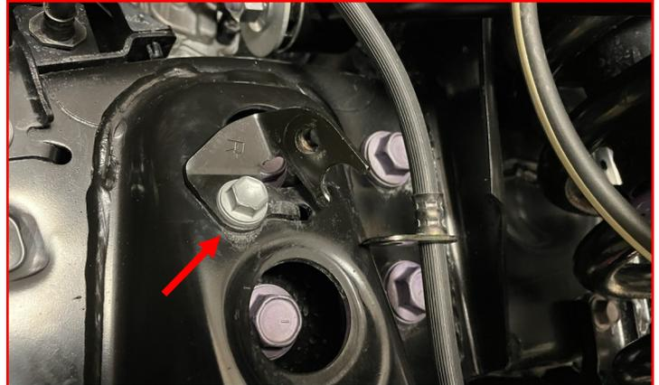
Attach the brake line to the **supplied brake line bracket** using **factory hardware** and the supplied **M8-1.25 locking nut** and **M8 washer**.
