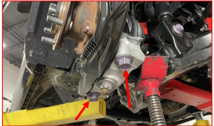
Torque the **axle nut** to **250 ft-lbs**.
