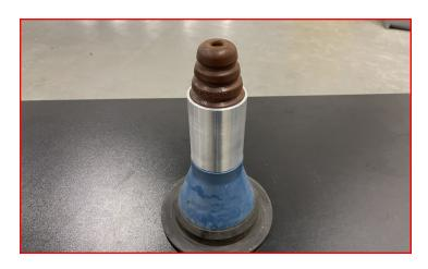
Place the factory bump stop and isolator on the top of the spring as shown.
