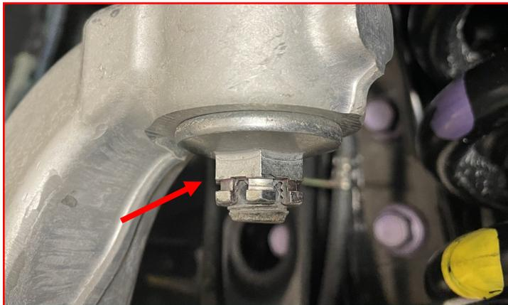
Remove the **cotter pin** and **castle nut** from the tie rod. Use the appropriate tool to release the taper.
