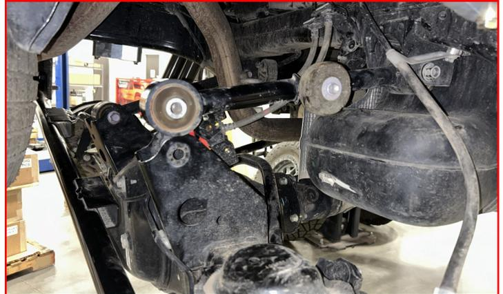
If equipped with headlight sensors on the rear upper control arms, disconnect sensor link from upper control arm, save link hardware for reinstallation. Mark around mounting bracket on upper control arm. Using a sufficient cutting tool, cut and remove mounting bracket. Clean the area thoroughly and paint the exposed metal with a good quality paint.
