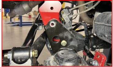
Note: The brackets can be installed on either side. The passenger side bracket shares the rear M14 mounting bolt with the trackbar relocation bracket.
