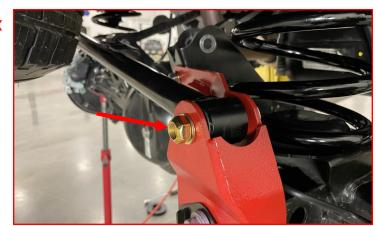
Install the rear ABS bracket between the brake line and the axle using the factory bolt (one on each side) holding the brake line to the axle.
