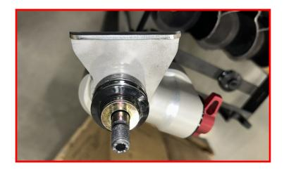
Install the Falcon rear shock and ensure the shock centering ring is located inside the large hole on the factory shock mount on the frame. Install the top bushing, washer, and nut. Tighten just enough to capture the shock centering ring within the frame mount.
