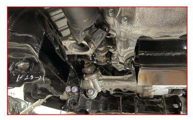
Temporally install the rear crossmember with the differential mount on the driver side. Use the supplied M18-2.5 X 160mm hex heads bolts and cam block off plates (four total).
