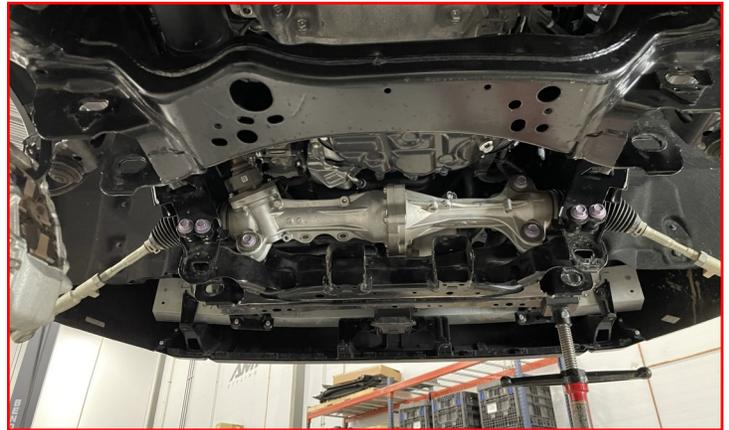
On the backside of the rear crossmember, mark a **vertical line 2.5 inches** from the **center** of the left hand side **alignment cam hole**.
