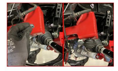
Due to frame variances, it may be necessary to trim an OE frame bracket to allow clearance for coil. Using a suitable cutting tool, (abrasive cutoff wheel, Sawzall, etc.) trim bracket for adequate clearance. After trimming the bracket, clean the area thoroughly and paint the exposed metal with a good quality paint.
