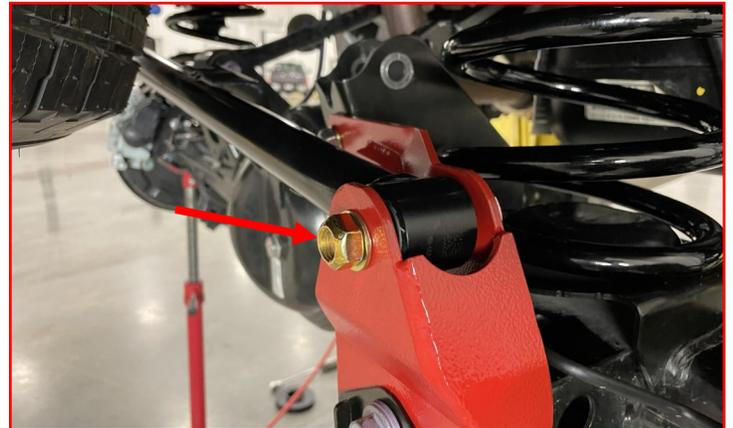
Install the **rear ABS bracket** between the brake line and the axle using the **factory bolt** (one on each side) holding the brake line to the axle.
