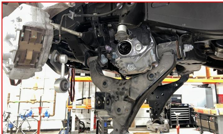
Locate the replacement axle assembly. The axle are etch with the part number on the shaft. The **68-52420CVL** is the Left (driver) side and will be the shorter of the two.
