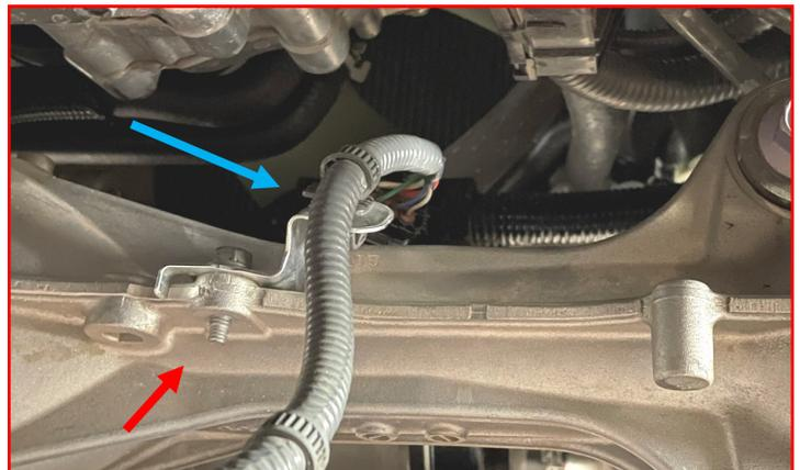
Attach the **supplied differential vent hose** to the front differential using the **factory hose clip**.
