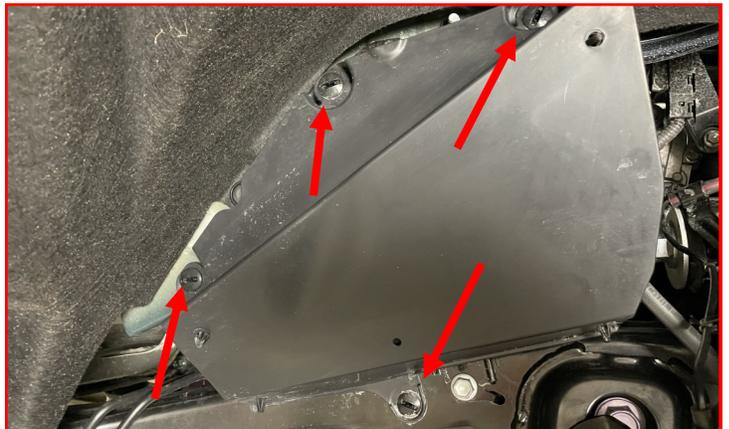
Install the four (4) clips for the front dust shield.
