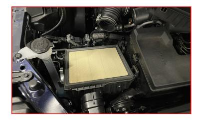
Slide the air box lid into the intake hose and clip it to the air box.
