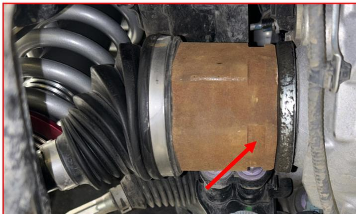
**DO NOT TRY TO PRY THE AXLE FROM THE DIFF HOUSING, THIS WILL DAMAGE THE HOUSING AND SEAL.**
