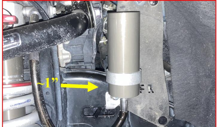
Use the factory hardware to attach the lower control arm to the Falcon coilover.
