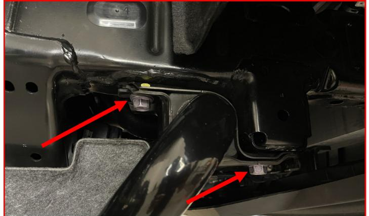
Remove the **ABS wire bracket** on the upper control arm and strut perch.
