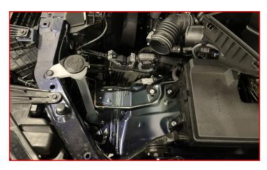
Remove the three (3) bolts holding the accumulator to the body.
