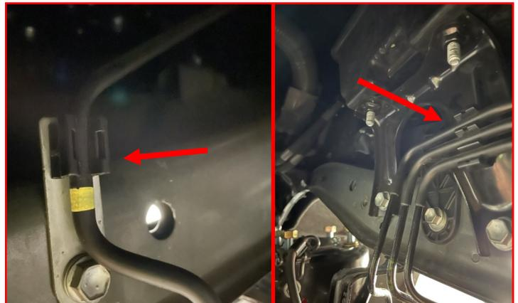
Attach the **supplied front brake line bracket 2** (left and right) to the body using **factory hardware**. Attach the factory brake line bracket to the **supplied bracket** using the **supplied M8-1.25 X hex head bolt**, **M8-1.25 locking nut**, and **four (4) M8 flat washers**.
