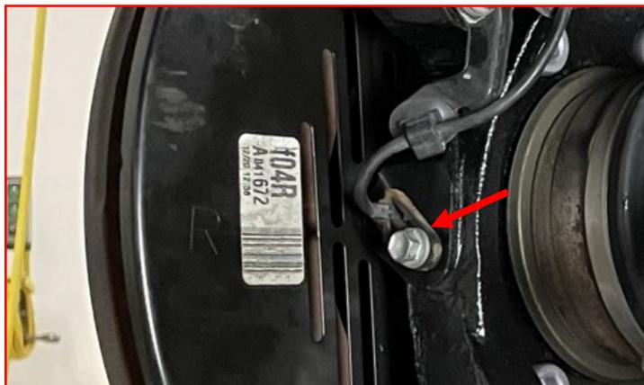
On the factory dirt shields removed on page 8, remove the retaining clip for the sound deadening in the front lower corner.
