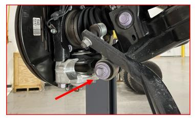
Using the supplied M12-1.75 X 50 bolt, locking nuts, and flat washers, attach the sway bar to the sway bar brackets.
