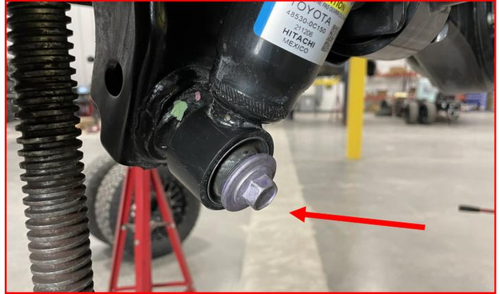
Remove the **upper shock nut** and bushing.
