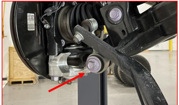
Using the **supplied M12-1.75 X 50 bolt, locking nuts, and flat washers**, attach the sway bar to the **sway bar brackets**.
