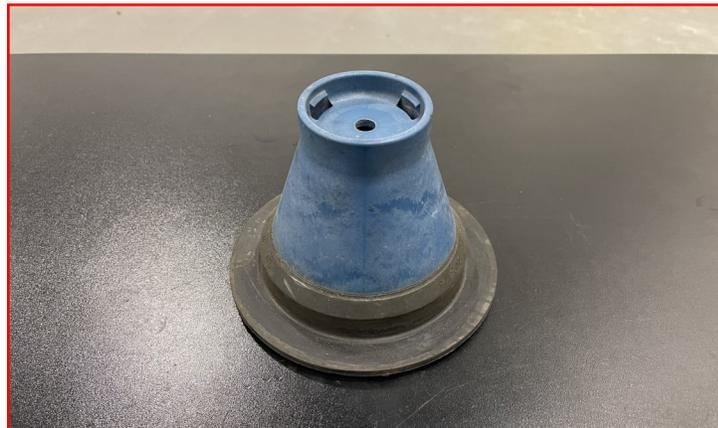
Install the supplied rear bump stop extension onto the factory isolator.
