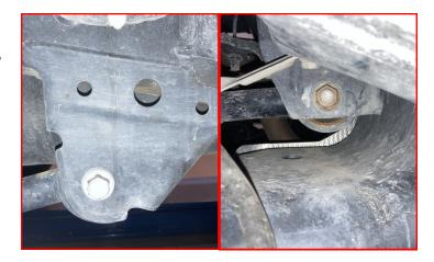
Remove rear driveshaft loop. Install driveshaft loop spacers from hardware pack between loop and frame using OE hardware. Torque to factory spec.
