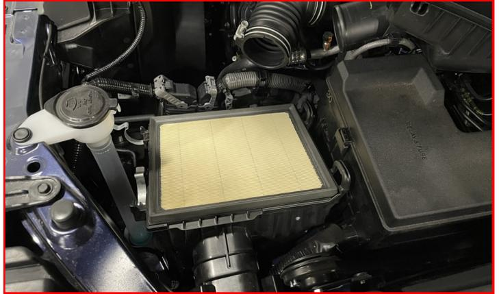
Slide the air box lid into the intake hose and clip it to the air box.
