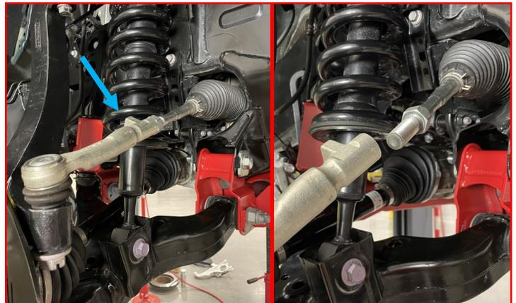
Note how the **nub** on the tie rod is opposite of the factory location in the previous step.
