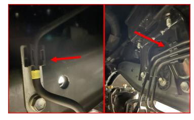
Attach the supplied front brake line bracket 2 (left and right) to the body using factory hardware. Attach the factory brake line bracket to the supplied bracket using the supplied M8-1.25 X hex head bolt, M8-1.25 locking nut, and four (4) M8 flat washers.
