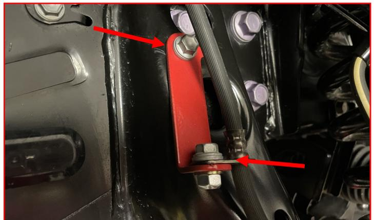
Attach the ABS wire to the strut perch using **factory hardware**.
