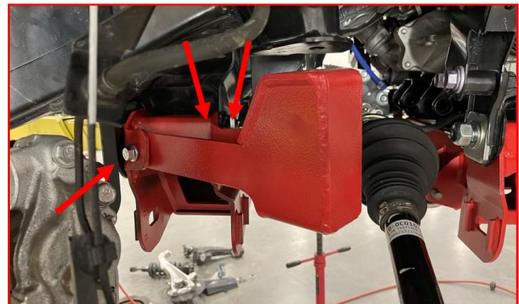
Use a **supplied M10-1.25 X 25 hex head flange bolt** to attach the bump stop to the chassis.
