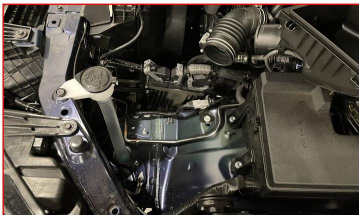
Remove the three (3) **bolts** holding the accumulator to the body.
