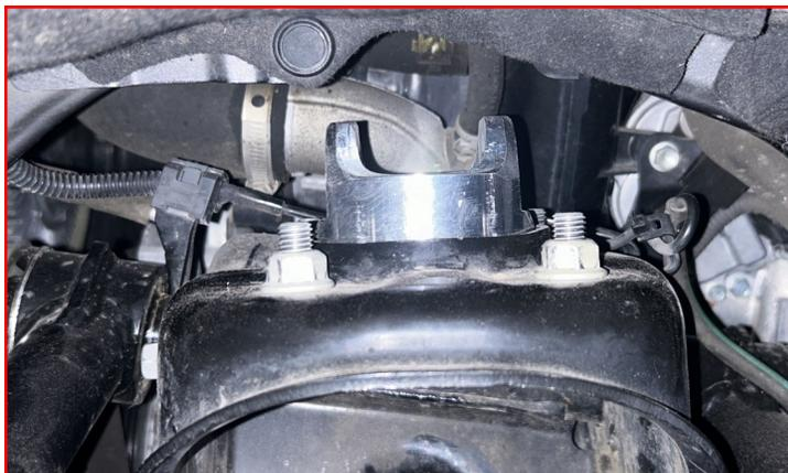
Install the falcon front coilover by installing the supplied M16 bolt and nut through the top hat.
