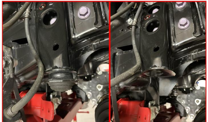
Using the **supplied M10-1.25 X 25mm hex head flange bolts (3)** and **M10-1.25 flange nuts (3)**, attach the front bump stops to the rear crossmember. Note: the long flange goes towards the rear of the vehicle.
