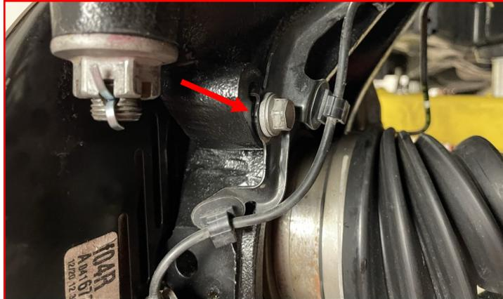
Using **factory hardware**, attach the ABS/wheel speed sensor.
