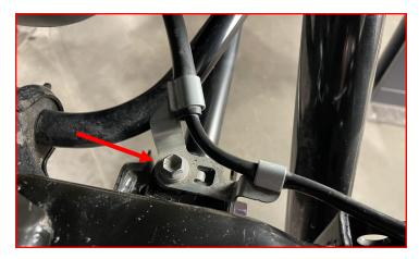
Remove the **bolt** (one on each side) holding the brake line to the body.
