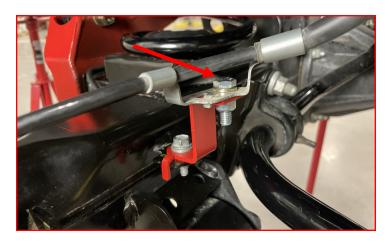
Install the rear ABS relocator between the brake lines and the axle using the factory bolt holding the brake line to the axle.
