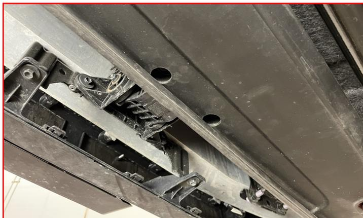
Using **factory hardware**, attach the front air dam to the chassis.
