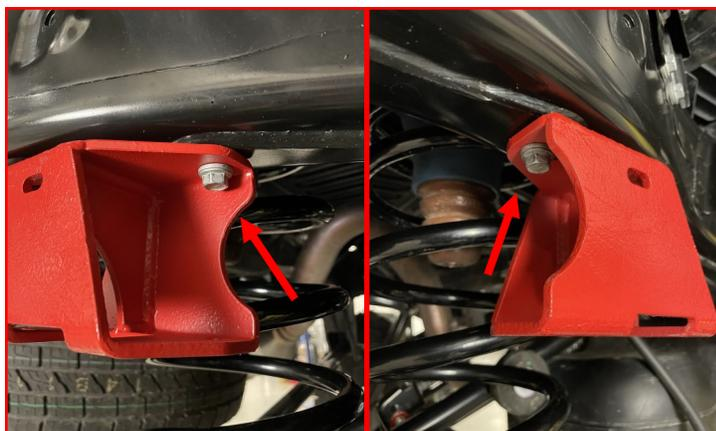
Attach the factory bump stop to the extension using the supplied **M8-1.25 X 20mm hex head bolts** and **M8 flat washers**, starting with the lower bolts.
