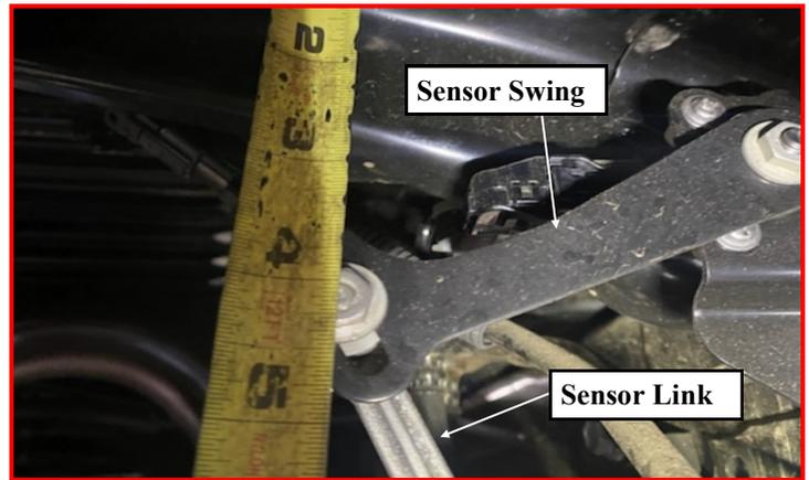
Using the sensor link hardware, and previously removed M8 bolt from the front skid plate, install headlight sensor relocation bracket (90-13800) from hardware pack (90-60866). Install sensor link on the furthest hole for 6" kits.
