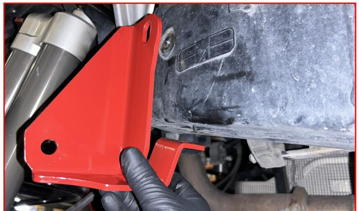
Attache the sway bar link to the drop bracket using the factory nut.
