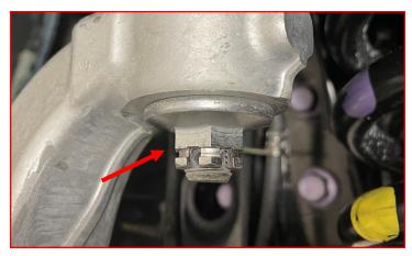
Remove the cotter pin and castle nut from the tie rod. Use the appropriate tool to release the tapper.
