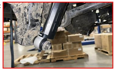
Using the supplied M14-2.00 X 90mm hex head bolt, M14-2.00 locking nut, and two (2) M14 washers attach the factory Panhard bar to the track bar bracket.
