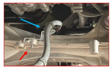
Attach the supplied differential vent hose to the front differential using the factory hose clip.
