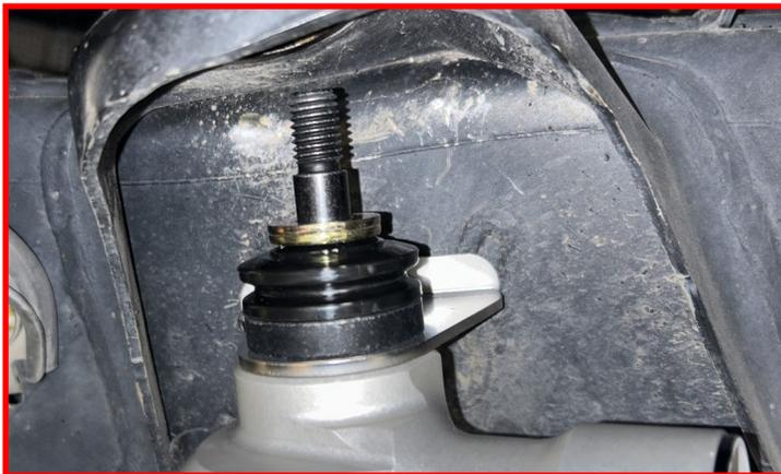
Second photo to help with orientation of anti-rotation plate.
