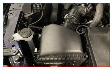
Plug the MAF sensor back into its housing.
