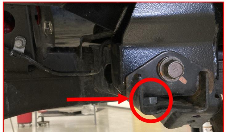
Using the factory control arm hardware and the supplied M14 hardware, install the Geometry Correction Bracket on the passenger side.
