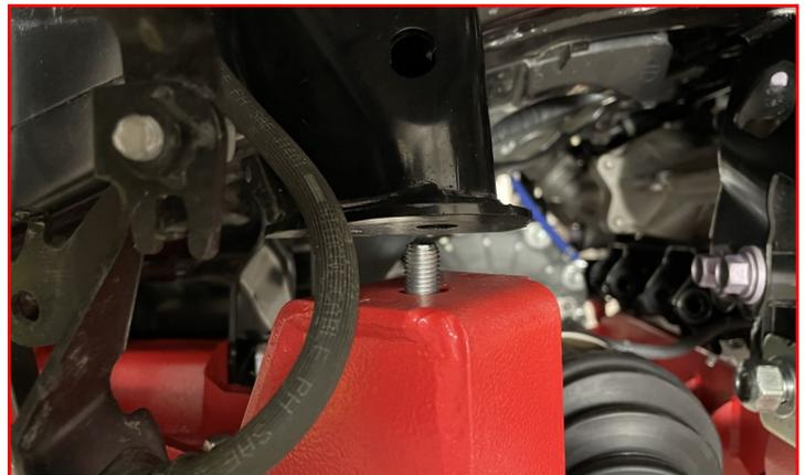
Torque the **chassis to differential drop bracket hardware** to **110 ft-lbs.**
