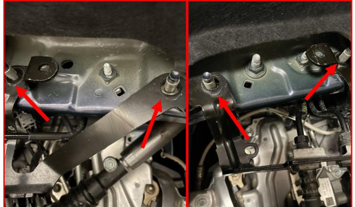
Remove the driver side brake lines from the plastic clip on the inside of the body panel opposite of the bracket removed in the previous step (left image).
