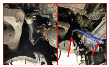
Install the front crossmember using the supplied M18-2.5 X 140mm hex head bolts, M18-2.5 lock nuts, M18 flat washers (4), and cam block off plates (4). Install the bolts from front to rear
