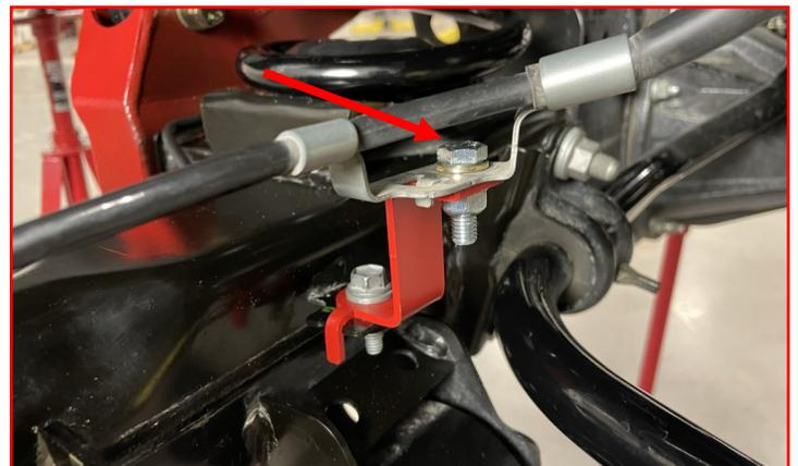
Install the **rear ABS relocater** between the brake lines and the axle using the **factory bolt** holding the brake line to the axle.
