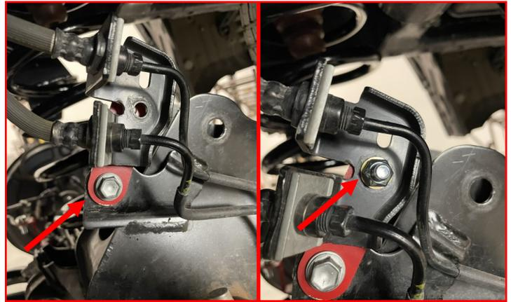
Install the **rear ABS relocater** between the brake lines and the frame using the **factory bolt** holding the brake line to the frame.
