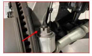
Remove the CV axle dust shield.
