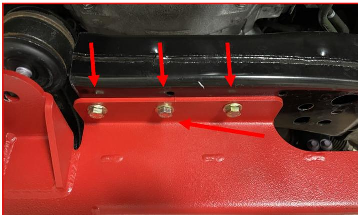
Use factory hardware to attach the rear front differential mount to the rear crossmember.
