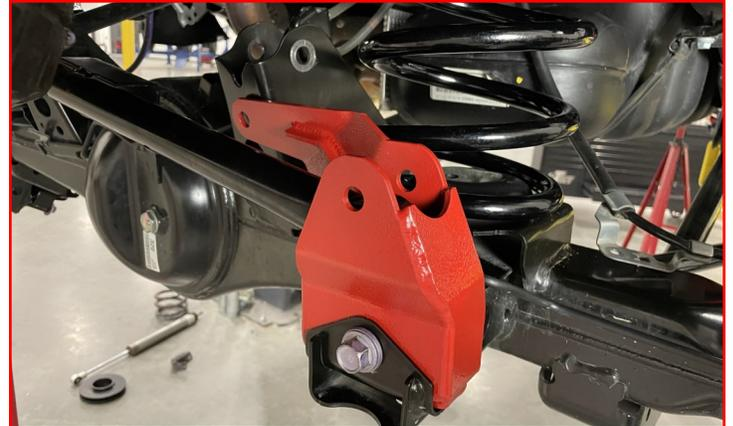
Use **two M12 washers** under the head of the **M12 Allen Head bolt** with the supplied **locking nut** inserted in the bottom side of the OE bracket. **DO NOT TIGHTEN**
