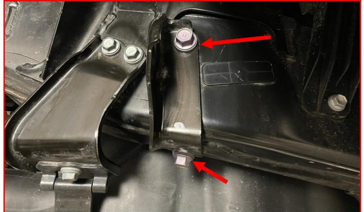
Install the **sway bar drop bracket** using the **factory hardware**.
