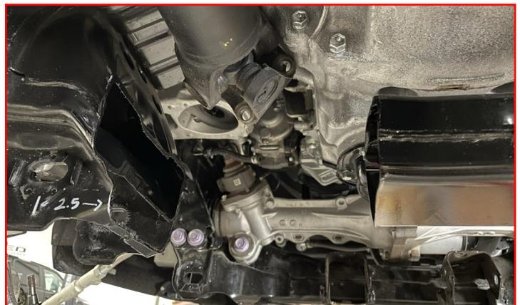
Temporarily install the **rear crossmember** with the differential mount on the driver side. Use the **supplied M18-2.5 X 160mm hex heads bolts** and **cam block off plates** (four total).
