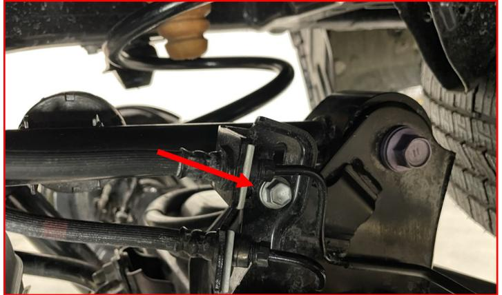
Remove the **end link nut** and let the end link hang out of the way.
