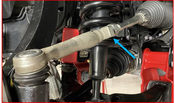
Using factory hardware, attach the tie rod to the knuckle from the top.
