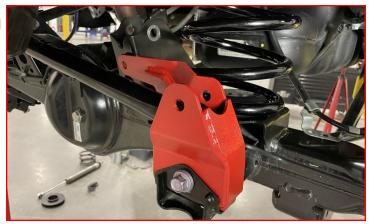
Use two M12 washers under the head of the M12 Allen Head bolt with the supplied locking nut inserted in the bottom side of the OE bracket. **DO NOT TIGHTEN**
