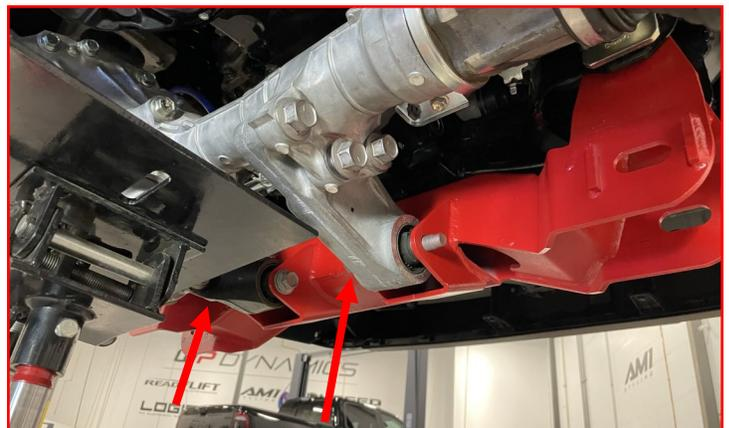
Install the rear crossmember using the supplied M18-2.5 X 160mm hex head bolts, M18-2.5 locking nuts, and M18 flat washers,
