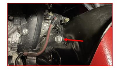
Using factory hardware, attach the ABS sensor wire at the middle of the knuckle.
