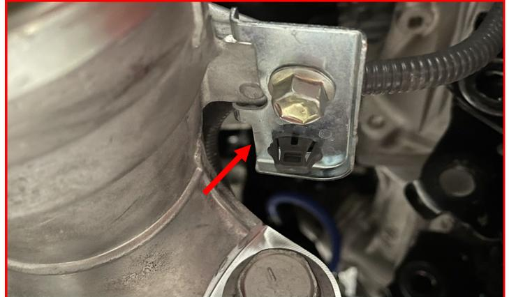
Plug the **harness** into the factory plug location. Attach the **harness** to the steering rack using **factory hardware** (right image).
