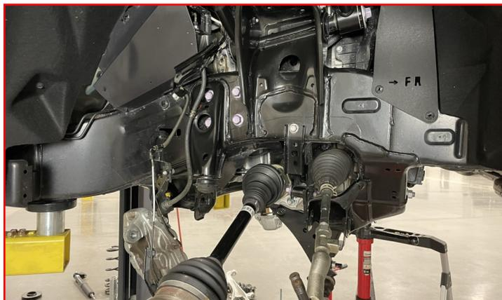
Remove the **four (4) nuts** holding the drive shaft to the front differential.
