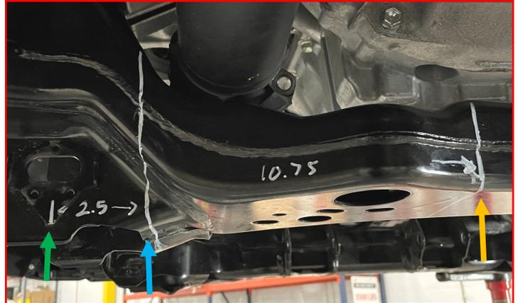
Using a suitable cutting tool, cut the crossmember at the marked lines.
