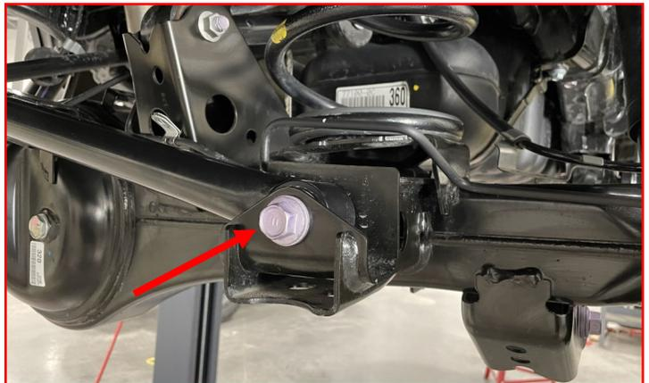
Loosen but **DO NOT** remove the **DRIVER upper control nut** at the axle.
