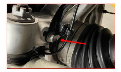
Using a trim removal tool, remove the four (4) clips for the front and rear plastic dirt shields.
