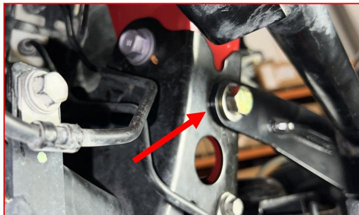
Using the supplied M14x100mm bolt, washers, and nut, attach the upper control arm to the geometry correction bracket.
