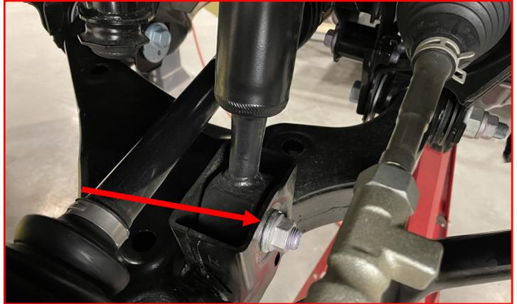
Loosen but **DO NOT** remove the four (4) **upper strut bolts**.
