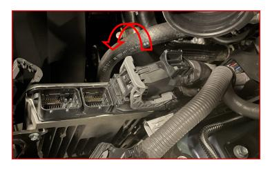
Plug the center plug into the accumulator and lock it in place by closing the handle to the right.
