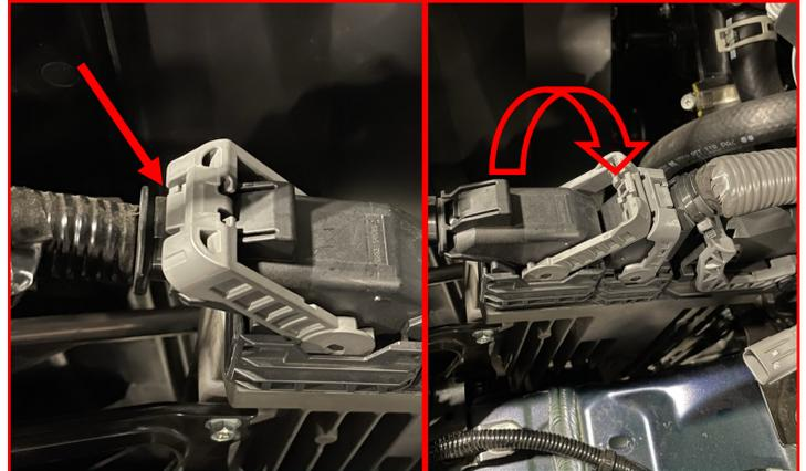
Release the hose clip on the middle plug by pressing in on the **tabs** on both side and lifting up.
