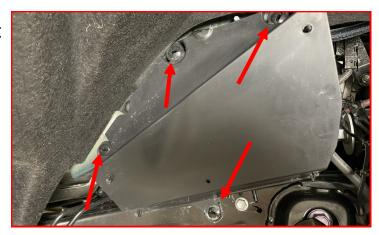
Install the four (4) clips for the front dust shield.
