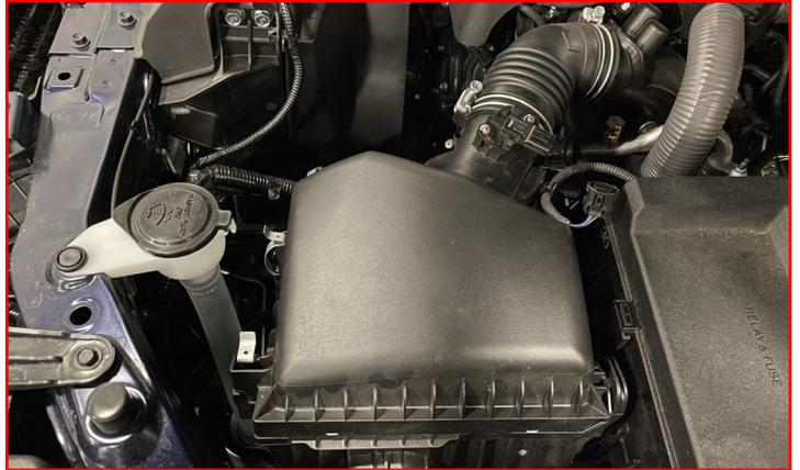
Plug the **MAF sensor** back into its housing.
