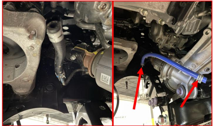
Install the **front crossmember** using the **supplied M18-2.5 X 140mm hex head bolts**, **M18-2.5 lock nuts**, **M18 flat washers (4)**, and **cam block off plates (4)**. Install the bolts from front to rear
