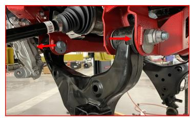
Remove the factory bump stop from the chassis mount.
