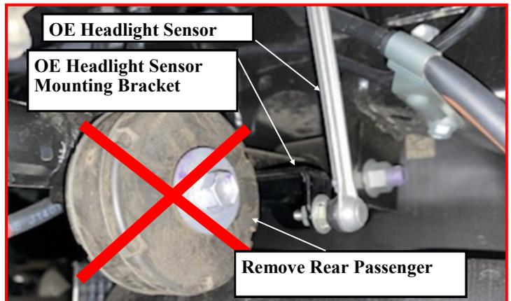
Remove rubber bumper from passenger side only to allow for full droop without contact of bumper and gas tank. Measure from bottom of the swing arm on sensor vertically to the frame. Should be about 4 3/16" at ride height. See Photos 31 and 32.
