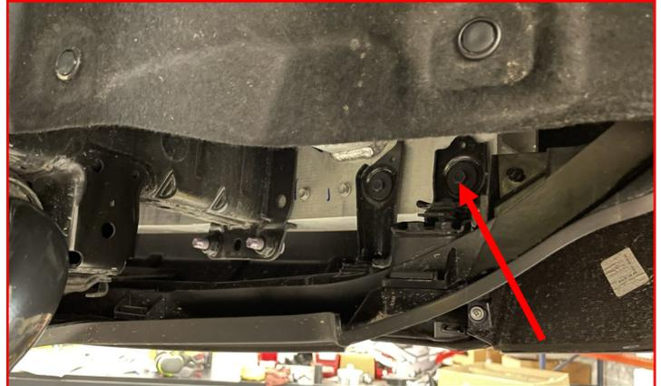
Remove the two (2) **screws** retaining the factory air dam to the actuator.
