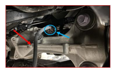
From the driver side wheel well, disconnect the front differential vent hose from the differential.
