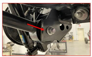
Loosen but **DO NOT** remove the lower and upper control arm nuts at the frame.
