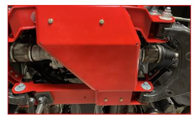
Using factory hardware, install the factory front dust shield.
