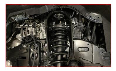
Using factory hardware (installed front to back), install the ReadyLift upper control arm.
