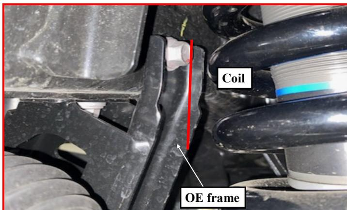
Install the **Falcon top hat assembly** using the **supplied nuts**.
