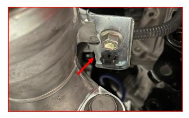
Plug the harness into the factory plug location. Attach the harness to the steering rack using factory hardware (right image).
