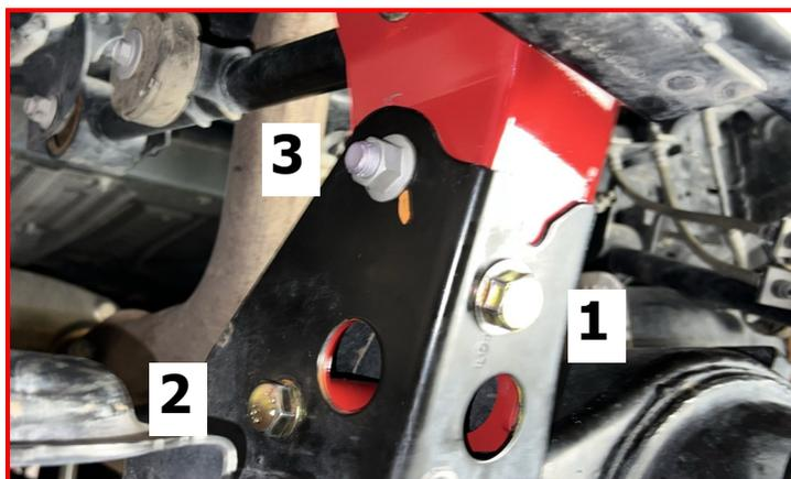
Remove the factory bump stop from the factory spring isolator.
