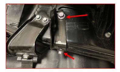
Install the sway bar drop bracket using the factory hardware.
