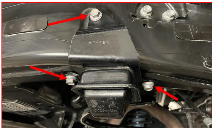
Attach the **supplied bump stop extension** to the frame with **factory hardware** in the bottom holes.
