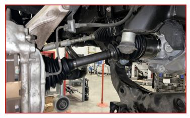
Remove the **bolt** holding the **front** differential control plug to the front differential (left image).
