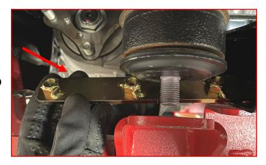
Use the supplied 3/8-16 X 1in hex head bolts and 3/8-16 flat washers to secure the rear crossmember to the chassis.
