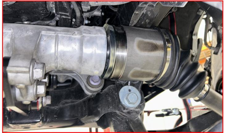
Install the outer splines through the hub assembly, in the factory orientation.
