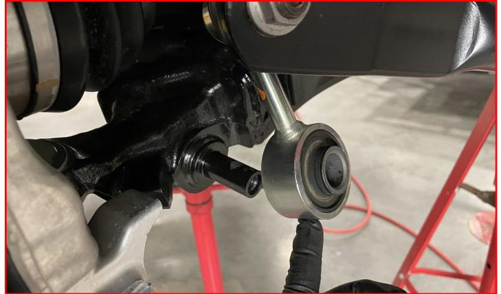
Remove the four (4)(two on each side) **sway bar bolts** and remove the sway bar from the vehicle.
