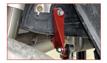
Remove the three bolts holding the bump stomp to the frame.
