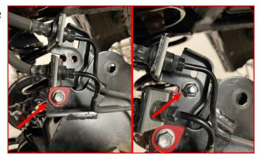
Install the rear ABS relocator between the brake lines and the frame using the factory bolt holding the brake line to the frame.
