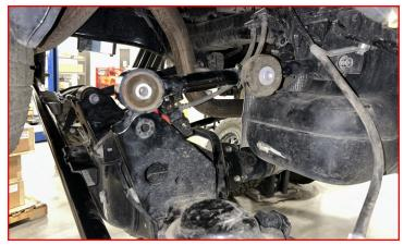
If equipped with headlight sensors on the rear upper control arms, disconnect sensor link from upper control arm, save link hardware for reinstallation. Mark around mounting bracket on upper control arm. Using a sufficient cutting tool, cut and remove mounting bracket. Clean the area thoroughly and paint the exposed metal with a good quality paint.
