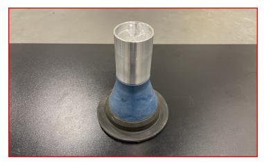
Attach the supplied bump stop extension to the factory isolator using thread locker and the supplied M10-1.5 X 25mm hex bolt and M10 washer.
