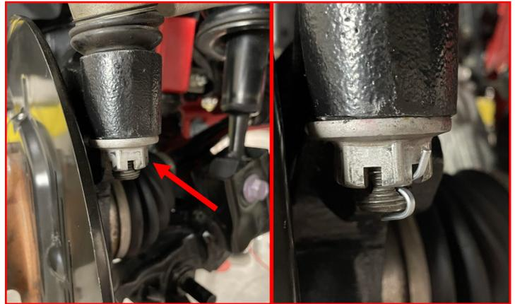
Remove the **two (2) nuts** holding the brake line bracket to the body (driver shown in the left image, passenger shown in the right image).
