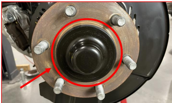
Remove the **cotter pin**, **sleeve**, and **nut**.
