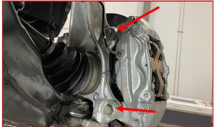
Remove the factory brake line bracket from the chassis.
