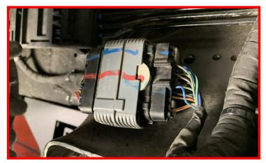
With the connector out of the way, install the connector relocation bracket using the provided M6 hardware.
