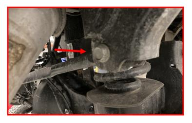
Remove the rear track bar bolt at the axle side.
