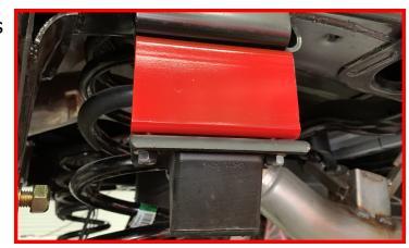
Remove the factory sway bar end link upper hardware.
