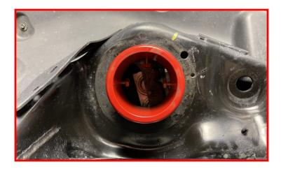
Install spring isolator over the retainer, ensure the alignment tab is installed into new clocking hole.
