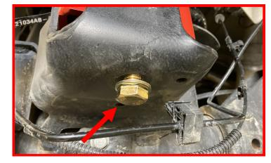
Install the track bar into the top hole on the track bar bracket using the provided M14 bolt.
