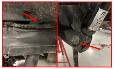
Lower the axle down until you have enough room to install the provided spring.
