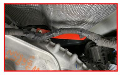
Install the transfer case shift solenoid connector.
