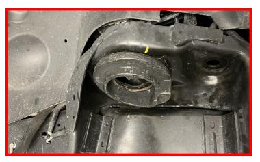
Install the provided coil springs with factory isolators on top. Make sure the isolator is positioned on the flat end of the coil spring. Lower the axle low enough to set both springs in place.
