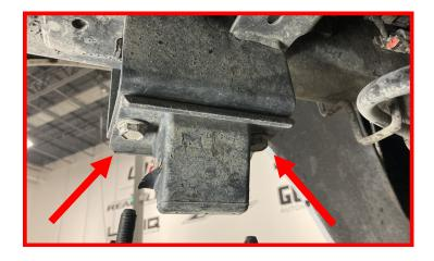
Install the provided bump stop extensions onto the frame using the factory hardware.
