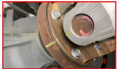
To remove the rear driveshaft, carefully slide the slip yoke out of the tail shaft housing on the transfer case. Take care not to damage the slip yoke or tail shaft boot when handling the driveshaft.
