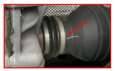
Using the appropriate pliers, spread open the retaining clip and slide the front driveline off the splines.
