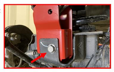
Install provided M14 bolt into the bottom of the rear track bar bracket.
