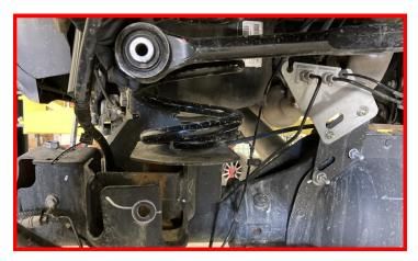
Remove the rear brake line/ wheel speed sensor bracket.
