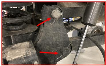
Loosen the rear track bar bolt at the frame side.
