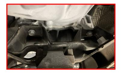
Tighten the transmission mount bolts.
