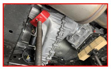
Install the transmission mount using the (4) factory bolts.
