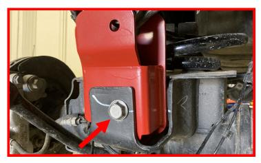
Plug factory brake line retaining plug back in.
