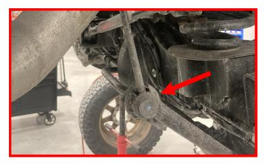
Install the provided sway bar end link upper using the provided hardware.
