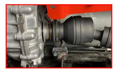
Install the provided clamp onto the dust boot and joint housing.
