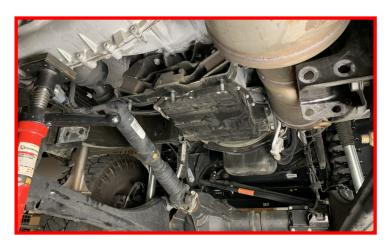
The transmission mount is attached with (4) bolts. Remove the (2) bolts located at the rear of the mount.
