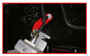
The passenger side bracket will angle around the frame gusset.
