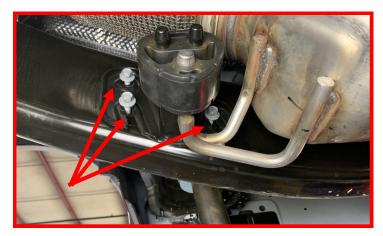
Make sure that the factory radius arm bolt is still loose to aid in the removal of the transmission crossmember.
