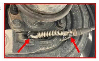
Once the cable is loose you will be able to back-feed the cable through the first frame rail hole you see.
