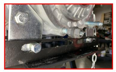
Option 2: Using the splines and an appropriate socket, unthread the stud.
