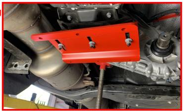
Ensure that the provided crossmember mount is installed with the slope facing towards the rear of the vehicle.
