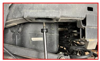
Install the rear Falcon shocks into the axle mounts using the factory bolt.
