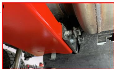
Install (3) provided M12 bolts, (3) locking nuts and, (6) flat washers through the rear holes on the transmission mounting plate, mounting plate spacer and the transmission crossmember.
