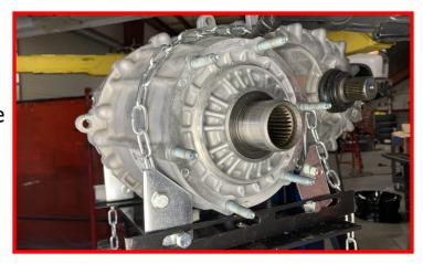
Once the transfer case is removed from vehicle, remove the factory mounting studs. There are two ways to remove the studs.
