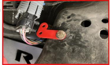
Install the harness connector onto the relocation bracket.
