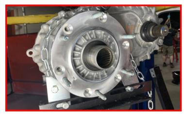
Install the supplied M10 flat head bolts using thread locker.
