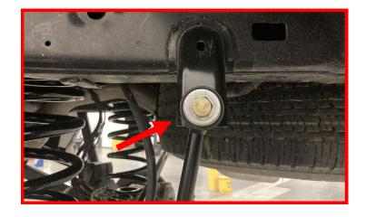
Install the provided sway bar end link lower using the provided hardware.
