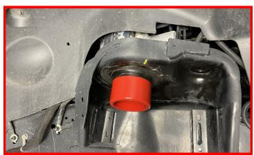
Tighten the (3) 5/16" bolts until tight. Torque the bolts to 35 ft-lbs.
