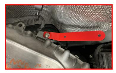
Install the harness that was attached to the top of the transmission crossmember onto the harness relocation bracket.
