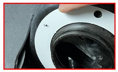
Center punch the marks and using an appropriate tool, drill the 1/2" holes through the spring tower.
