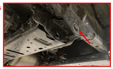
Install provided radius arm to the axle using the factory lower cam bolt.
