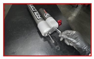
Install the bottom stem bushing, this will ensure the anti-rotation bracket stays in place.
