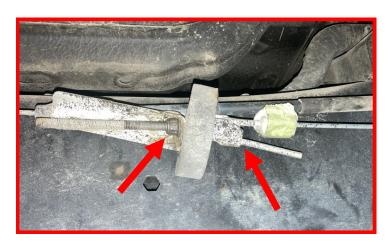
Remove the e-brake cable setup from the back of the rear driver side hub. You will need to unhook the cable hook attachment and also undo the clip that retains the cable housing itself.
