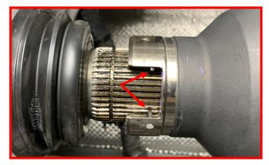
Mark the rear driveshaft to pinion flange location. Remove the rear driveshaft hardware from the flange. Let hang out of the way.
