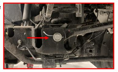
Remove the rear track bar from factory bracket.
