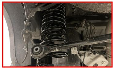
When installing the provided springs orient the flat end of the coil parallel with the sides of the vehicle.
