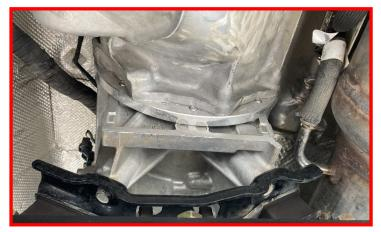
With the transfer case installed and mated back to the transmission, install the (8) provided nuts and washers.
