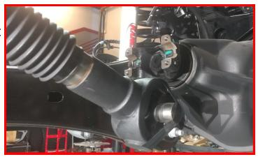
Remove the transfer case skid plate.
