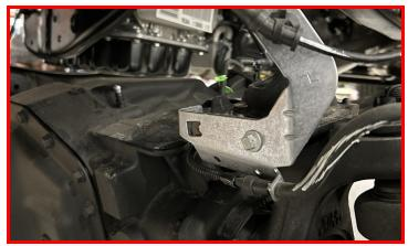
Remove the vacuum line clips from the driver side radius arm.
