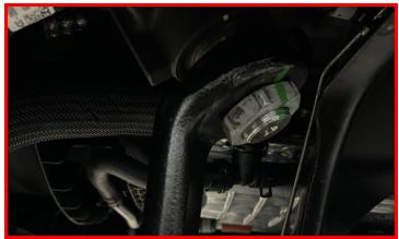
Remove the shock bolt and nut from the axle.
