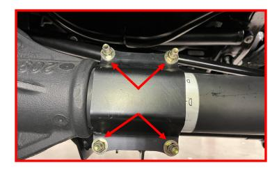
Remove tie rod retaining clips from vehicle and discard.
