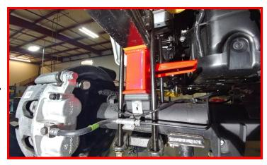
Install Falcon rear shock using factory hardware. Do not tighten at this time.
