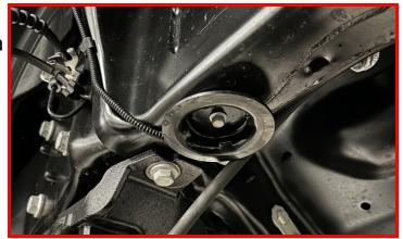
Remove the bump stop mount from the frame.
