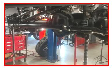
Remove the factory radius arm pivot hardware.
