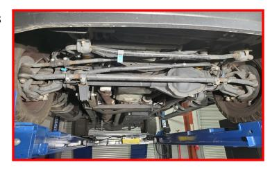
Remove the (2) middle bolts on the passenger side of the differential cover and retain the factory hardware. Remove the differential ID tag and either place in a secure location (skip next step), or reinstall on the driver side of the differential (see next step).
