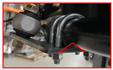
Install the passenger tie rod bracket using the supplied 3/8" U-bolts, 3/8" flat washers, and 3/8" toplock nuts. Place the plate flush against the flat face on the bottom of the tie rod. Do not fully tighten at this time.
