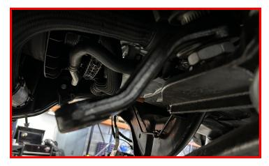
Clean off any debris off the sector shaft. Coat the sector shaft splines with a light duty liquid based lubricant or oil.
