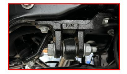
Remove the steering stabilizer from the frame.
