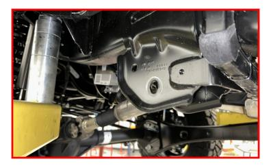
Install the replacement radius arm to axle using factory hardware for the upper connection and using the supplied cam bolts for the lower connection.
