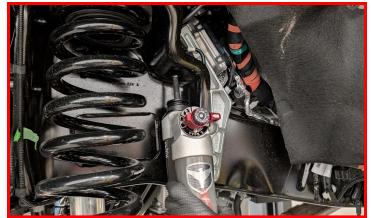
Using the factory hardware on the bottom, install into the lower shock perch.
