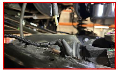
Install the supplied barbed coupler and vacuum line in between the factory line and the elbow.
