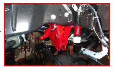
Install the track bar into the ReadyLIFT track bar mount using the factory hardware and the ReadyLIFT offset square washers. Make sure the offset is closest to the driver side, as shown.
