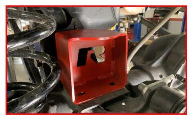
On the driver side only, Install the bump stop nut plate.
