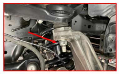
Loosen the upper control arm bolts located inside strut tower.
