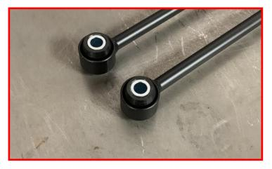
Use a fair amount of grease on the inside of the bushing and press the M10 crush sleeve into the bushing.
