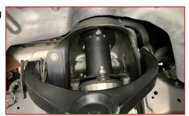
Swing the lower control arm up and install the factory lower strut bolt through the lower control arm.
