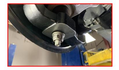
Install the upper ball joint into the knuckle using the factory ball joint hardware.
