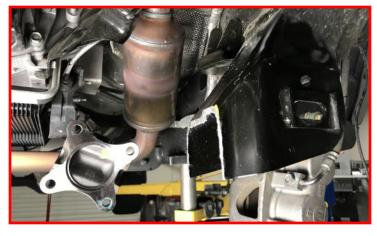
Install the driver side differential drops onto factory differential mounting point using the factory bolts. Do not tighten at this time.
