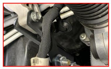
Note: Due the fact that there are minor differences in frame production, it may be necessary to trim the bottom edge of the front control arm pivot pocket.
