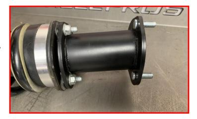
Mark the factory brake line bracket on the upper strut mount as shown.
