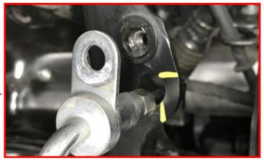
Remove brake line from factory mounting area.
