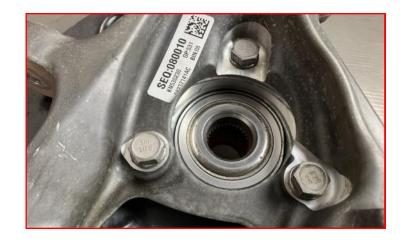
Remove hub assembly from factory knuckle.
