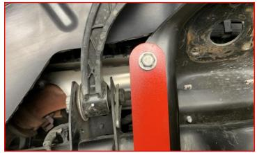
Install the completed strut assembly using the supplied M10 serrated flange nut.
