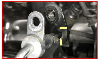
Remove brake line from factory mounting area.
