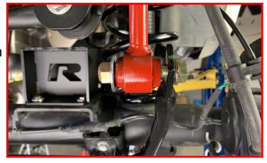
Note: Ensure the fender washer is installed on the bushing side.
