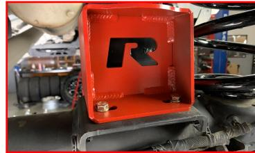
Install the driver rear brake line bracket onto the spring tower using the supplied M6 x 25mm bolt, nut and washers. Do not tighten at this time.
