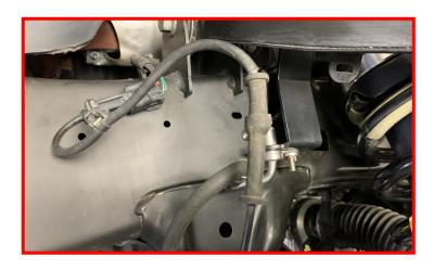
Connect the ride height sensor link to the upper control arm.
