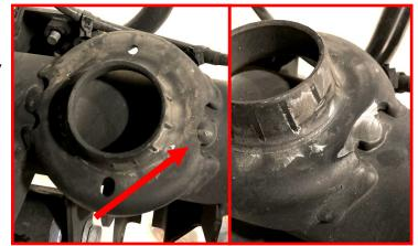
Install the air bag spacer using the 1/4-20 x 1" bolts, washers, and lock nuts. Orient the oval mounting hole toward the front of the vehicle.
