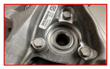
Remove hub assembly from factory knuckle.
