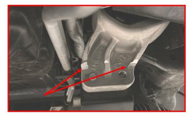
Before tightening the passenger side rear differential drop, ensure the large notch is orientated up and against the factory differential mounting point.
