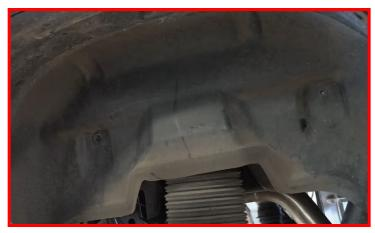
Install the tires and slowly lower the truck. Ensure that the air bag seats on the spacer properly as the truck is lowered.
