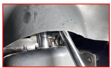
Remove the outer tie rod end nut.
