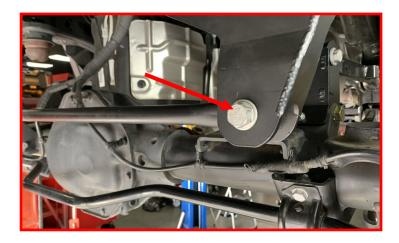
If necessary, gently compress the air bag to make room for the air bag spacer.
