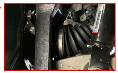
Install the factory ball joint hardware.
