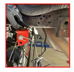
While gently pulling down on the brake line install the factory brake line bracket onto the rear track bar bracket using the factory hardware and supplied M8 nut and washer.
