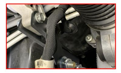
NOTE: Due to minor differences in frame production, it may be necessary to trim the bottom edge of the front control arm pivot pocket.
