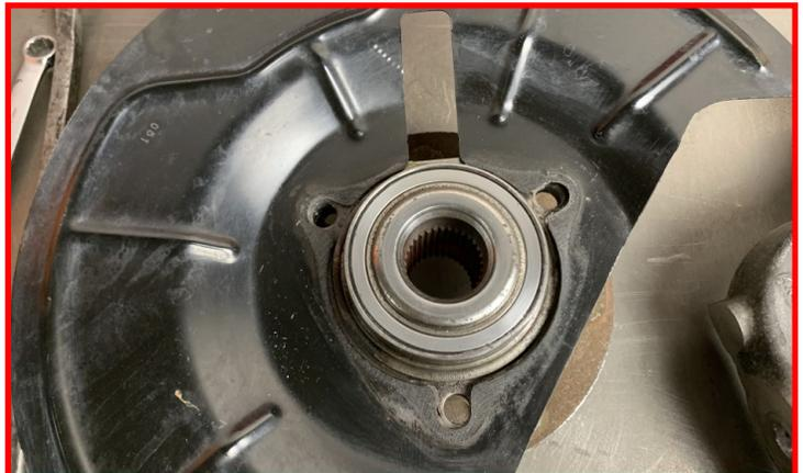
Install rotor dust shield and hub assembly into replacement knuckle using the (3) factory hub bolts and thread locker.
