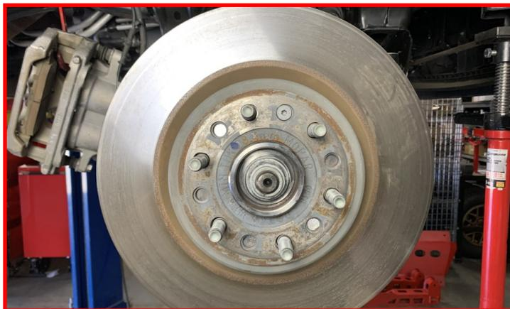
Install the brake caliper to the knuckle using the factory hardware and a drop of thread locker.
