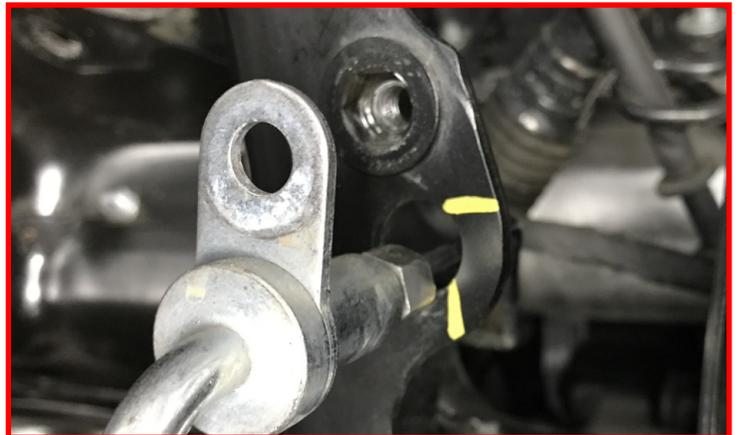
Remove brake line from factory mounting area.
