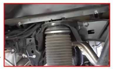
Remove the upper sway bar end link at the frame rail.
