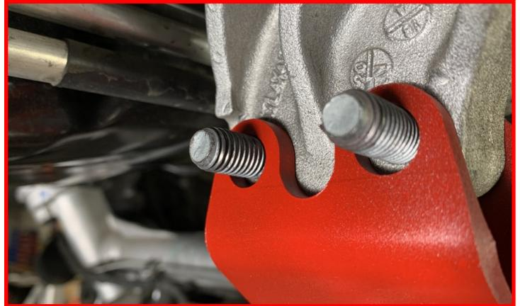
Install the rear differential drop onto the rear factory differential mounting point using the supplied M12 x 35mm bolts, nuts and washers.
