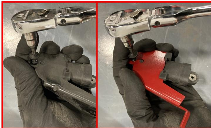
Install the ride height sensor and relocation bracket using the factory bolt torqued to **8 ft-lbs**.
