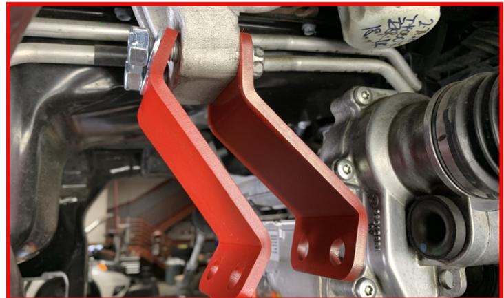
**NOTE:** Due to minor differences between trucks, it may be necessary to grind the webbing on the mount to clear the new drop bracket.
