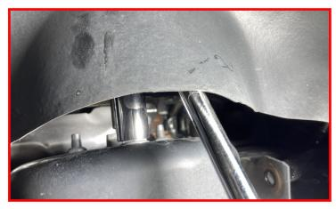
Remove the outer tie rod end nut.
