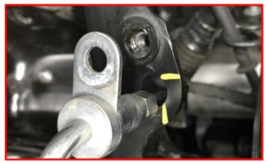
Remove brake line from factory mounting area.
