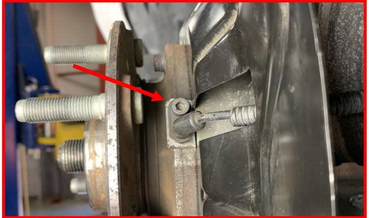
Remove rubber isolator from the ABS bracket on the inside of the knuckle.
