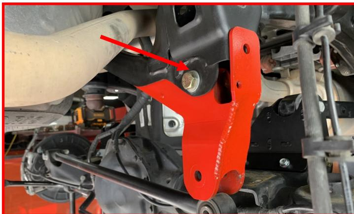
With the track bar bracket in place install the supplied M12 x 35mm bolt, nut and washers through the track bar bracket and the factory track bar mount brace. Do not tighten at this time.
