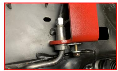
Using the factory brake line mounting hardware, install the brake line drop bracket onto the factory brake line mounting location.
