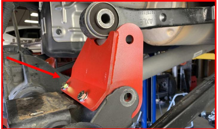
Install the upper control arm crush sleeve between the upper control arm bracket and the control arm axle mount.
