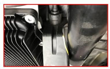
Mark the factory brake line bracket on the upper strut mount as shown.
