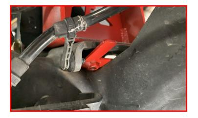
Install the supplied M8 bolts, nuts and washers through the bump stop extension and axle pad.
