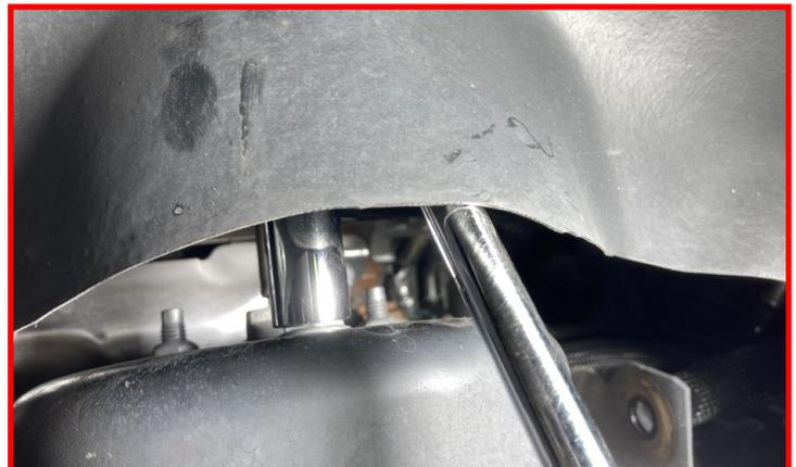
Remove the outer tie rod end nut.
