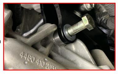
Install the (3) factory mounting bolts through the rear differential drop bracket and into the differential.
