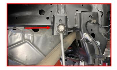
Remove the lower sway bar end link at the sway bar.
