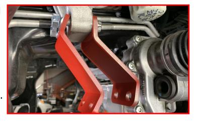
NOTE: Due to minor differences between trucks, it may be necessary to grind the webbing on the mount to clear the new drop bracket.
