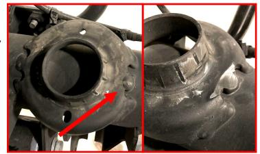
Install the air bag spacer using the 1/4-20 x 1" bolts, washers, and lock nuts. Orient the oval mounting hole toward the front of the vehicle.
