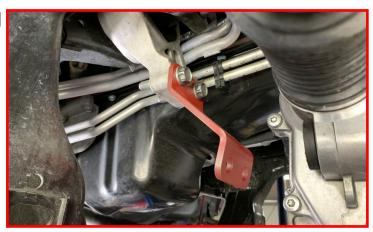
Before tightening the passenger side front differential drop, ensure the small notch is orientated up and against the factory differential mounting point.
