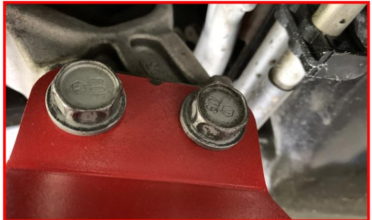
Install the passenger side rear differential drop onto the rear factory differential mounting point using the using the supplied M12 locking nuts and M12 washers.
