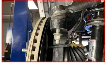
Install sway bar drop brackets using the factory hardware.
