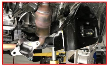
\*\*\*Parts shown in red for picture clarification only\*\*\* Install the driver side differential drops
