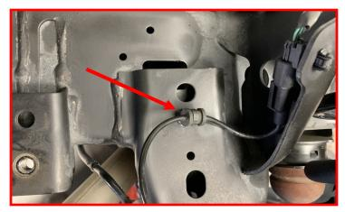
Locate and remove the driver brake line bracket mounted on the frame rail.
