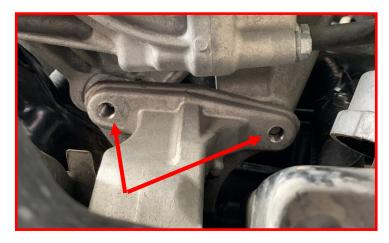
Remove (2) passenger side differential mounting bolts. Retain the factory hardware.
