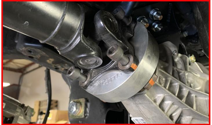
**NOTE:** Due to variation in vehicle models, you may need to trim the plastic bracket on the side of the transmission due to contact with the driveshaft.
