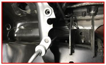
Using care, carefully pull down on the brake line. While pulling the brake line down into place you'll need to rotate the bulkhead fitting so the hardline is aimed toward the rear on the vehicle.
