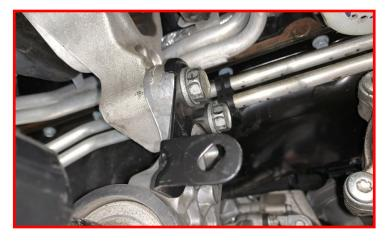
Remove the (3) driver side rear differential mounting hardware. Retain the factory hardware.
