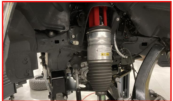
Swing the lower control arm up and install the factory lower strut bolt through the lower control arm.
