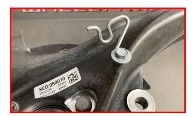
Locate the factory knuckle and hub assembly. Remove the (3) hub assembly mounting bolts.
