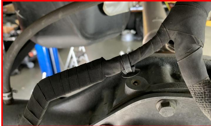
Remove the harness retaining clip from the stud on the rear differential cover.
