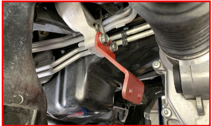
Before tightening the passenger side front differential drop, ensure the small notch is orientated up and against the factory differential mounting point.
