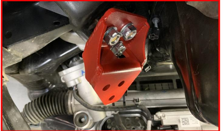
Raise differential into place. Be sure to use a helper to aid in the installation process. With the differential in place, install the provided M12 x 60mm bolt, washers and nut through the driver side inner differential drop bracket, the diff drop spacer, the differential housing, then the driver side outer differential drop bracket.
