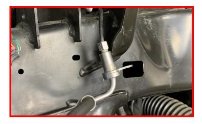
Install the brake line drop bracket onto the factory brake line bulkhead fitting using the supplied M6 bolt, locking nut and washers.
