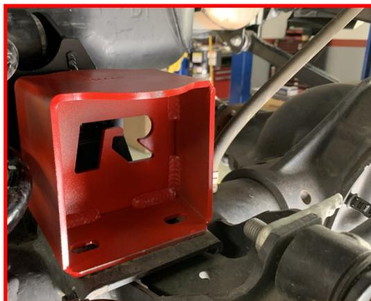
On the driver side only, Install the bump stop nut plate.
