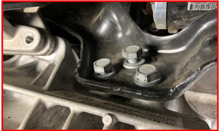
Ensure all the differential mounting hardware is removed, slowly lower the differential and remove from vehicle.
