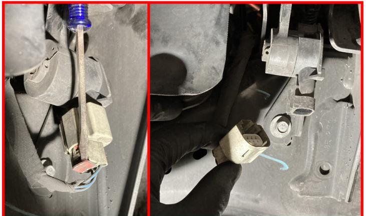
Remove the ride height sensor link from the control arm using a small pry bar or similar tool.
