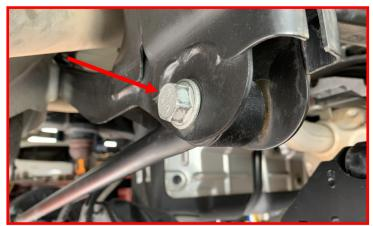
Install track bar bracket using the 14mm x 70mm bolt, washers, and c-lock nut in the track bars original location. Do not tighten at this time.
