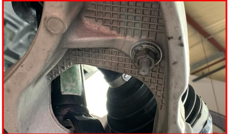
Remove (4) sway bar mounting bolts from the frame and retain the factory hardware. Remove sway bar from the vehicle.
