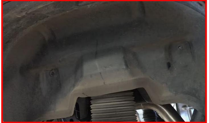
Install the tires and slowly lower the truck. Ensure that the air bag seats on the spacer properly as the truck is lowered.
