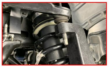
Install the opposite side ABS wire bracket on the inside of the knuckle using the factory hardware (i.e. Driver will be installed on passenger side).
