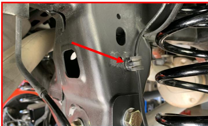
Install the sway bar end link assembly onto the frame using the supplied M10 x 70mm bolt and M10 fender washer. Do not tighten at this time.
