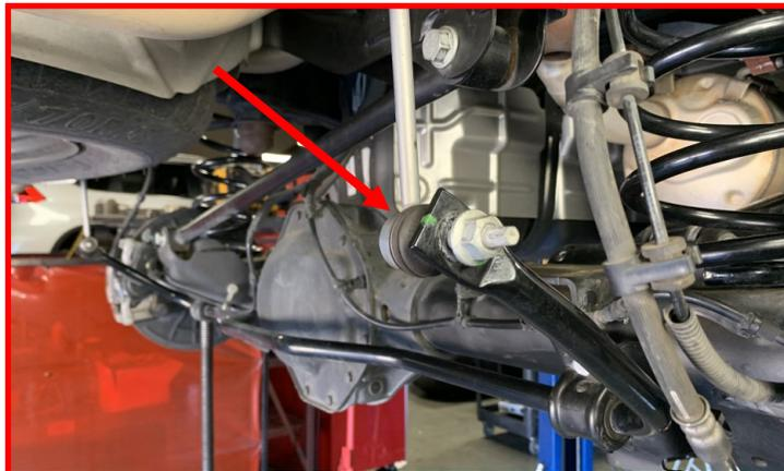
Locate and remove the passenger brake line bracket mounted on the frame rail.
