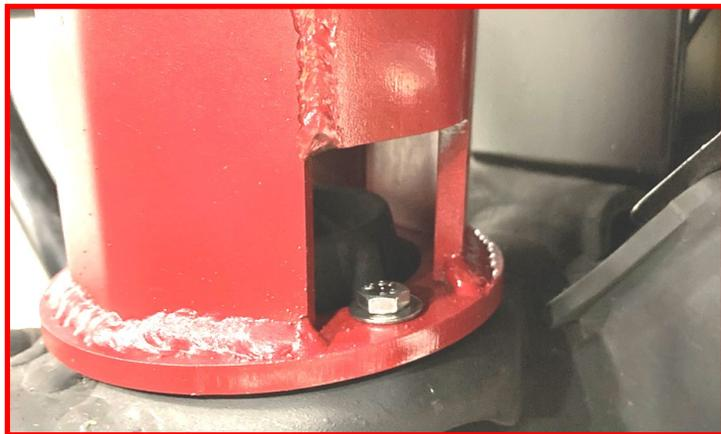
Using the factory mounting hardware, install the aftermarket shock per the manufacturer's suggested installation instructions.
