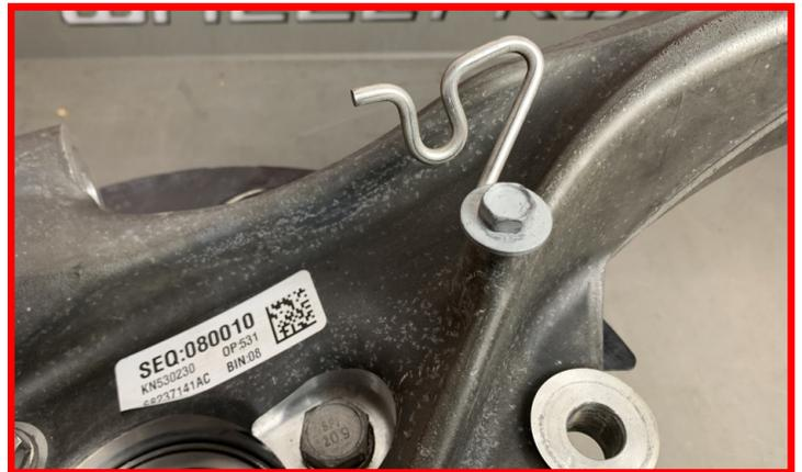
Locate the factory knuckle and hub assembly. Remove the (3) hub assembly mounting bolts.
