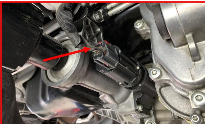
Remove the harness retaining clip from the retaining bracket attached to the differential mount.
