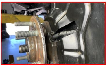
Install the ABS wire mounting grommet into the ABS wire bracket .
