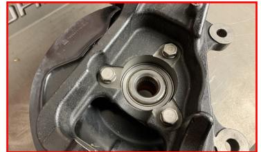
Install the completed knuckle assembly to the lower ball joint while guiding the CV axle through the hub.
