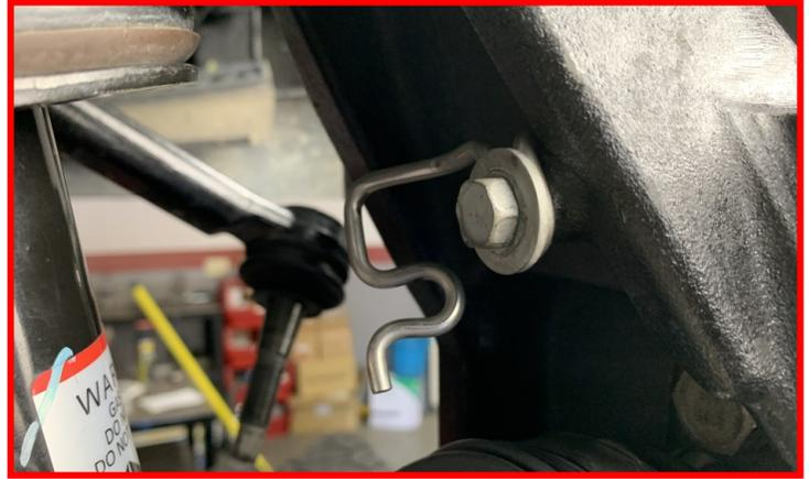
Remove the ABS wire harness retaining clips that are attached to the frame rail. This will allow additional length that is required to install the ABS sensor into the knuckle.
