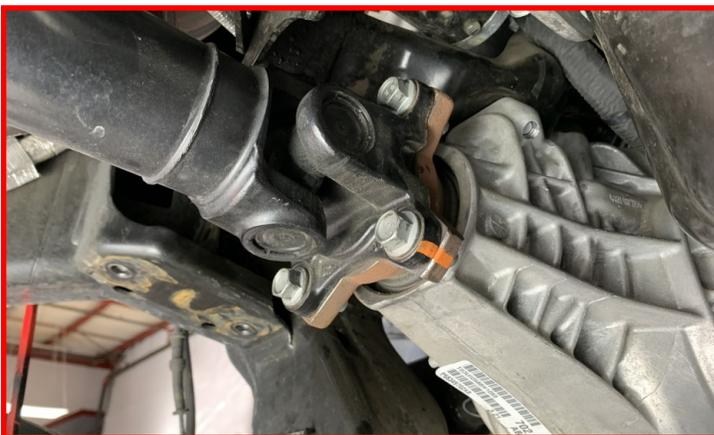
Unplug the differential shift actuator. Ensure all clips are removed and clear of the differential.
