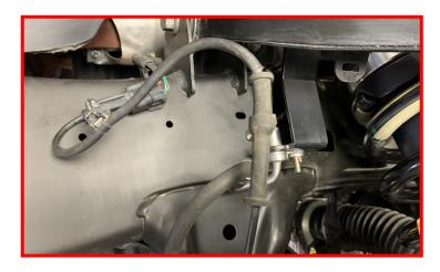
Connect the ride height sensor link to the upper control arm.
