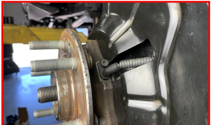
Install the ABS wire mounting grommet into the ABS wire bracket .
