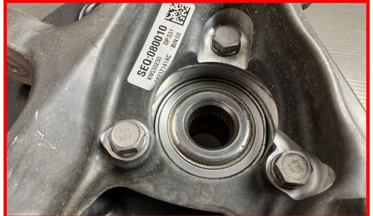
Remove hub assembly from factory knuckle.
