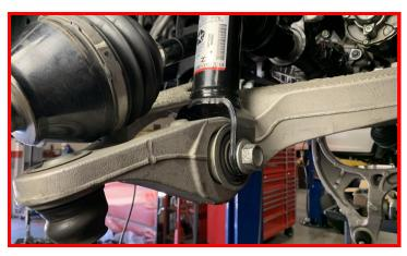
With the strut installed, use the supplied cable ties to secure the air line to the steel portion of the brake line.
