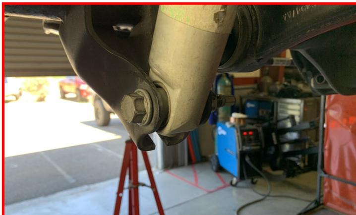
Remove the shock top mounting hardware. Remove shock from the vehicle and dispose of the shock in an appropriate manor.
