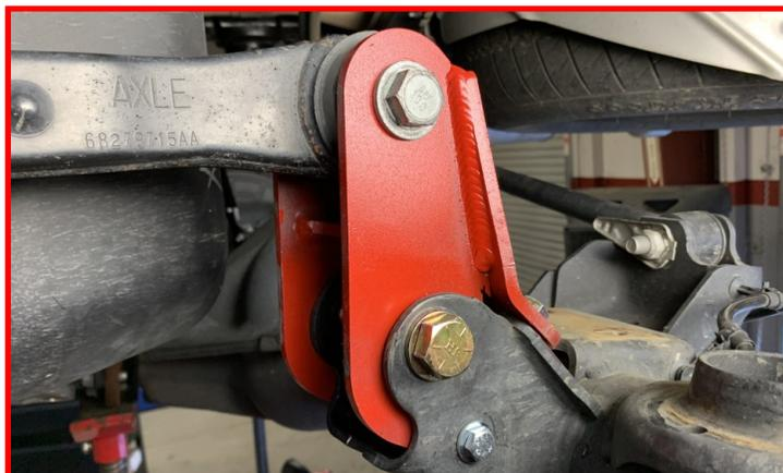
Remove the frame side track bar mounting bolt.
