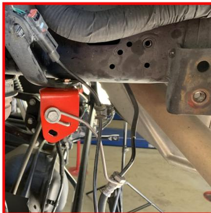
Install the ABS retaining clip into the driver rear brake line bracket in the bottom hole. Tighten the bracket at this time.
