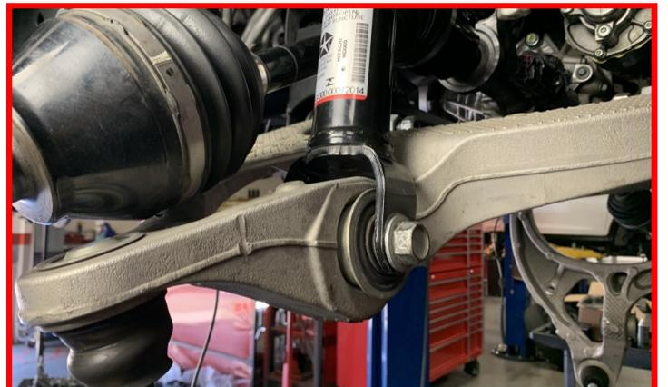
With the strut installed, use the supplied cable ties to secure the air line to the steel portion of the brake line.
