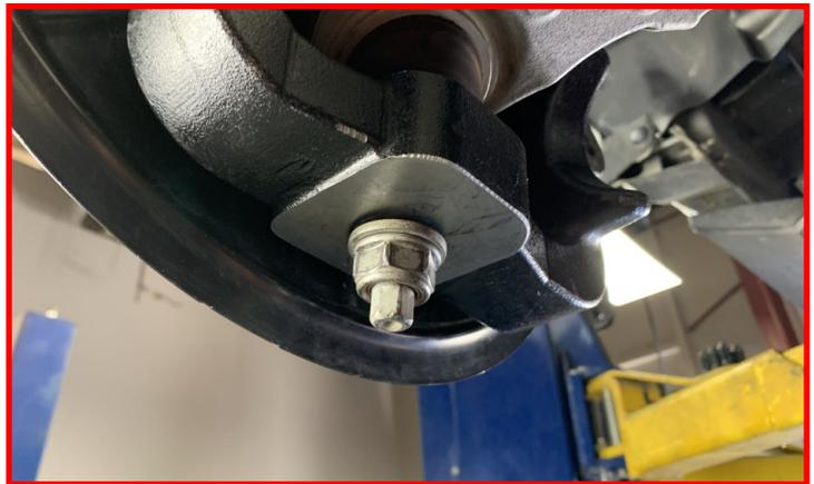
Install the upper ball joint into the knuckle using the factory ball joint hardware.
