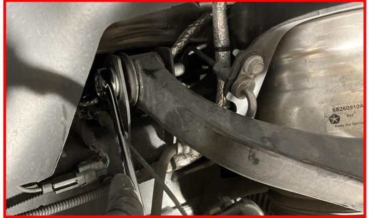
Loosen but do not remove the lower control arm ball joint nut. Strike the lower ball joint boss on knuckle with a dead blow hammer to dislodge the taper. Remove nut and then the knuckle from the vehicle.
