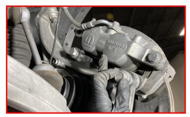
Remove brake rotor retaining bolt and remove the rotor. Retain the factory hardware.
