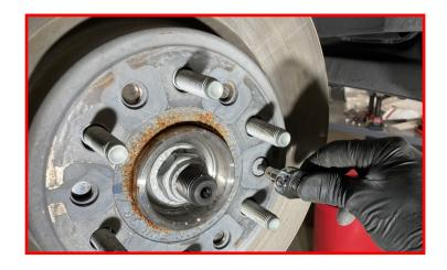
Remove the wheel speed sensor from the knuckle and hang out of the way. Retain the factory hardware.
