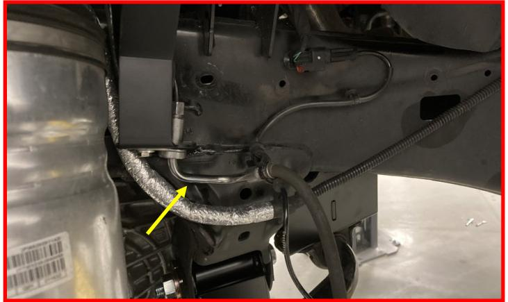
Remove the **ABS wire bracket** on the inside of the knuckle. Pay close attention to the orientation of the wire bracket.
