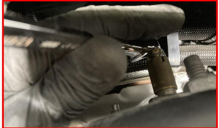
Loosen the three top air strut nuts but do not remove at this time.
