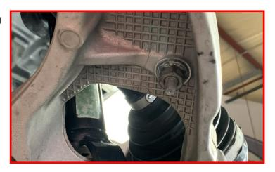
Remove (4) sway bar mounting bolts from the frame and retain the factory hardware. Remove sway bar from the vehicle.
