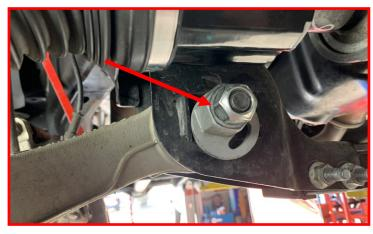
Remove the lower air strut mounting bolt from the lower control arm. Retain the factory bolt.
