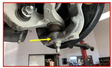
Remove the lower sway bar end link from the lower control arm. Retain factory hardware.
