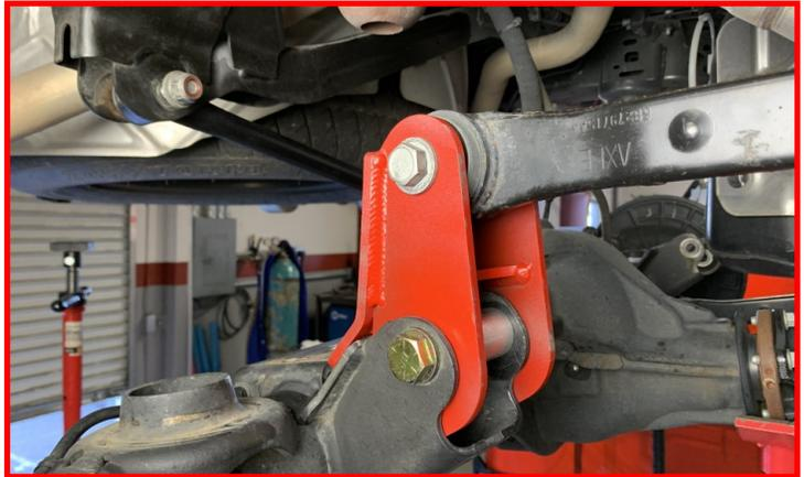
Torque the M10 axle bolts to **55 ft-lbs.**
