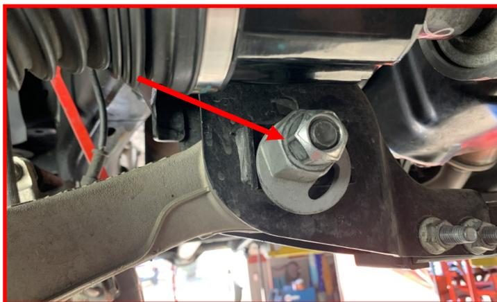
Remove the lower air strut mounting bolt from the lower control arm. Retain the factory bolt.
