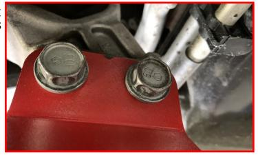
Install the passenger side rear differential drop onto the rear factory differential mounting point using the using the supplied M12 locking nuts and M12 washers.
