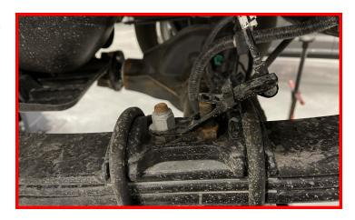
Slightly loosen but do not remove the Passenger side u-bolts.
