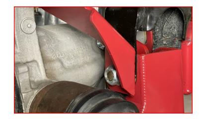
Install the passenger differential support bracket on the passenger side differential drop bracket using M14 washer and lock nut on the M14 x 100mm bolt already installed, as well as the supplied M14 x 35mm bolt, washer and lock nut.
