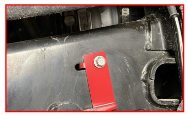
Install the brake line into the new brake line bracket using the clip previously removed.
