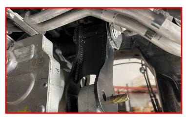
Install the sway bar brackets to frame using the factory hardware.
