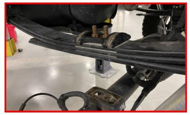
Install the provided lift block making sure the bump tang is facing inboard of the vehicle. Raise the axle and the block up to the spring while aligning the center pins.
