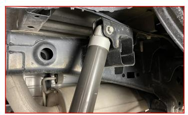
Install the rear shock into the factory axle mounting location using the factory hardware.
