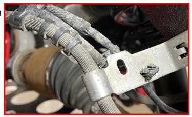
Install vacuum line onto brake line bracket.
