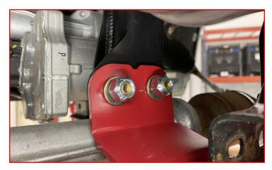
The other end of the passenger diff support bracket will install onto the rear crossmember using the provided M12 x 35mm bolt, washer and lock nut.
