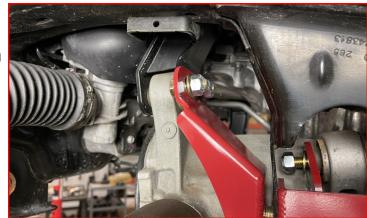
The other end of the driver diff support bracket will install over the rear crossmember M18 bolt. Install the provided M18 washer and lock nut at this time.
