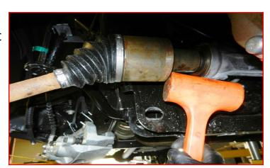
Remove the mounting bolts and oil drip tray that is located on the driver side over the steering rack.
