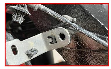
Install the ABS wire to factory locations on factory brake line brackets. Run the ABS line on the outside of the strut tower next to the vacuum lines at strut tower location. install electrical connectors in engine compartment.
