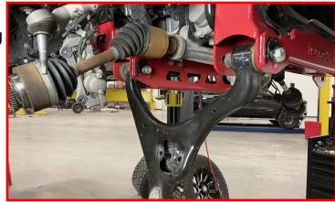
With the differential tight and crossmember torqued to spec, install the skid plate using the M10 x 30mm bolts, washers and thread locker.
