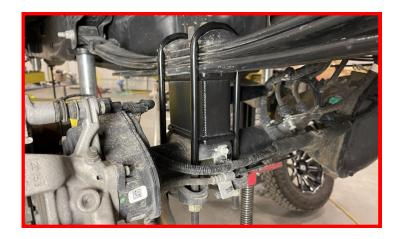
Install the rear sensor bracket on the forward axle center pin in the factory orientation.
