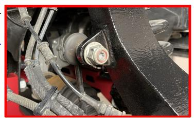
Install the tie rod end into the knuckle using the factory hardware.
