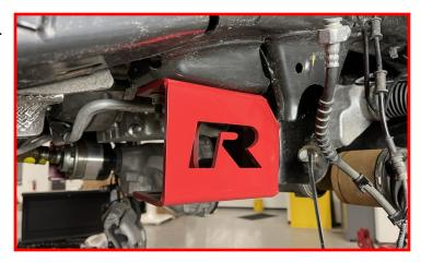
Install the rear cross member into the factory control arm frame pockets using M18 x 150mm bolts, flat washers, and lock nuts.
