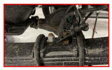
Install the rear brake line drop bracket to the frame using factory hardware.
