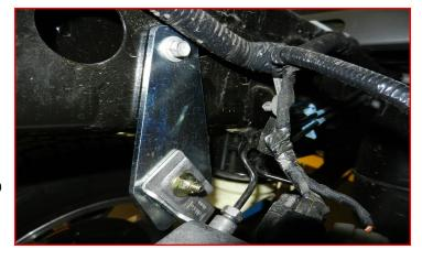
Install the provided rear shock into the factory frame mounting location using the factory hardware.
