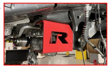
Install the rear cross member into the factory control arm frame pockets using M18 x 150mm bolts, flat washers, and lock nuts.
