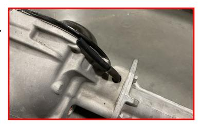
Raise differential into place. Be sure to use a helper to aid in the installation process. With the differential in place, install the factory bolt and nut through the factory driver side differential mount and the driver diff drop bracket.
