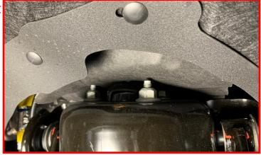
Remove the lower strut nuts.
