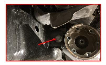
Remove the passenger side diff mounting bolt.
