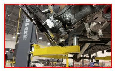
Install upper ball joint to knuckle using factory hardware.
