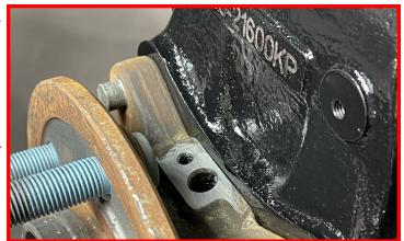
Install dust shield to knuckle using factory hardware.
