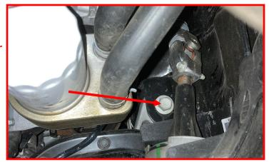
Remove the rear diff mounting bolt.
