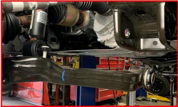
Remove the factory rear crossmember (4) mounting bolts and nuts and carefully remove the crossmember from the vehicle.
