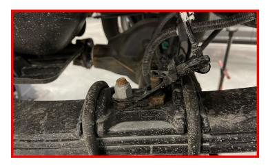
Slightly loosen but do not remove the Passenger side u-bolts.
