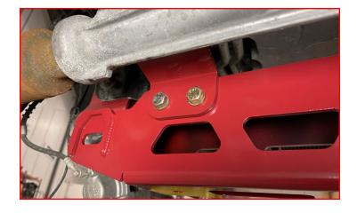
Install the front cross member using the factory hardware from the front of the vehicle facing rearward.
