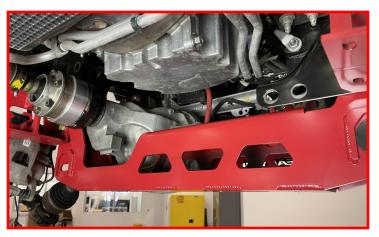
Install the rear diff mount into the rear crossmember using the supplied M14 x 100mm bolt, washers and lock nut.
