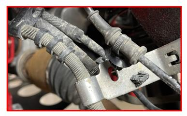
Install the sway bar onto the sway bar drop brackets using the supplied M10 x 30mm bolts, washers and lock nuts.
