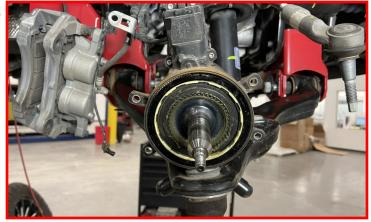
Install the knuckle onto the lower ball joints using factory ball joint nut. Run the nut tight at this time.
