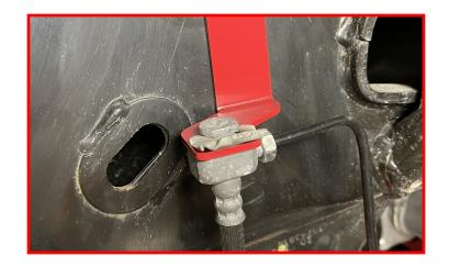
Install the factory brake line bracket to knuckle using the supplied M8 x 16mm bolt, and washer
