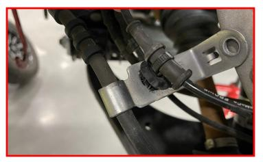
Remove the **EIWE** vacuum line from the brake line bracket.
