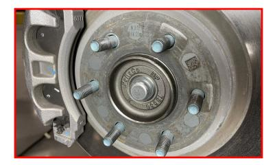
Remove the brake caliper mounting bolts from brake caliper.
