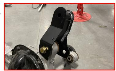
Install the passenger side differential drops onto passenger differential mounting point using the supplied M14 x 100mm bolt and washer. Do not install the backside M14 washer and nut at this time.
