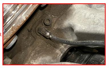
Remove the CV shaft retainer nut.
