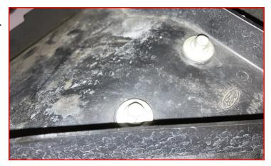
Using an appropriate jack, support the deferential.
