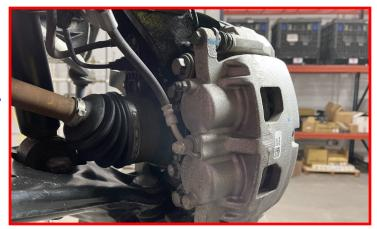
Fasten the CV shaft to the hub with the factory nut.
