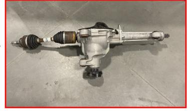
Measure from the outside edge of the driver side rear control arm pocket 2 5/8".
