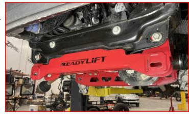
Install driver and passenger side lower control arms into the cross members using the supplied M18 x 150mm cam bolt, eccentric plates and lock nut.
