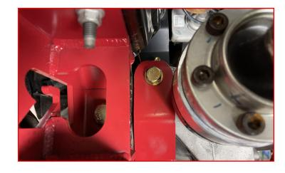
Install the driver differential support bracket on the driver side differential drop bracket using M14 washer and lock nut on the M14 x 100mm bolt already installed, as well as the supplied M14 x 35mm bolt, washer and lock nut.
