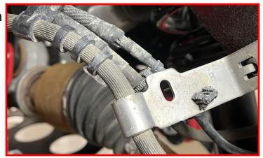
Install vacuum line onto brake line bracket.
