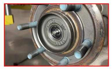
Remove the (4) bolts that attach the EI-WE to the knuckle and pull both axle and the EIWE out of the factory knuckle.
