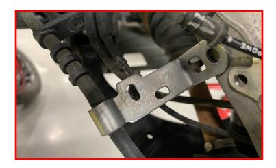
While supporting the sway bar, remove the frame side mounting nuts.
