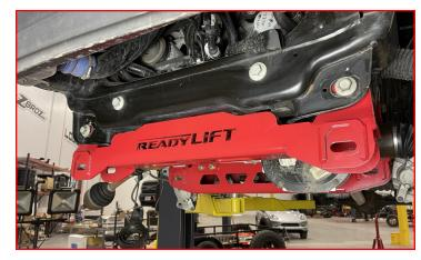
Install driver and passenger side lower control arms into the cross members using the supplied M18 x 150mm cam bolt, eccentric plates and lock nut. NOTE: Do not fully tighten these bolts until the weight of the vehicle is resting upon the suspension.
