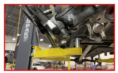
Install upper ball joint to knuckle using factory hardware.
