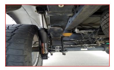
Prior to installing wheels, complete all installation steps on the opposite side. Install the wheels and lower the vehicle to the ground. Install rear wheels and lower vehicle to the ground. Torque lug nuts to wheel manufacturers specifications. Jounce vehicle to settle suspension. Torque rear u-bolts to 110 ft-lbs, and shock hardware to 60 ft-lbs. Install the vehicles power source at the ground terminal.
