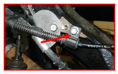
Attach the IWE Vacuum lines to the IWE.
