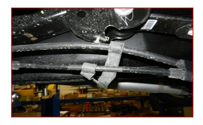
Remove the brake line bracket from the frame. Support rear axle with a suitable jack and remove the shocks.
