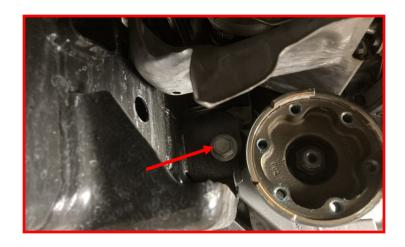
Remove the passenger side diff mounting bolt.
