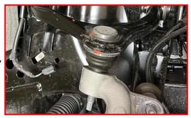
Remove the (3) bolts that attach the EIWE to the knuckle and pull both axle and the EIWE out of the factory knuckle.
