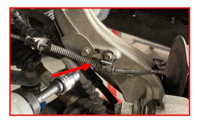
Remove the IWE vacuum lines from the IWE on the backside of the knuckle.
