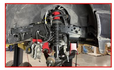
Install the passengers side CV shaft (If removed).
