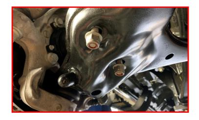
Remove the factory front brake line bracket from the frame.
