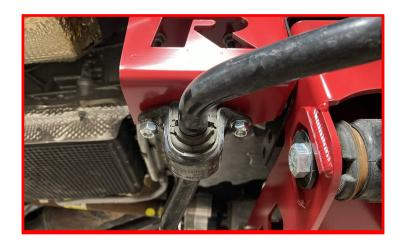
Install the sway bar end links to the control arm with the factory hardware.
