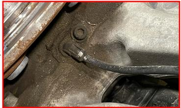
Remove the CV shaft retainer nut dust cover.
