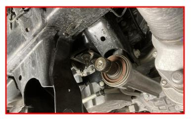
Install the IWE onto the CV shaft. Ensure the gears are lined up and engaged properly.
