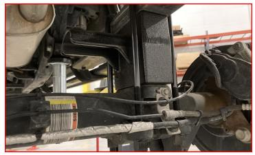
Install the rear brake line drop bracket to the frame using factory hardware. Gently pull the rear hard lines down and attach the rear brake line bracket to the drop bracket using M8 x 25mm bolt, washers, and lock nut. Torque all to 10 ft-lbs.
