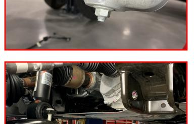
Remove the factory rear crossmember (4) mounting bolts and nuts and carefully remove the crossmember from the vehicle.
