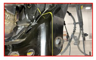
Install the driver side differential drops onto driver differential mounting point using the supplied M14 x 100mm bolt and washer. Do not install the back side M14 washer and nut at this time.
