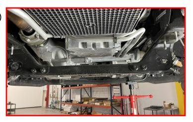
Mark the driveshaft to pinion flange location. Remove the (6) drive shaft mounting bolts and disconnect the drive shaft from the differential. Allow the drive shaft to rest out of the way.
