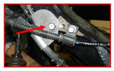
Attach the ABS bracket to the knuckle. Torque to 5 ft-lbs.
