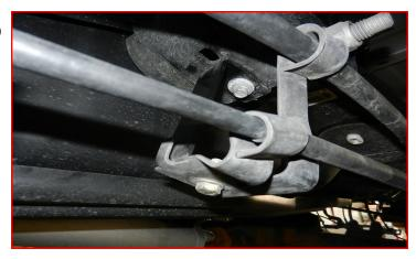
Install new rear shocks with factory hardware. Do not tighten at this time.
