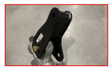
Attach the differential breather tube extension to the differential breather elbow.
