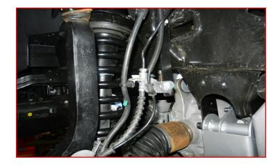
Install the factory brake line bracket to knuckle using the factory hardware.
