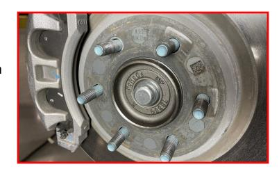
Remove the CV shaft retainer nut.
