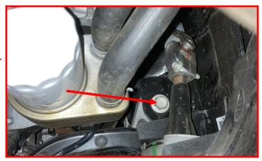
Remove the rear diff mounting bolt.
