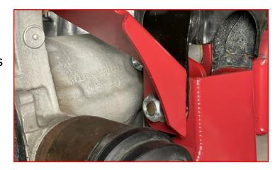
Install the passenger differential support bracket on the passenger side differential drop bracket using M14 washer and lock nut on the M14 x 100mm bolt already installed, as well as the supplied M14 x 35mm bolt, washer and lock nut.
