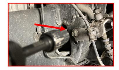
Remove the brake line bracket from the knuckle.
