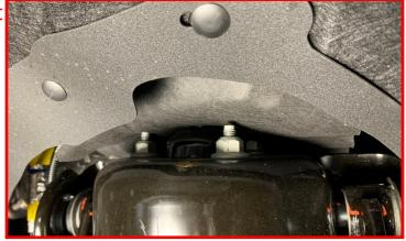
Remove the lower strut nuts.
