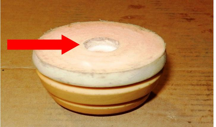
Use a soap and water solution to aid in installation, push the bump stops into the ReadyLIFT extensions with a twisting motion. Make sure they fully seat.
