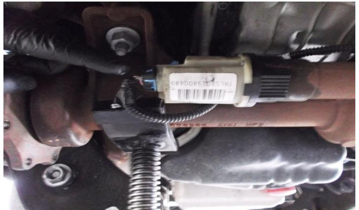
Mark the front drive shaft to pinion orientation for reinstallation later. Remove the front drive shaft from the differential. Let hang out of the way.
