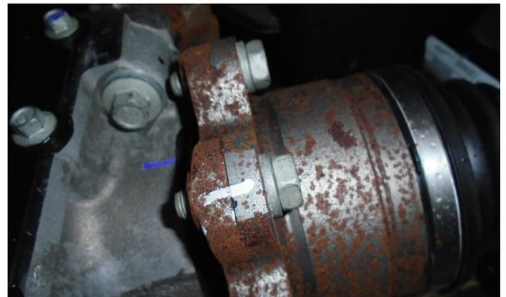
Remove the LCA and torsion bars from the frame. Make sure to keep the torsion bars in the same direction as they were installed from the factory.
