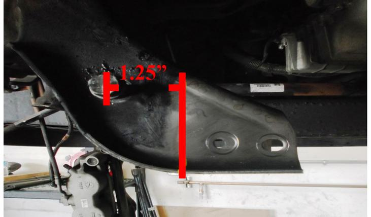
Using a suitable cutting tool, cut along the previous made marks. Remove and discard the outer portion of the control arm pocket. Paint the exposed metal with a quality rust preventative paint.
