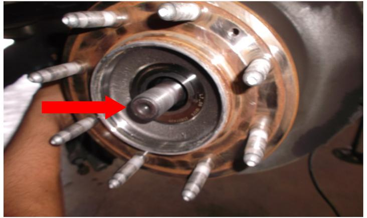
Remove the hub bearing mounting hardware from the knuckle. Make sure to not drop the hub assembly. Remove the dust shield with the assembly.
