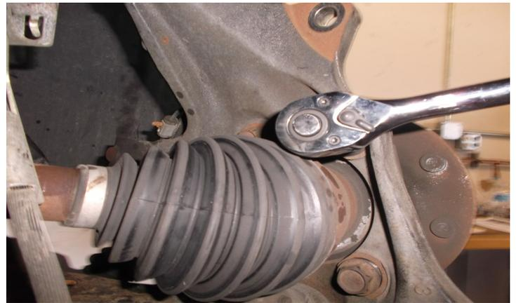
Support the LCA with a suitable jack. Loosen but do not remove the upper and lower ball joint nuts. Strike the ball joint boss on the knuckle to dislodge the tapers. Remove the knuckle from the upper and lower control arms.
