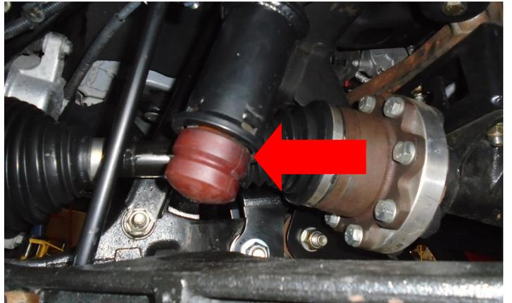
Reinstall The CV axle factory nut.
