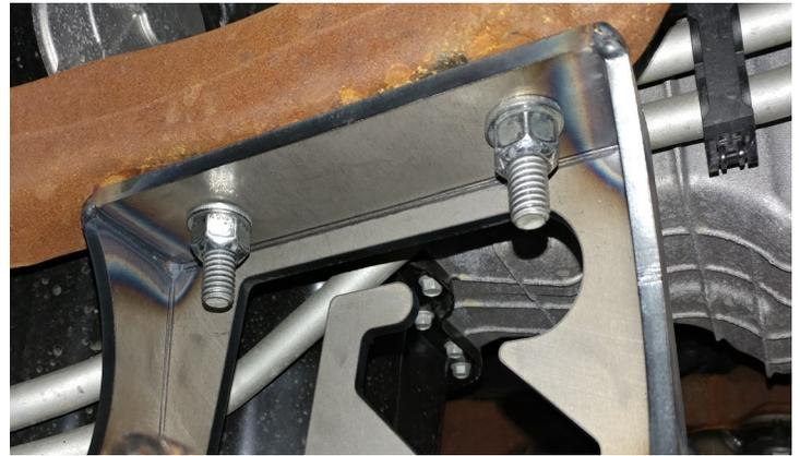
Install the ReadyLIFT driver side diff drop to the diff cradle using provided **M12 bolts and washers** to the forward two locations. Install the last mount using the **factory bolt and a provided M12 washer and nut**. Do not tighten at this time.
