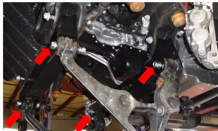
**Tighten and torque** the ReadyLIFT cross members to the frame. Torque to 150 FT-LBS. Do not tighten the LCA these have bonded bushings and must be tightened when the vehicle is at ride height.
