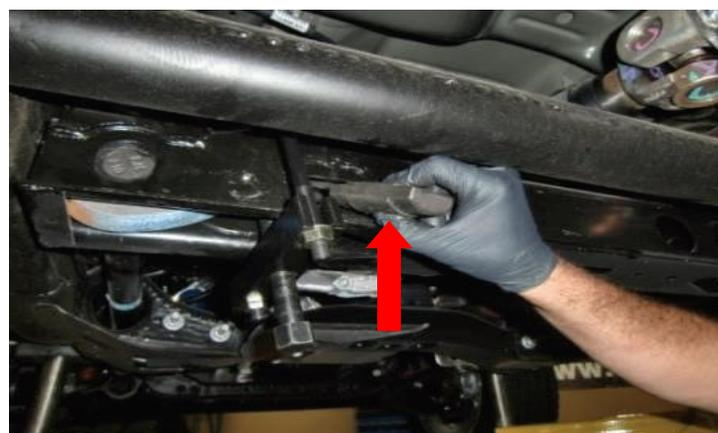
Push the torsion bar forward through the factory keyway cross member and lower control arm. You may need to use a hammer and punch. Hammer on the end of the bar to break it loose from the keyway and control arm. Remove the factory Key.
