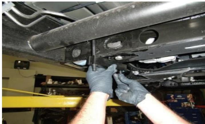
Once the torsion key is adjusted high enough, remove the cross pin. **DO NOT push it through with your finger.** Always pull it out away from the keyway. Once the cross pin is out, remove the torsion bar unloading tool.
