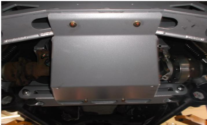
Use the torsion bar unloading tool, load the torsion bar enough to install the cross pin. **DO NOT pull it through with your fingers**.
