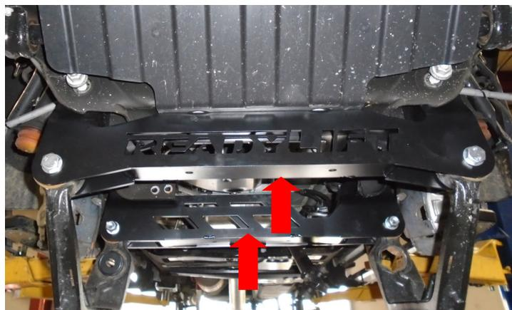
Install the lower control arms to the ReadyLIFT cross members using the provided **M18 bolts, washers, and nuts**. Do not tighten at this time.
