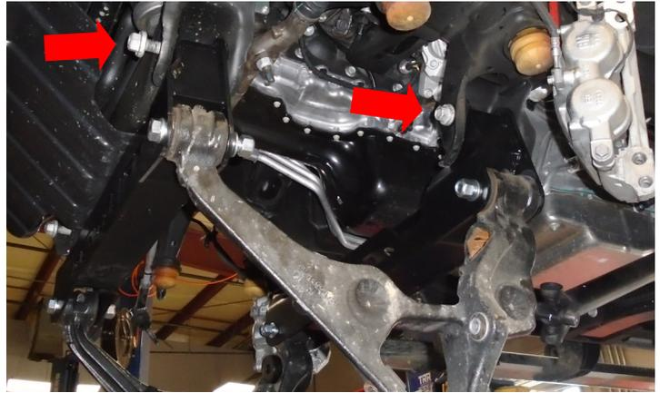
Install the provided torsion bar bracket spacer into the torsion bar pocket on the lower control arm. Install the spacer from the back side of the LCA and add the collar to the spacer from the front side of the LCA
