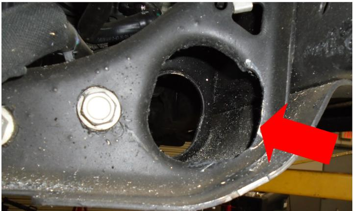
Install the torsion bar bracket with the pervious installed torsion arm spacer. The spacer bolt should be tight, but does not need to be torqued.
