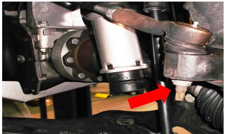
Install the extended brake line brackets. Use factory hardware to attach the bracket to the frame. Use provided hardware to attach the brake line to the bracket. Torque all brake line hardware to **20 ft-lbs**.
