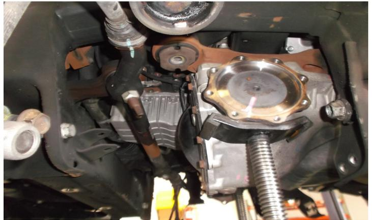
Clean the driver side rear control arm pocket. Measure from the center of the control arm mounting bolt hole to the inside of the frame pocket **1.25"**, mark a line vertically across the back and front side of the pocket. Connect the two lines across the top of the pocket.
