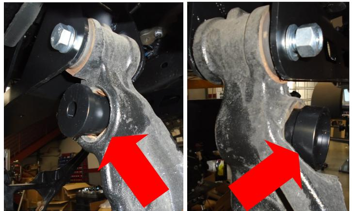
Mark the **front** side only of the transmission cross member where the torsion bars pass through. Mark at the 1 o'clock position and 5 o'clock position draw a 1/4" thick clearance line between these marks.
