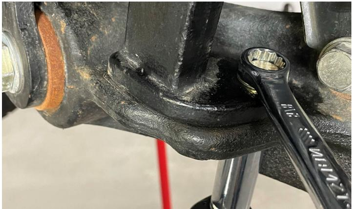
Reinstall the factory torsion bars and torsion keys. Make sure the torsion bars are installed in the same direction as they were installed from the factory. Leave the torsion keys loose. Do not add the cross pin or set screw at this time. Add the new torsion bar bracket to the torsion bars.
