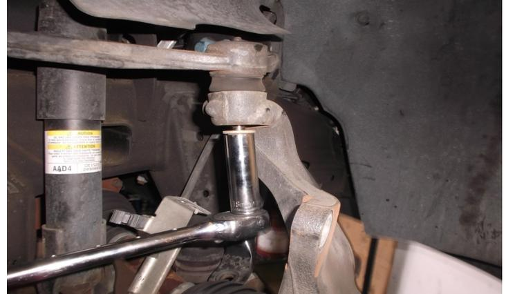
Mark the CV axle flange to the differential flange and driver / passenger side for reinstallation later. Remove the CV axle hardware. Remove the CV axle from the vehicle.
