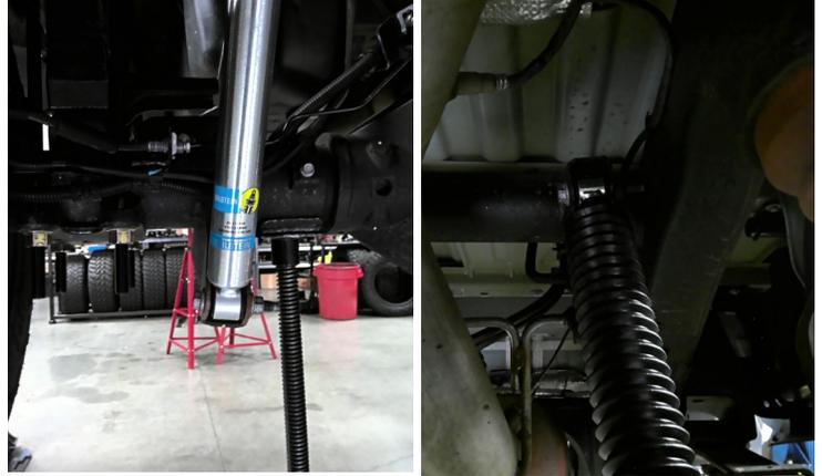
Install the provided **brake line bracket** to the differential. Use factory hardware. Attach the brake line to the extended bracket. Use provided hardware. Torque to **20 ft-lbs**.
