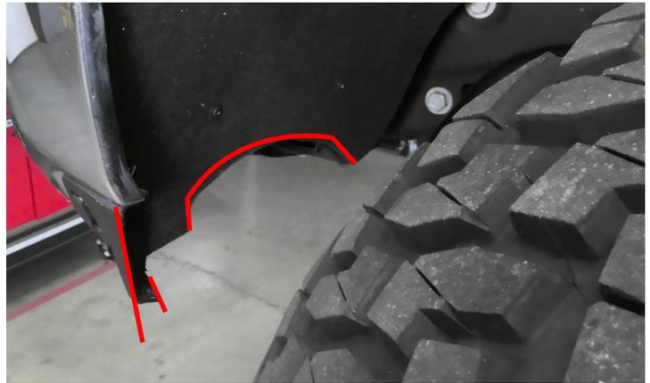
Remove the front wheel mud flap. mark a straight horizontal line 2" from the seamed edge. Use a suitable cutting tool, cut along the marked edge. Reinstall the mud flap.
