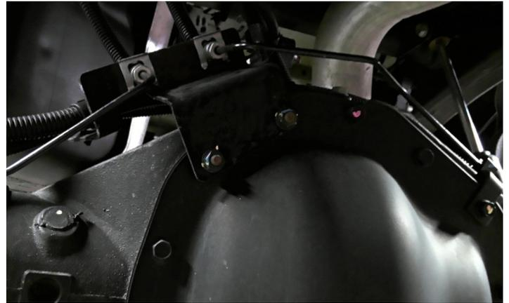
Remove the factory rear shocks. Retain hardware.
