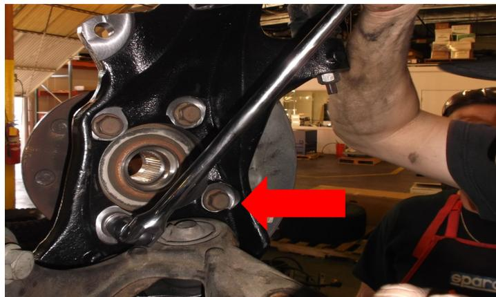
Reinstall The CV axle. Make sure to line up the previous marks on the flanges.
