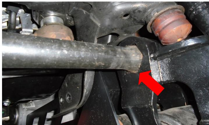
Raise the lower control arm and align the torsion bar bracket with the previous installed torsion arm spacer. Attach the bracket to the spacer. Use provided hardware. Torque the 3/4" hardware to 250 ft-lbs.
