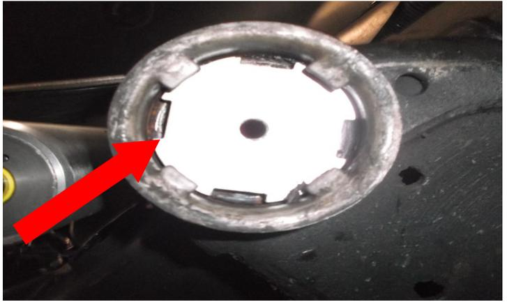
Place the ReadyLift Bump Stop Extension Washer between the bump stop and vehicle. Install the ReadyLIFT bump stop extension using provided **3/8" x 5.5" long Allen head bolt and washer.** Torque to **35 ft-lbs.**
