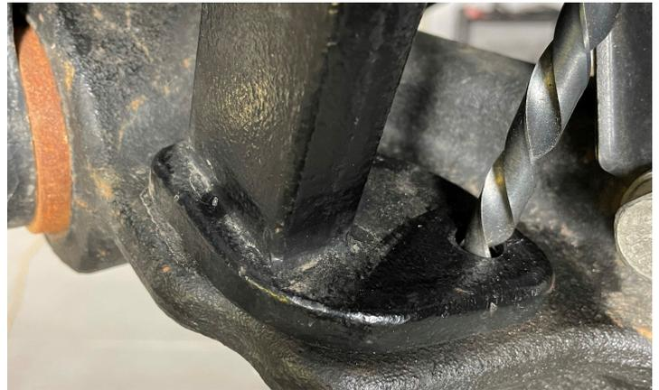
Remove the torsion bar bracket. Drill out to 7/16".
