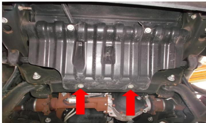
Remove the lower skid plate from the cross members. Reinstall the gravel guard bolts to the front cross member.
