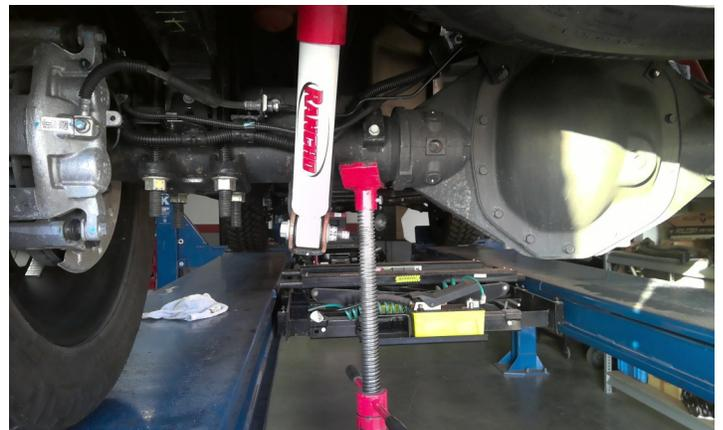
Loosen but do not remove the U-bolts on the side of the axle. This will allow slack. With a suitable jack remove the U-bolts on the opposite side and discard.
