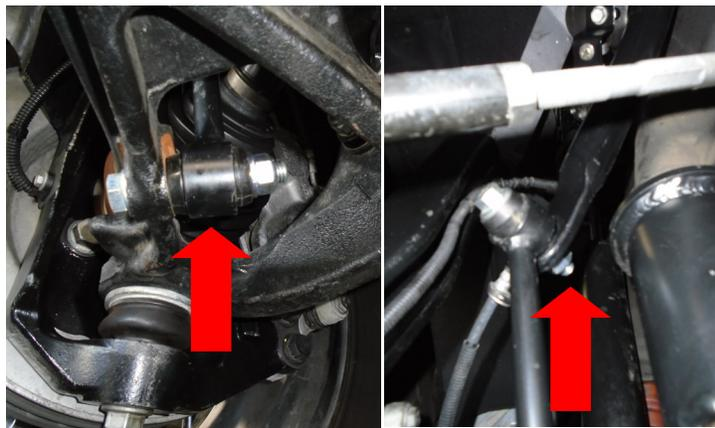
Install the ReadyLIFT front skid plate using the provided **3/8" bolts and washers**. Torque to **30 ft-lbs**.
