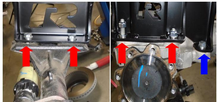
Torque all diff hardware **95 ft-lbs** starting with the driver and passenger side upper hardware first. Then driver lower hardware. When tightening the passenger side lower hardware, make sure to "center" the bracket in the diff's slotted mount. Verify that the diff clears the frame cut made earlier. If not, trim more frame material out until a minimum 1/4" clearance is gained. The frame should rest right inside the divot in the diff housing between the middle and last bolt bosses.
