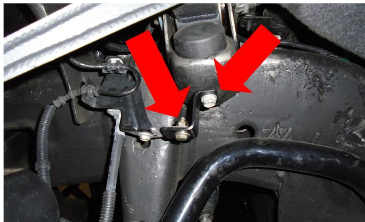
Attach the wheel speed sensor to the steering knuckle. Use factory hardware. Torque to **10 ft-lbs**.
