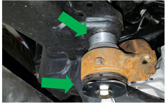
Install the ReadyLIFT passenger side diff drop to the diff cradle using the provided **M12 nuts and washers**. Do not tighten at this time.
