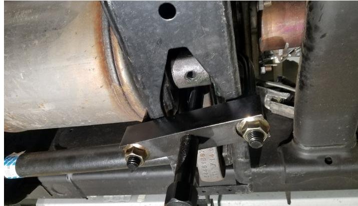
Install factory adjustment bolt. Set the bolt to the recorded Measurement from page 7.
