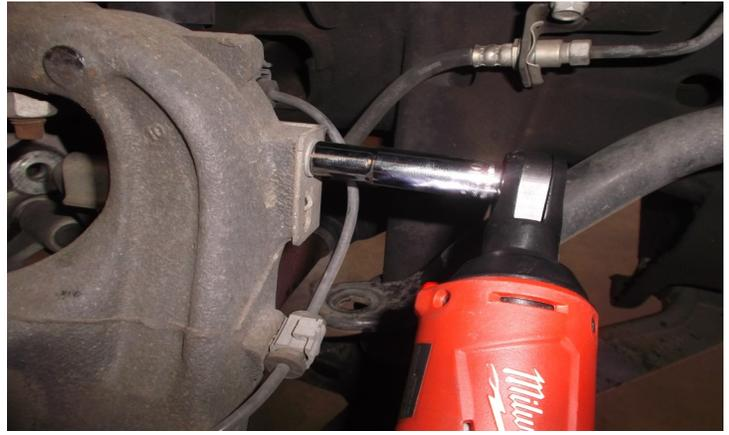
Remove all ABS wire clips and brake line brackets at the frame and knuckle.
