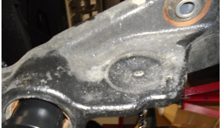
Install the 7/16" bolt, washer, and top lock nut. Torque to 55 ft-lbs.
