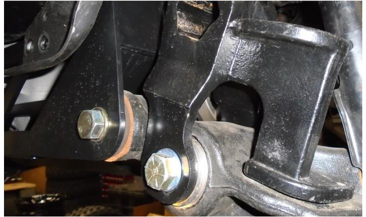
Mark the location of the lower control arm attachment hole. It can help to use the 7/16" drill for this operation.
