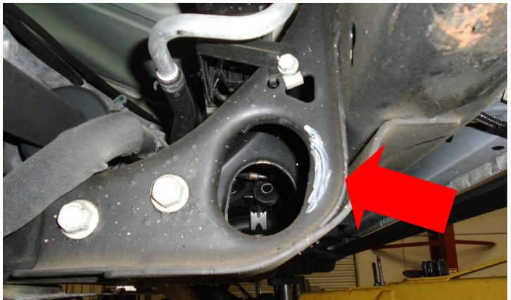
Using a suitable cutting tool, cut along the previous made marks. Remove and discard the outer portion of the cross member. Paint the exposed metal with a quality rust preventative paint.
