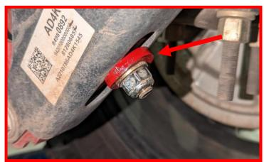
Install shock into extension using supplied M14x80mm bolt.
