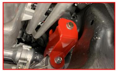
Install passenger differential drop bracket using factory hardware.
