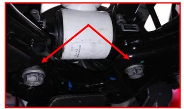
Remove the (3) top strut mounting nuts located on top of the strut tower. Remove strut assembly from vehicle.
