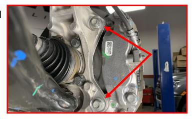
Remove brake rotor retaining bolt and remove the rotor.
