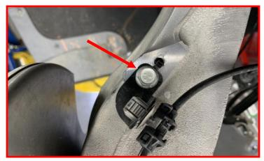
Remove the wheel speed sensor from the knuckle and hang out of the way.
