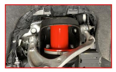
Remove the lower nut clips from the strut and discard.
