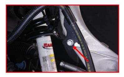
Remove the ABS sensor harness bracket from the knuckle.
