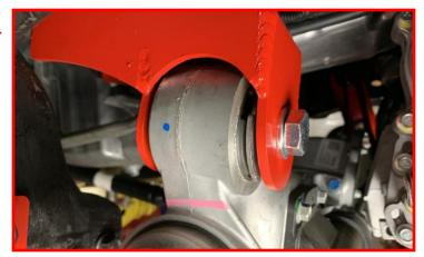
Tighten driver differential drop bracket hardware.
