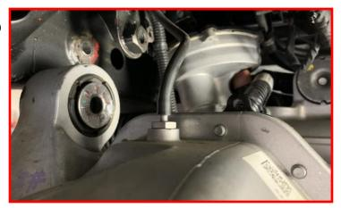
Unplug electrical connector on top of the differential.
