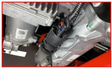
Plug in electrical connector on top of differential.
