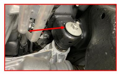
Remove driver side differential mounting hardware. Retain the factory hardware.
