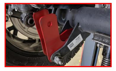
Install factory fastener between lower shock extension and lower shock axle bracket.
