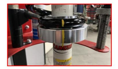
Install front strut spacers using factory nuts.
