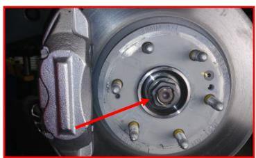
Remove brake caliper mounting bolts and hang caliper out of the way. Do not hang the caliper by the brake line.
