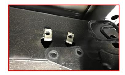
Remove ABS sensor harness bracket from top of rear differential.
