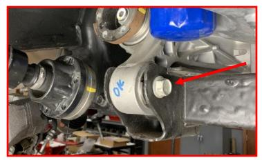
Remove the (4) rear crossmember mounting bolts. Remove crossmember from the vehicle and discard.
