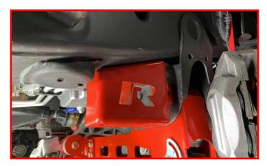
Install sway bar using the supplied M10 bolts, washers and nuts hardware.
