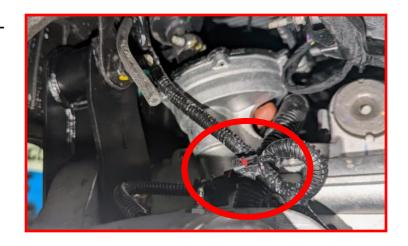
Using supplied vent line extension and vent line connector, extend the vent line and re-install into the differential.
