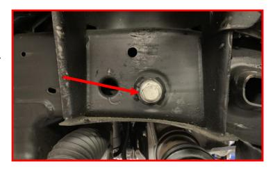
Using the inside edge of the rear control arm/ rear crossmember pocket, measure towards the outside of the vehicle frame 1.625" and make a vertical mark on both sides of the frame. Connect the two lines across the top of the frame rail. Using an appropriate cutting tool, cut through marked line. Sand the cut surface to remove any sharp edges. Paint the cut surface to prevent any corrosion.
