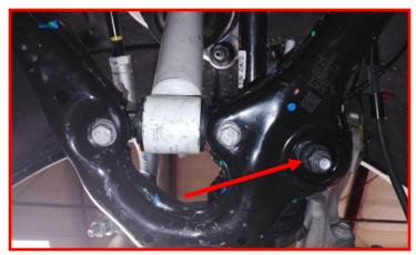
Loosen but do not remove the upper control arm ball joint nut. Strike the upper ball joint boss on knuckle with a dead blow hammer to dislodge the taper. Remove nut and let knuckle hang out of the way.
