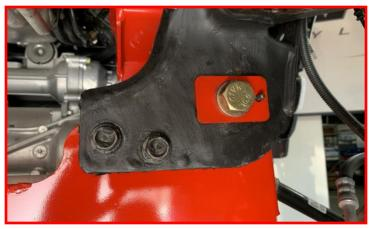
Install the (1) factory rear crossmember bolt and nut and supplied cam block off plates, M18 bolt, washers and nut through the driver side factory mount and replacement crossmember.
