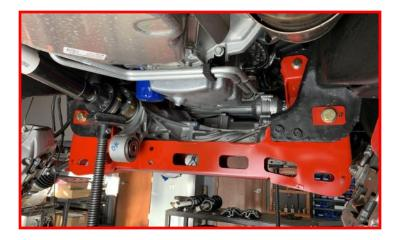
Install the (2) factory rear crossmember bolts and nuts and supplied cam block off plates, M18 bolt, washers and nut through the passenger side factory mount and replacement crossmember.
