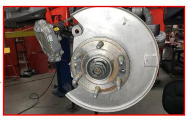
Insert ball joint stud into knuckle taper and attach the upper ball joint to the knuckle using provided hardware.
