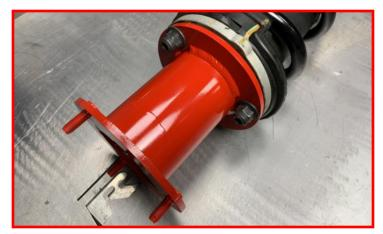
Install strut assembly into vehicle using the provided M10 serrated flange nuts.
