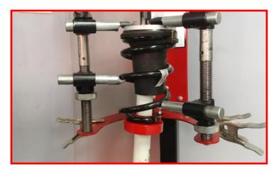
Note: Ensure orientation of the strut assembly is same as factory.
