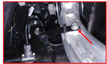
Remove the ABS sensor harness and brake line bracket from the knuckle and hang out of the way.
