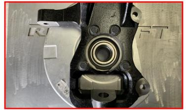
Install the completed knuckle assembly to the lower ball joint using the factory hardware while guiding the CV axle through the hub.
