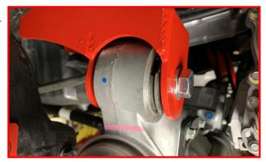
Tighten driver differential drop bracket hardware.
