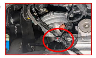
With an appropriate jack stand, support the front differential and remove the rear differential mounting hardware.
