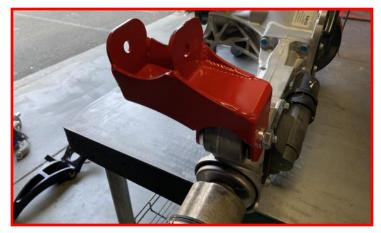
Install driver side differential drop on factory differential mounting point using the supplied M14 x 90mm bolt, washers and nut.
