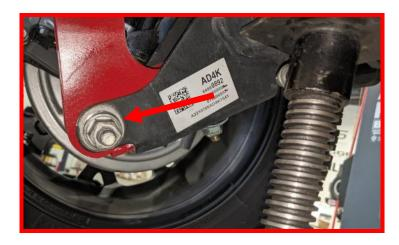
Install supplied M12x30mm bolt into slot on axle shock bracket, along with supplied 12mm washers and the supplied 1/4" thick ReadyLIFT washer.
