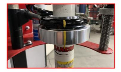
Install front strut spacers using factory nuts.
