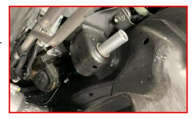
Raise differential into place. Be sure to use a helper to aid in the installation process. With the differential in place, install provided M14 x 110mm Bolt, washers and nut through the passenger differential drop bracket.
