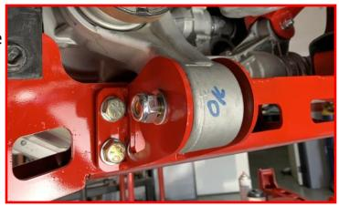
Tighten passenger differential drop bracket hardware.
