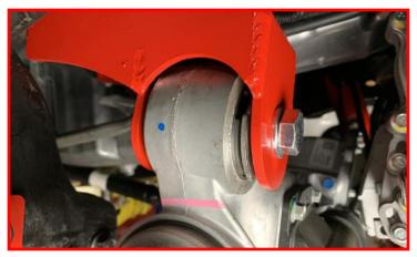
Tighten driver differential drop bracket hardware.
