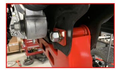
Install the heavy duty skid plate using the provided M10 bolts, washers and nuts.
