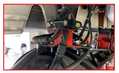
Install the rear wheels and lower vehicle to the ground. Torque the lug nuts to the wheel manufacturer specs, the U-bolts to 110 ft-lbs and all shock hardware to 65 ft-lbs.
