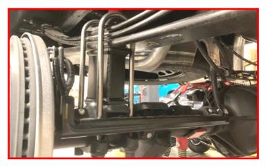
Install the performance aftermarket shock into the frame using factory hardware. Do not tighten at this time.
