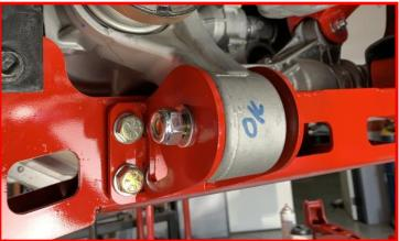
Tighten passenger differential drop bracket hardware.
