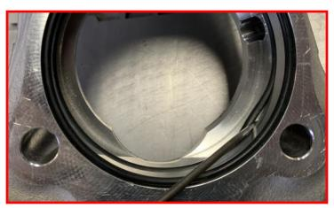
Install the o-rings from the factory knuckle into the replacement knuckle, take care when installing not to tear the o-rings.
