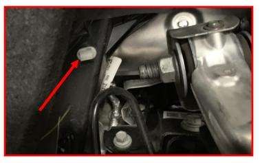
Route the ABS wire under the tie rod end boss on the knuckle and over the CV axle. Install ABS sensor into knuckle using the factory hardware.
