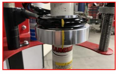
Install front strut spacers using factory nuts.
