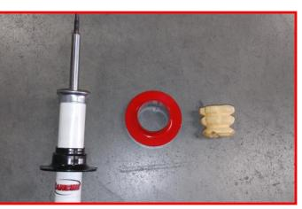
Install shock into to spring. Using the spring compressor, Compress spring and install the factory shock nut. Tighten and torque to 30 ft-lbs.
