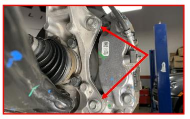
Remove brake rotor retaining bolt and remove the rotor. Retain the factory hardware.
