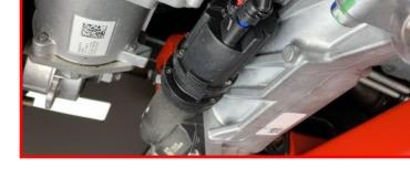
Install vent line. It is necessary to pull down on the vent line to gain the slack needed for installation.
