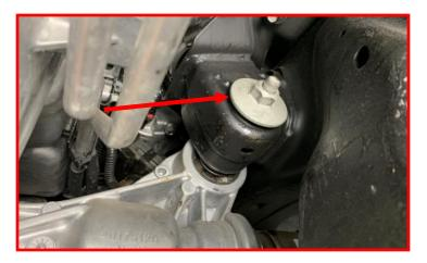
Remove driver side differential mounting hardware.
