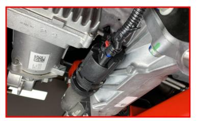
Plug in <u>electrical connector</u> on top of differential.
