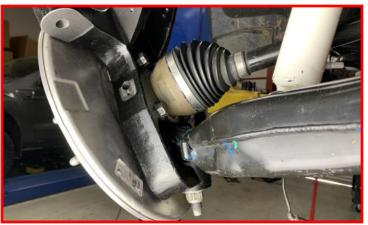
Note: BOTH sides CV axle will receive a 1/4" aluminum spacer. Install onto the CV axle with the chamfered side towards the axle.
