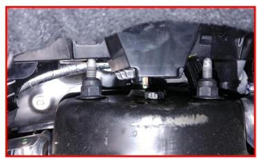
Remove the ABS sensor harness bracket from the knuckle.
