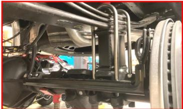
Install rear shock extensions into shock axle brackets.
