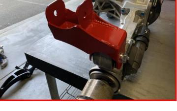
Install passenger differential drop bracket using factory hardware.
