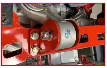
Tighten passenger differential drop bracket hardware.
