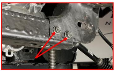
Remove passenger side differential mounting hardware.
