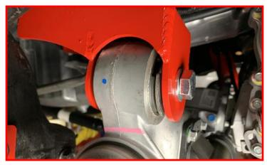
Tighten driver differential drop bracket hardware.
