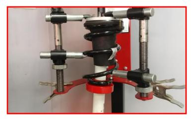
Install strut top spacer onto strut assembly. Using the supplied M10 nuts, install, tighten and torque nuts to 35-ft/lbs.
