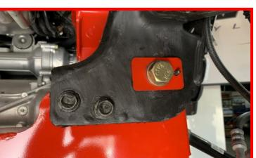
Using the factory cam bolts, cams and nuts, install the lower control arms in the factory orientation. Do not tighten at this time.
