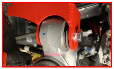
Tighten driver differential drop bracket hardware.
