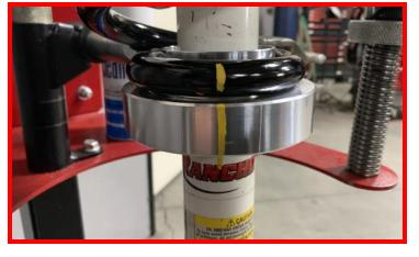
Install front strut spacers using factory nuts.
