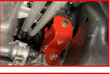
Install the (2) factory rear crossmember bolts and nuts and supplied cam block off plates, M18 bolt, washers and nut through the passenger side factory mount and replacement crossmember. Do not tighten hardware as this time.
