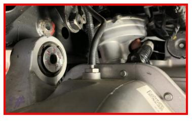
With an appropriate jack stand, support the front differential and remove the rear differential mounting hardware. Retain the factory hardware.
