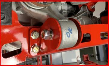
Tighten passenger differential drop bracket hardware.
