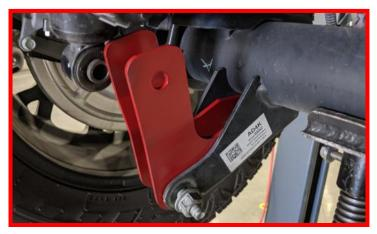
Install factory fastener between lower shock extension and lower shock axle bracket. Do not tighten at this time.
