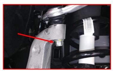
Support the lower control arm with a suitable jack. Remove the lower strut mounting bolts from the lower control arm. Discard factory bolts.
