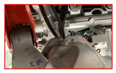
Using a suitable jack, lift differential up and ensure there is clearance between the differential and rear crossmember. Tighten rear differential drop hardware.
