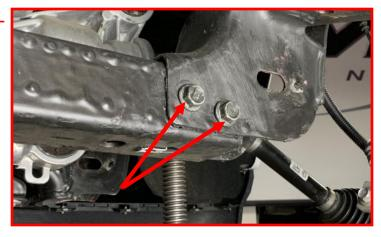
Remove passenger side differential mounting hardware. Discard the hardware.
