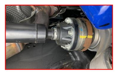
Unplug differential shift actuator. Ensure all clips are removed and clear of the differential.
