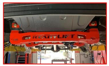
Using the factory cam bolts, cams, washers and nuts, install the lower control arms in the factory orientation.
