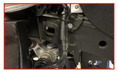
Install the sway bar drop link into the lower control arm using factory nut.
