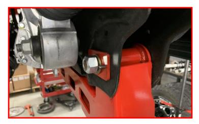
Install the heavy duty skid plate using the provided M10 bolts and washers.
