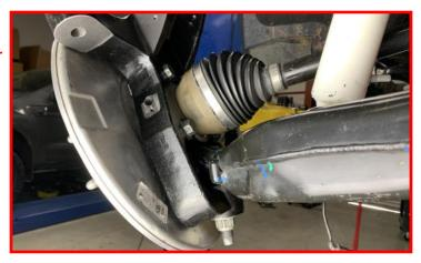
Note: driver side CV axle will receive a 1/4" aluminum spacer. Install onto the CV axle with the chamfered side towards the axle.
