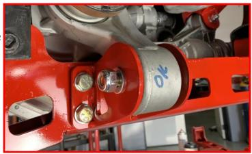
Tighten passenger differential drop bracket hardware.
