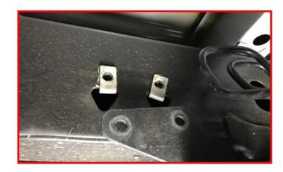
Remove ABS sensor harness bracket from top of rear differential. Retain the factory hardware.
