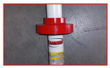
Install shock into to spring. Using the spring compressor, Compress spring and install the factory shock nut. Tighten and torque to 30 ft-lbs.
