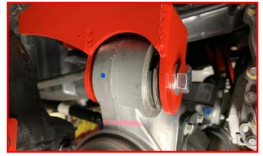
Tighten driver differential drop bracket hardware.
