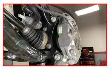
To gain the length needed to reach the ABS sensor mounting location it is necessary to remove the ABS sensor harness from the clip located passenger side inner fender.
