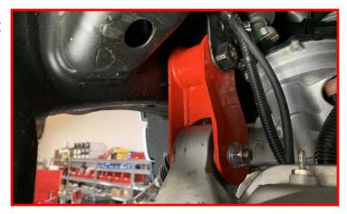
Install rear crossmember using the supplied cam block off plates, M18 bolts, washers, and nuts. Do not tighten at this time.
