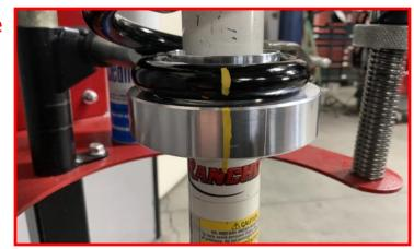
Install front strut spacers using factory nuts.
