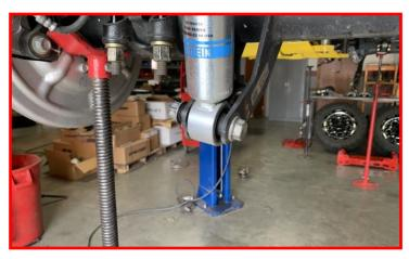
Install the brake line drop bracket to the factory brake line bracket using the supplied M8 bolts, washers and nuts.
