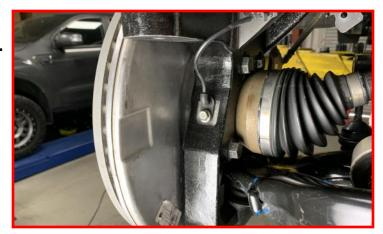
Install ABS sensor harness bracket to the front of knuckle using the factory mounting hardware.
