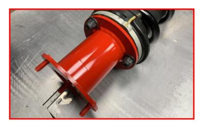
Install strut assembly into vehicle using the provided M10 serrated flange nuts. Do not tighten at this time.
