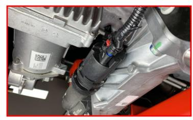
Install vent line. It is necessary to pull down on the vent line to gain the slack needed for installation.
