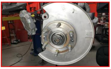
Install the upper ball joint to the knuckle using the provided hardware.
