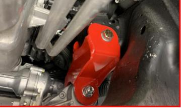
Install passenger differential drop bracket using factory hardware. Do not tighten at this time.
