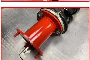
If the strut still has the lower clip nuts attached, remove and discard.
