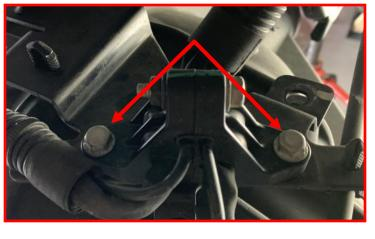
Support the axle with a suitable jack. Remove both driver and passenger shocks from vehicle and discard.
