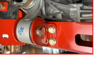
Install front crossmember using the supplied cam block off plates, M18 bolts, washers, and nuts. Do not tighten at this time.
