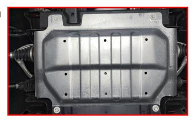
Using (2) of the factory skid plate bolts, install into the two gravel guard bolt holes.
