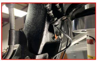
Using a couple wire ties, secure the ABS sensor harness/ brake pad sensor to the brake line.
