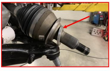
Ensure the CV axle is properly inserted into the hub assembly. Install and tighten axle nut.
