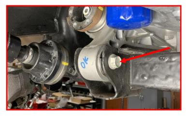
Remove the (4) rear crossmember mounting bolts. Remove crossmember from the vehicle and discard. Retain (3) of the crossmember mounting bolts and nuts.
