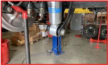
Install the brake line drop bracket to the factory brake line bracket using the supplied M8 bolts, washers and nuts.
