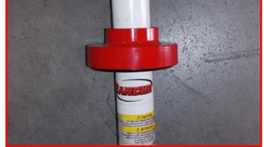
Install shock into to spring. Using the spring compressor, Compress spring and install the factory shock nut. Tighten and torque to 30 ft-lbs.
