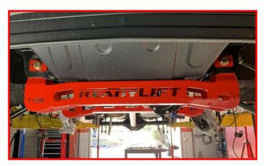
Using the factory cam bolts, cams and nuts, install the lower control arms in the factory orientation. Do not tighten at this time.
