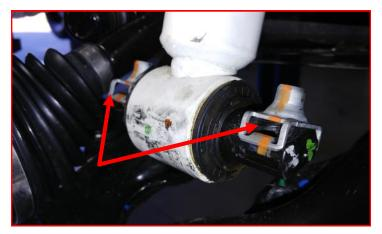
Swing lower control arm up, Install supplied M10 bolts through strut cross pin and lower control arm. Install M10 washers, and nuts on to bolts.
