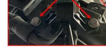
Support the axle with a suitable jack. Remove both driver and passenger shocks from vehicle and discard.
