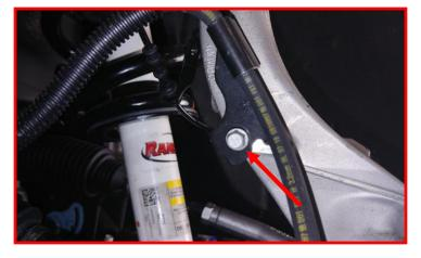
Remove the ABS sensor harness bracket from the knuckle. Retain the factory hardware.
