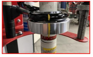
Install front strut spacers using factory nuts.
