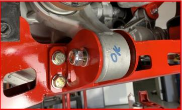
Tighten passenger differential drop bracket hardware.
