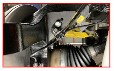
Install ABS sensor harness bracket to the back of knuckle by flipping bracket over and mounting bracket with the factory mounting hardware.
