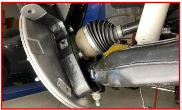
Note: driver side CV axle will receive a 1/4" aluminum spacer. Install onto the CV axle with the chamfered side towards the axle.
