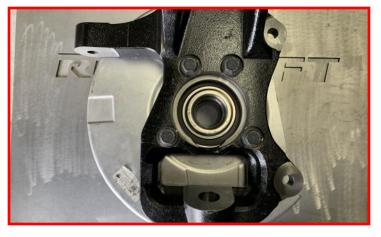
Install the completed knuckle assembly to the lower ball joint using the factory hardware while guiding the CV axle through the hub.
