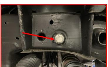
Measure from the pinion seal forward 6" and mark location. Measure from the outside of the fin inward approximately .375" and mark the location. Connect the two marks. Using an appreciate cutting tool cut away the material while following the marked line. Repeat steps for the bottom fin as well.
