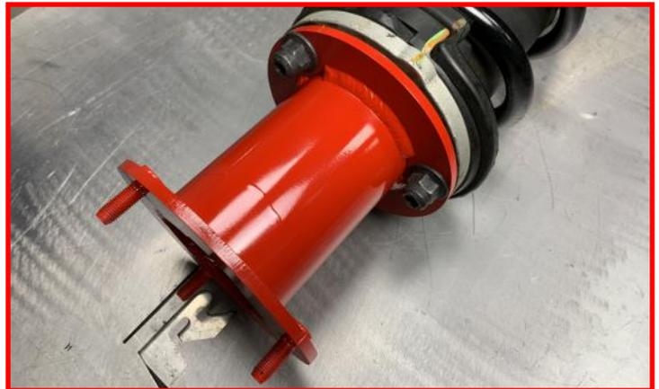
Install strut assembly into vehicle using the provided M10 serrated flange nuts. Do not tighten at this time.
