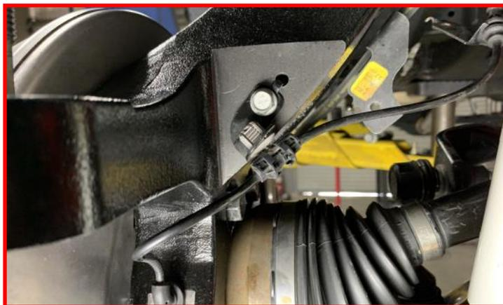
Torque the factory hardware to **80-in/lbs.**
