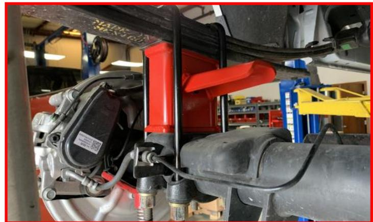
Install the performance aftermarket shock into the frame using factory hardware. Do not tighten at this time.
