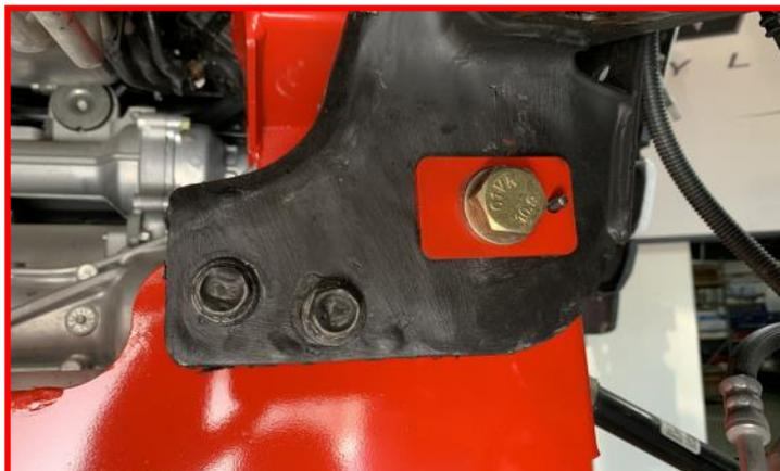
Install the (1) factory rear crossmember bolt and nut and supplied cam block off plates, M18 bolt, washers and nut through the driver side factory mount and replacement crossmember. Do not tighten hardware as this time.
