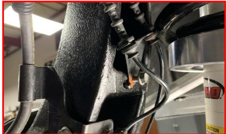
Using a couple wire ties, secure the **ABS sensor harness/ brake pad sensor** to the brake line.
