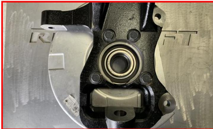
Install the completed knuckle assembly to the lower ball joint using the **factory hardware** while guiding the CV axle through the hub.
