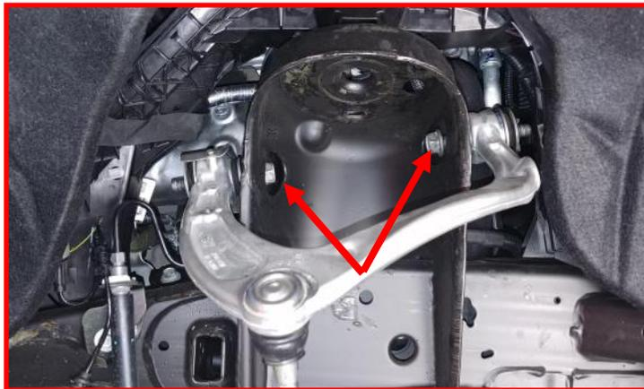
Remove **(4) sway bar mounting bolts** from the frame. Remove sway bar from the vehicle and retain factory hardware.
