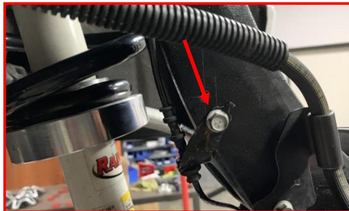
Torque the factory hardware to **80-in/lbs.**
