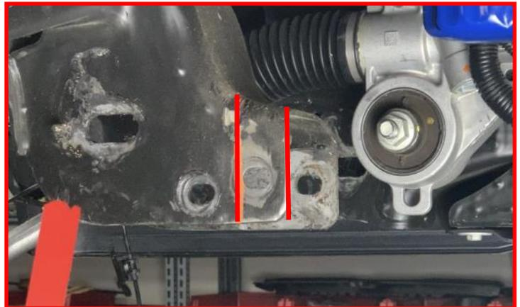
Measure from the pinion seal forward 6" and mark location. Measure from the outside of the fin inward approximately .375" and mark the location. Connect the two marks. Using an appropriate cutting tool cut away the material while following the marked line. Repeat steps for the bottom fin as well.
