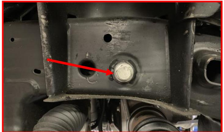
Using the inside edge of the rear control arm/ rear crossmember pocket, measure towards the outside of the vehicle frame 1.625" and make a vertical mark on both sides of the frame. Connect the two lines across the top of the frame rail. Using an appropriate cutting tool, cut through marked line. Sand the cut surface to remove any sharp edges. Paint the cut surface to prevent any corrosion.
