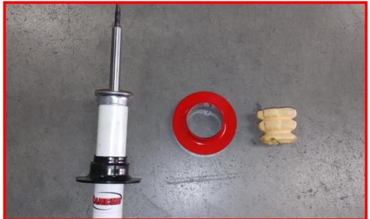
Install the **billet pre-load spacer** on top of factory spring perch. The spacer should nest onto the factory spring perch.
