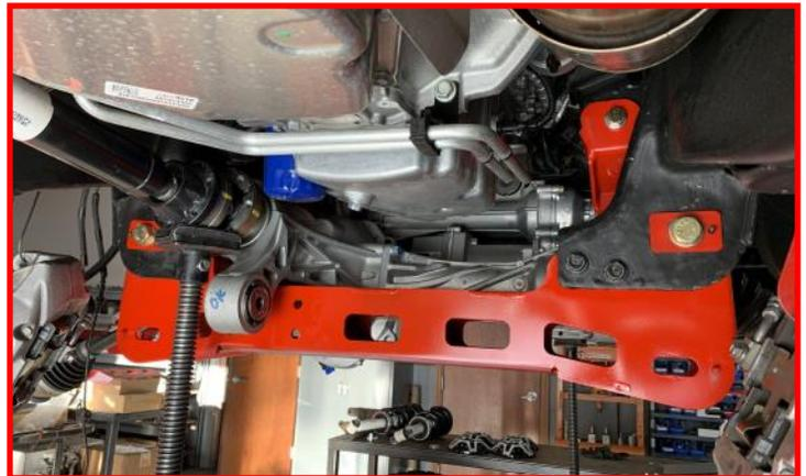
Install the (2) factory rear crossmember bolts and nuts and supplied cam block off plates, M18 bolt, washers and nut through the passenger side factory mount and replacement crossmember. Do not tighten hardware as this time.
