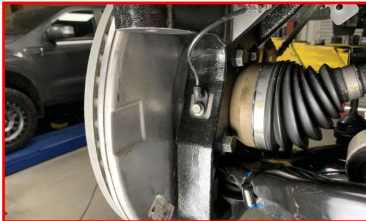
Torque the factory hardware to **80-in/lbs.**
