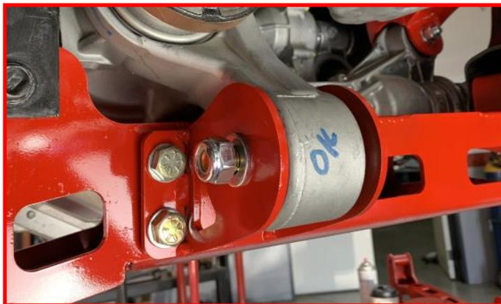
Tighten **passenger differential drop bracket** hardware.
