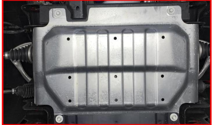
Using (2) of the factory skid plate bolts, install into the two gravel guard bolt holes.
