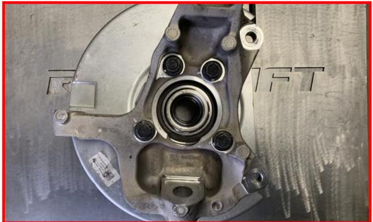
Remove the O-rings from factory knuckle, be careful not to tear the O-rings when removing .
