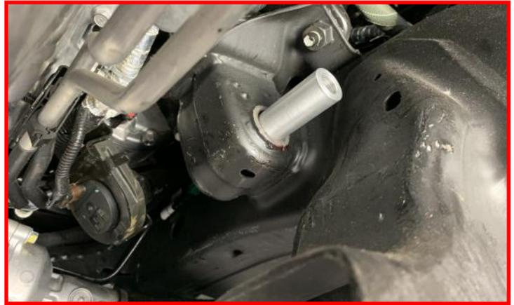
Raise differential into place. Be sure to use a helper to aid in the installation process. With the differential in place, install provided **M14 x 110mm Bolt, washers and nut** through the passenger differential drop bracket. Do not tighten at this time.
