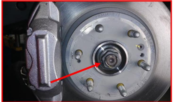
Remove **brake caliper mounting bolts** and hang caliper out of the way. Do not hang the caliper by the brake line. Retain factory hardware.
