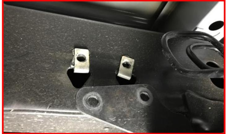
Remove **ABS sensor harness bracket** from top of rear differential. Retain the factory hardware.
