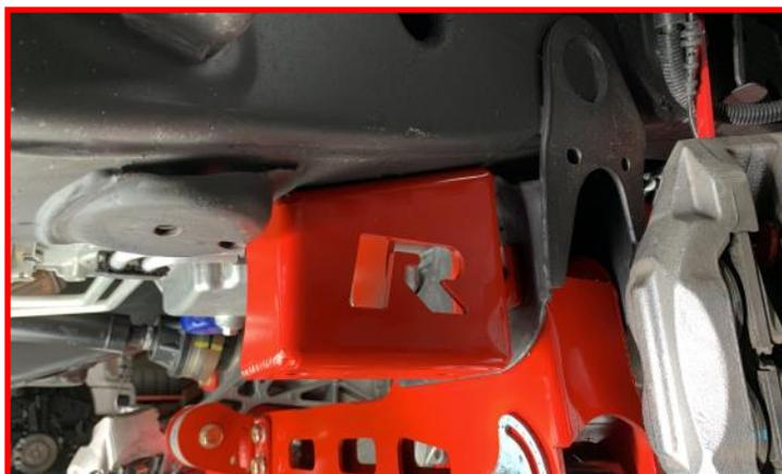
Install **sway bar** using the supplied M10 bolts, washers and nuts hardware.
