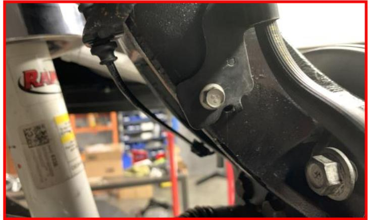
Using a couple wire ties, secure the **ABS sensor harness** to the brake line.
