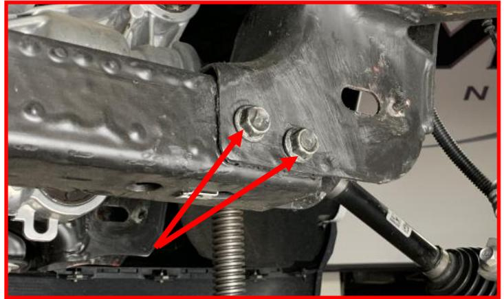
Remove passenger side differential mounting hardware. Discard the hardware.
