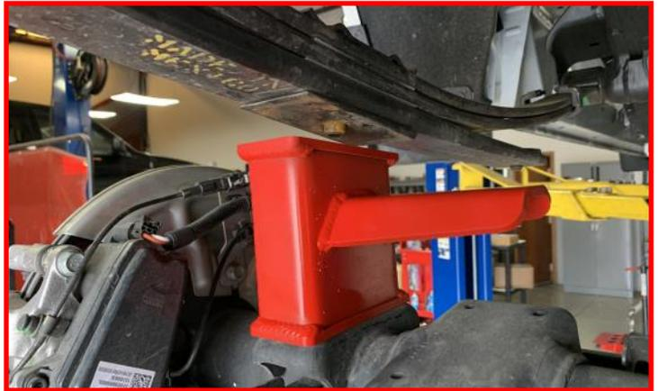
Install the provided U-bolts, and nuts. Snug the U-bolt nuts but do not fully tighten at this time. Repeat steps for passenger side.
