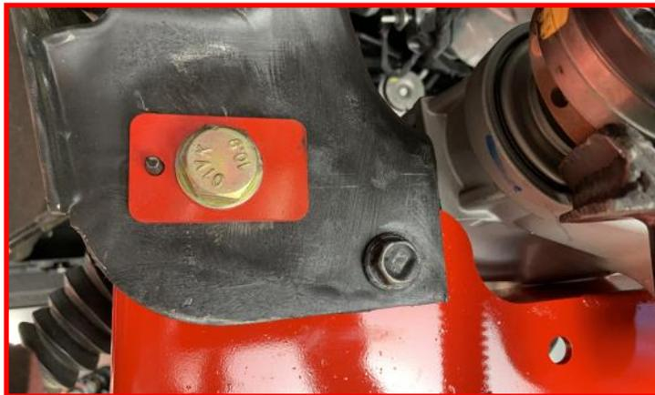
Install rear differential drop onto rear crossmember using the (4) supplied 1/2" bolts, washers and a drop of thread locker.
