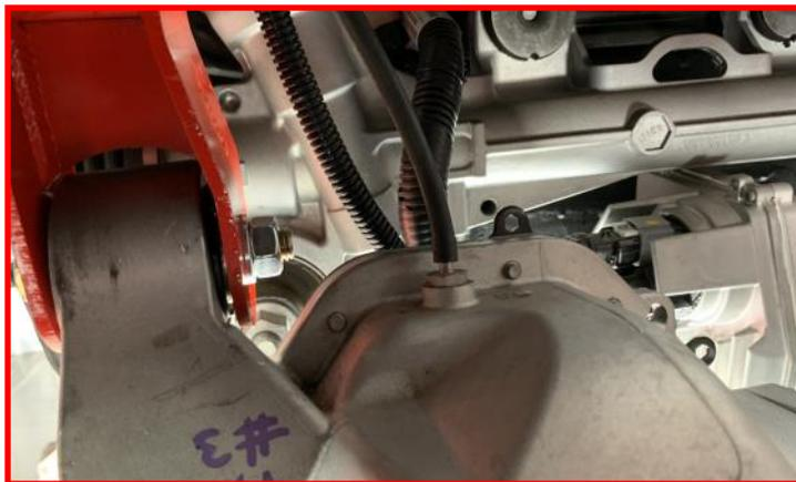
Using a suitable jack, lift differential up and ensure there is clearance between the differential and rear crossmember. Tighten rear differential drop hardware.
