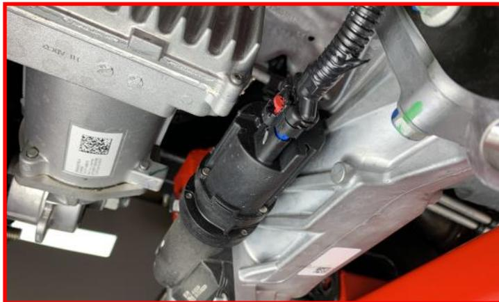
Install vent line. It is necessary to pull down on the vent line to gain the slack needed for installation.
