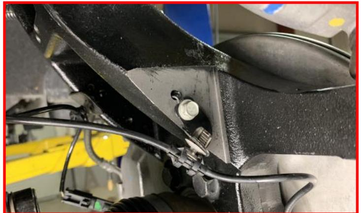
Install **brake pad sensor bracket** to the back of knuckle by flipping bracket over and mounting bracket with the **factory mounting hardware**.
