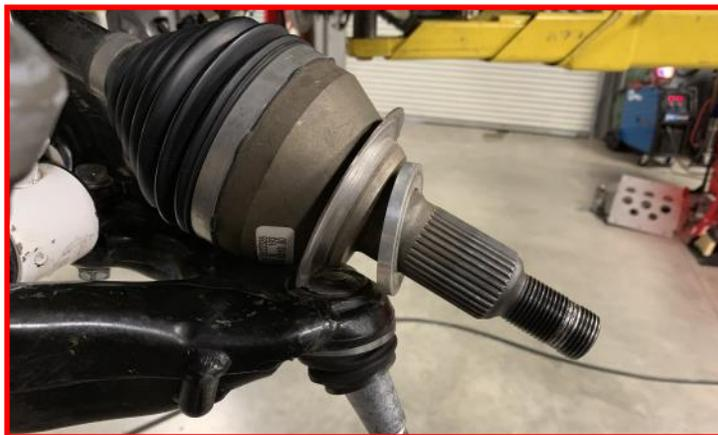
Ensure the CV axle is properly inserted into the hub assembly. Install and tighten **axle nut**.
