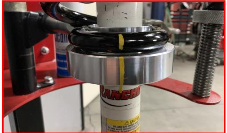
Install front strut spacers using factory nuts.
