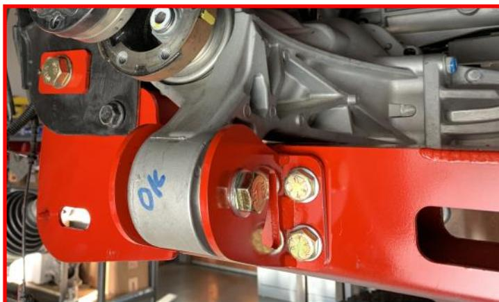
Install front crossmember using the supplied cam block off plates, M18 bolts, washers, and nuts. Do not tighten at this time.
