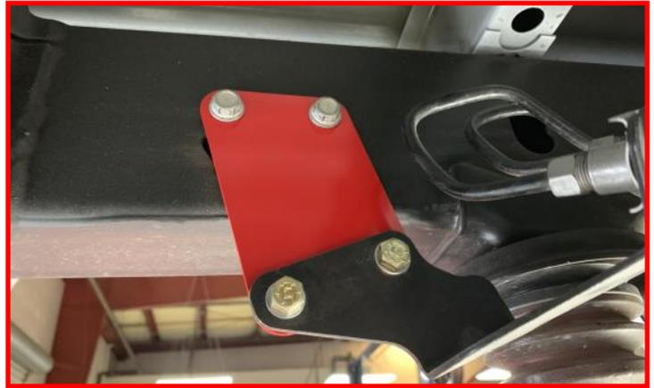
Install ABS harness drop bracket to the axle using the factory hardware.
