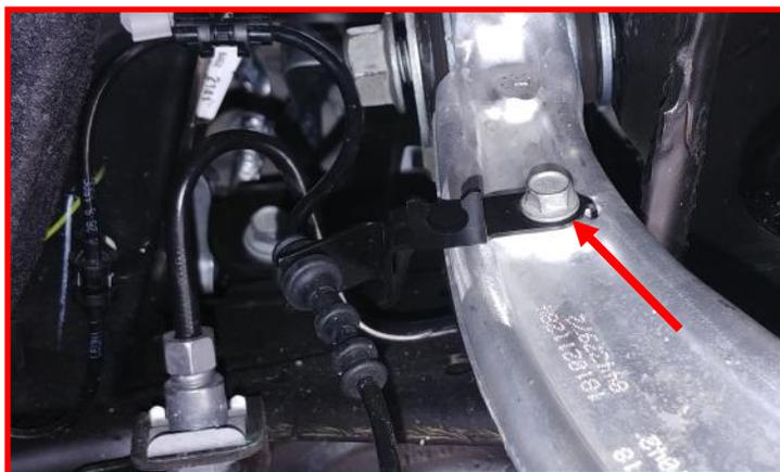
Remove the **ABS sensor harness and brake line bracket** from the knuckle and hang out of the way. Retain the factory hardware.
