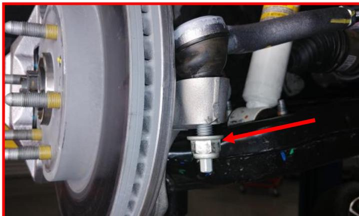
Remove the **ABS bracket** from the upper control arm. Remove ABS sensor harness from bracket and discard bracket.
