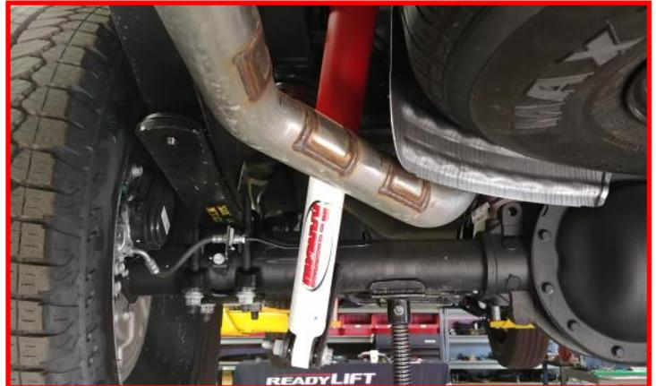
Remove the driver side U-bolts completely and discard. Lower the axle enough to ensure clearance to install lift block making sure that all brake lines and ABS lines do not get over extended.
