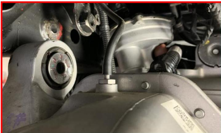
With an appropriate jack stand, support the front differential and remove the rear **differential mounting hardware**. Retain the factory hardware.
