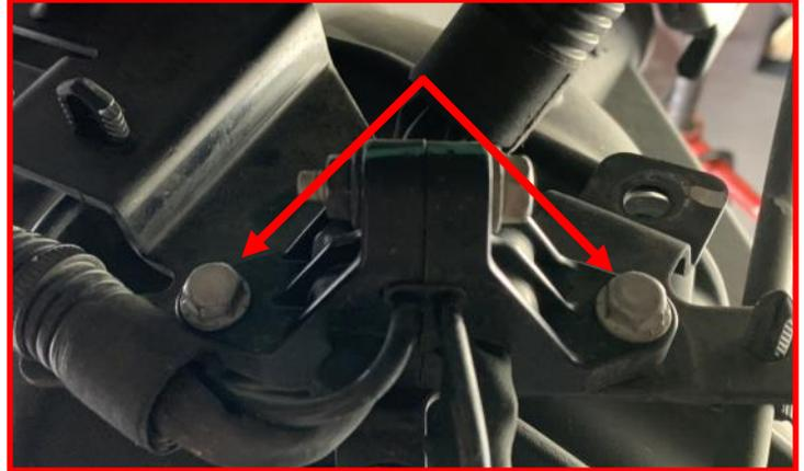
Support the axle with a suitable jack. Remove both **driver and passenger shocks** from vehicle and discard.
