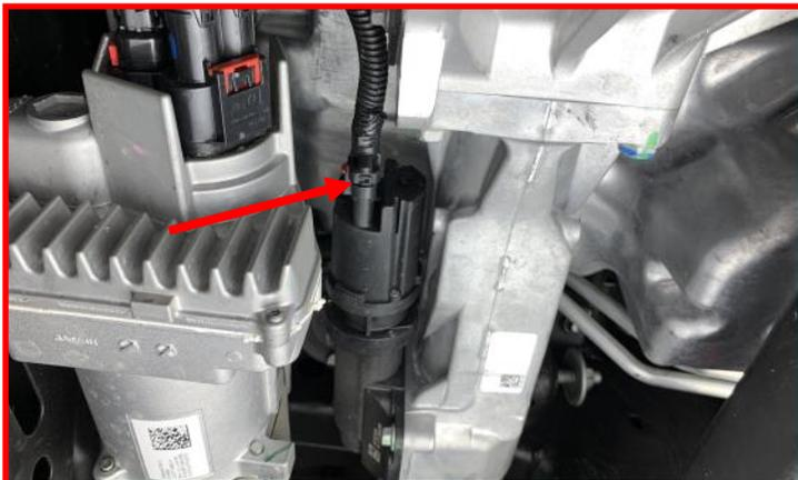
Remove **differential vent line** from the top of the differential.
