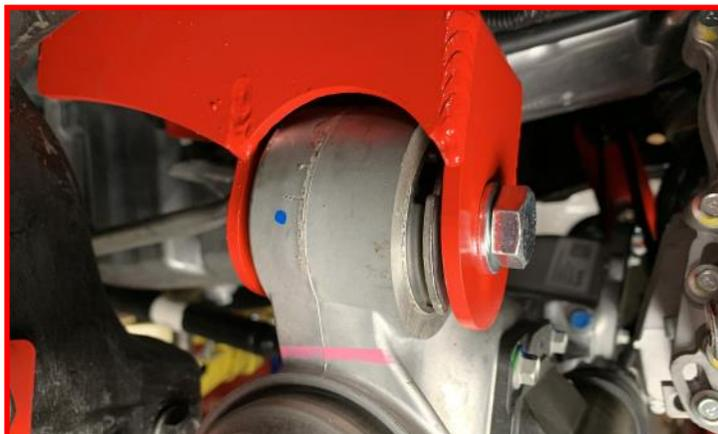
Tighten **driver differential drop bracket** hardware.
