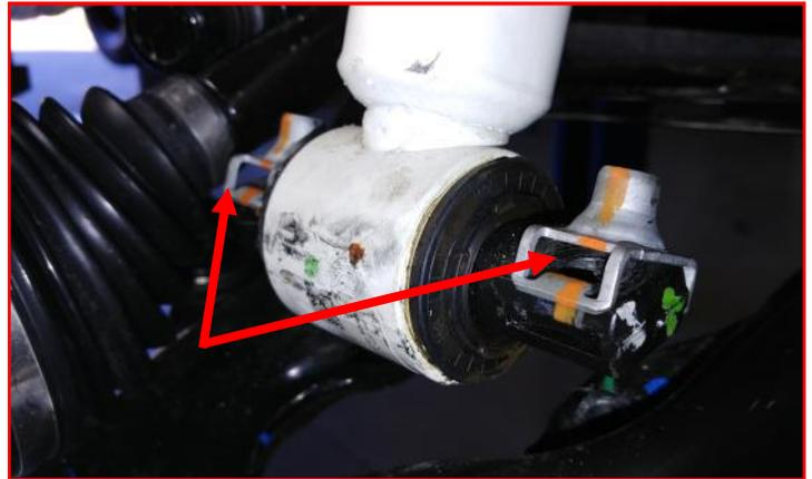
Swing lower control arm up, Install supplied **M10 bolts** through strut cross pin and lower control arm. Install **M10 washers, and nuts** on to bolts.
