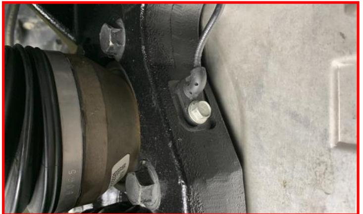
Install **ABS sensor harness bracket** to the front of knuckle using the **factory mounting hardware**.
