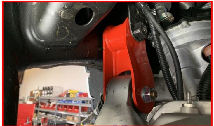
Install **rear crossmember** using the supplied **cam block off plates, M18 bolts, washers, and nuts**. Do not tighten at this time.
