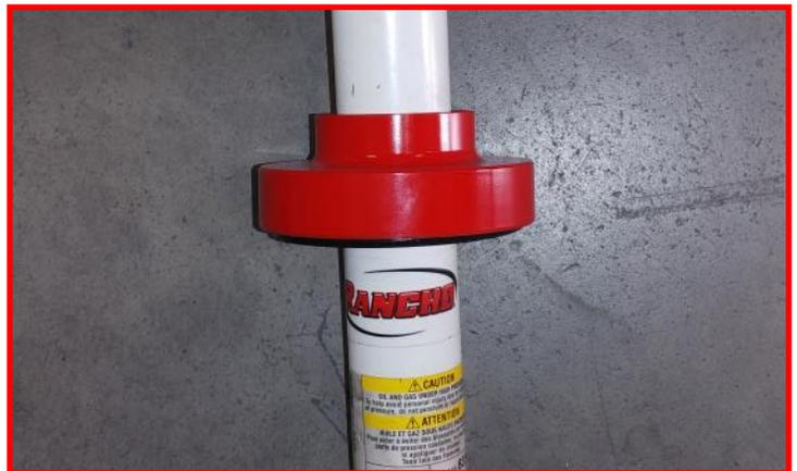
Install shock into to spring. Using the spring compressor, Compress spring and install the factory shock nut. Tighten and torque to 30 ft-lbs.
