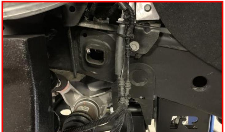
Install the **sway bar drop link** into the lower control arm using factory nut.
