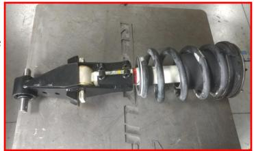
Bolt the two halves together using the provided M12 x 30mm bolts and washers. Do not tighten at this time.
