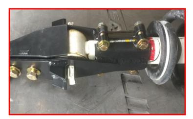
Install the strut cross bar to the strut extension using the provided M10 x 40mm bolts, washers and locking nuts.
