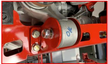
Tighten passenger differential drop bracket hardware.
