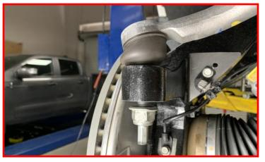
With everything tightened and torqued to the specified specifications, install front tires and lower vehicle. Jounce the suspension to settle it to the new ride height.
