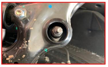
Install the outer tie rod end to the knuckle using factory hardware.
