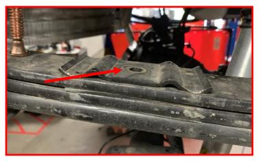
With the overload spring removed from the vehicle, remove the alignment pin from the spring by driving it out using a drift punch and hammer. Discard the alignment pin.
