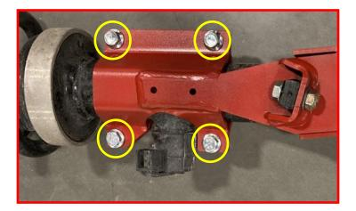
Remove 5mm button cap screw from provided control arm; screw will be installed on the forward side of the arm. RETAIN SCREW.
