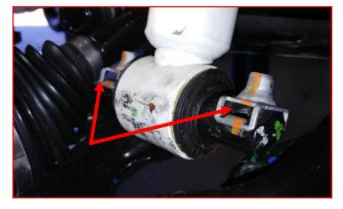
Locate the front clamshell strut extensions and hardware. (M12 x 25mm bolts, washers, M10 x 30mm bolts, M10 x 60mm bolts, washers and locking nuts) You will see the strut extensions are labeled with a "D" and "P". This is to identify the location the extension is to be installed. "D" corresponds with the driver and "P" corresponds with the passenger side. This orientation is important to prevent damage to other suspension and driveline components. Passenger side shown.
