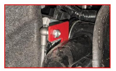
Install strut assembly into vehicle using the factory nuts.
