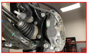
To gain the length needed to reach the ABS sensor mounting location it is necessary to remove the ABS sensor harness from the clip located passenger side inner fender.
