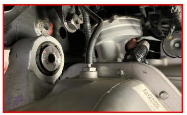
With an appropriate jack stand, support the front differential and remove the rear differential mounting hardware. Discard the factory hardware.
