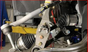
Install provided strut thrust washer on the backside of the strut extension cross pin.
