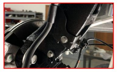
Install ABS sensor harness/ brake pad sensor bracket to the inside of knuckle. It is necessary to remove rubber grommets from bracket and rotate 180 degrees. Ensure the bracket points down and install using the factory mounting hardware.
