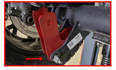
Install supplied M12x30mm bolt into slot on axle shock bracket, along with supplied 12mm washers and the supplied 1/4" thick ReadyLIFT washer. Torque to 50 ftlbs.
