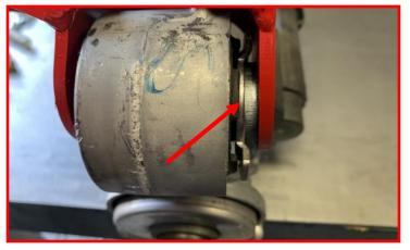
Install passenger side differential drop on factory differential mounting point using the supplied M14 x 100mm bolt, washers and nut. Do not tighten at this time.
