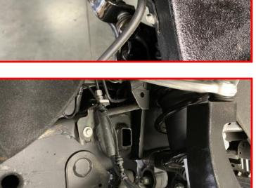
Install ABS sensor harness bracket to the front of knuckle using the factory mounting hardware.
