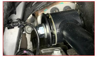
Use the provided M6 nylon locking nut to attach the ball stud to the ARC bracket.
