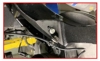
Install brake pad sensor bracket to the back of knuckle by flipping bracket over and mounting bracket with the factory mounting hardware.
