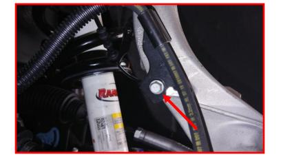
Remove the ABS sensor harness bracket from the knuckle. Retain the factory hard-ware.
