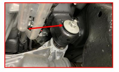
Remove driver side differential mounting hardware. Retain the factory hardware.
