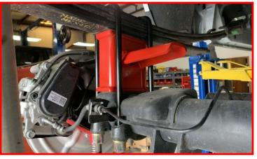
Install rear shock extensions into shock axle brackets using the factory shock hardware.
