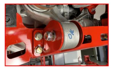
Tighten passenger differential drop bracket hardware.
