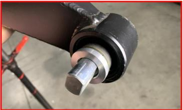
Swing lower control arm up, Install supplied M10x60mm bolts through strut cross pin and lower control arm. Install M10 washers, and nuts on to bolts.
