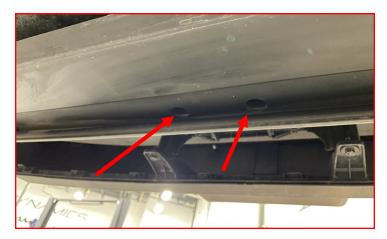
Remove the four (4) bolts for the front dust shield.
