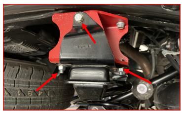
Attach the supplied rear shock to the lower mount using factory hardware.
