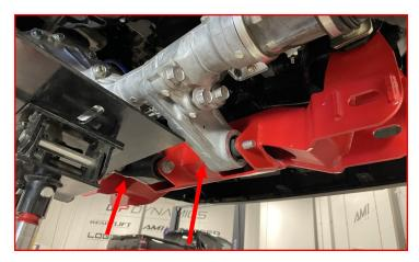
Install the rear crossmember using he supplied M18-2.5 X 160mm hex head bolts, M18-2.5 locking nuts, and M18 flat washers,
