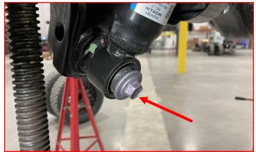
Remove the upper shock nut and bushing.
