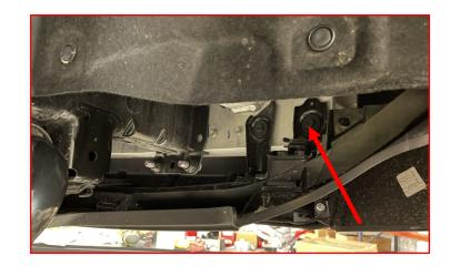
Remove the two (2) screws retaining the factory air dam to the actuator.
