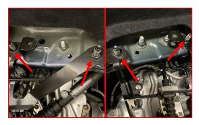
Remove the driver side brake lines from the plastic clip on the inside of the body panel opposite of the bracket removed in the previous step (left image).
