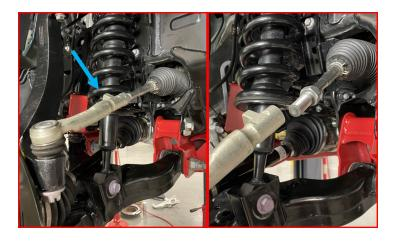
Note how the <u>nub</u> on the tie rod is opposite of the factory location in the previous step.
