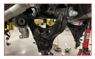
Remove the shock from the vehicle.
