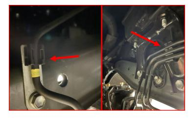
Attach the supplied front brake line bracket 2 (left and right) to the body using factory hardware. Attach the factory brake line bracket to the supplied bracket using the supplied M8-1.25 X hex head bolt, M8-1.25 locking nut, and four (4) M8 flat washers.
