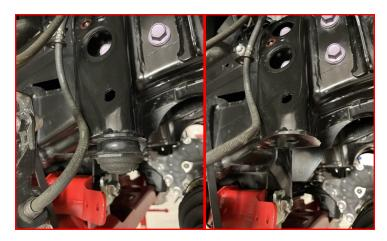
Using the supplied M10-1.25 X 25mm hex head flange bolts (3) and M10-1.25 flange nuts (3), attach the front bump stops to the rear crossmember. Note: the long flange goes towards the rear of the vehicle.
