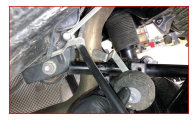
Mate the air ride sensor link to the new sensor relocation bracket using the factory nut. Torque to factory spec.
