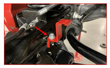
Using the supplied M8-1.25 X 20mm hex head bolt, M8-1.25 locking nut, and two (2) M8 washers attach the brake line to the supplied bracket.
