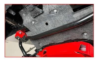
Trim the front air dam 0.25" from the inner edge. Contour the line to blend it into the air dam.
