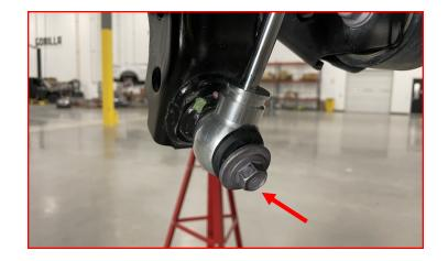
Using the supplied shock hardware, attach the shock to the upper mount.
