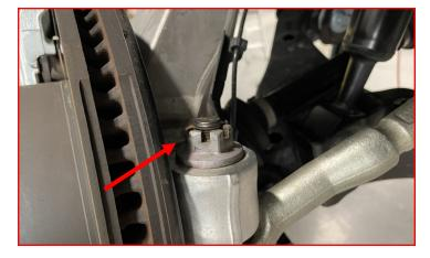
Remove the CV axle dust shield.
