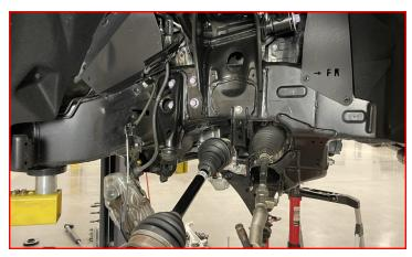
Remove the four (4) nuts holding the drive shaft to the front differential.
