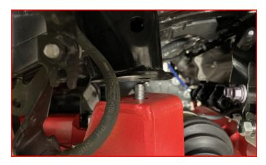
Torque the chassis to differential drop bracket hardware to 110 ft-lbs.
