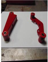
Install the passenger side ReadyLift differential bracket to the front and rear crossmember the pointed end of the bracket goes toward the front of the vehicle. Use provided hardware do not tighten at this time.
