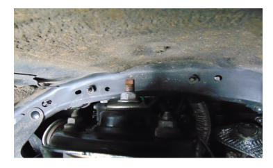
Add the lower strut extension to the strut assembly. Align the lower strut bushing with the through hole on the strut extension. Use factory hardware to fasten torque to 125 ft-lbs. Add the billet clamps to the strut extension use provided hardware torque 35 ft-lbs.
