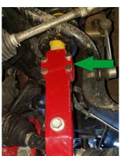
Raise the lower control arm and fasten to the lower strut, use provided hardware hand tight only.
