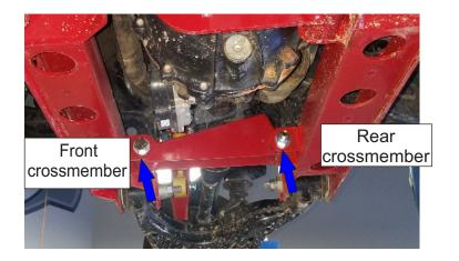
Install the driver side ReadyLift differential bracket to the front only crossmember use provided hardware. Do not tighten at this time.
