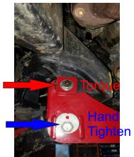
Tighten and torque the passenger differential bolts 75 ft-lbs.
