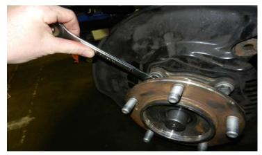
Remove the tie rod nut. Strike the tie rod boss with a hammer to dislodge the taper, and from the knuckle.
