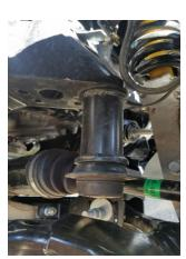
Make alignment marks on the strut assembly. Compress the strut and remove the containment nut. Do not use an air ratchet/gun for this and use a clamp or correct size wrench to hold the top stud. If the stud spins with the nut the shock shaft will unscrew from the shock body, resulting in the shock blowing apart and a new shock will have to be purchased.
