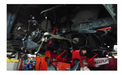
Remove the bump stops by turning them counter clockwise to unscrew from the frame. Install the Ready-Lift extensions onto the frame and bump stops on to the extensions with a drop of thread locker. Tighten down until the bump stop extension bottoms out onto the frame rail.
