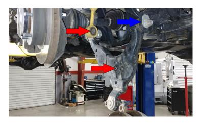
Remove the LCA from the vehicle. Loosen but do not remove the upper control arm. Hold onto the strut, remove the upper strut hardware, remove the strut from the vehicle.
