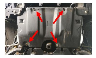
Remove the differential gravel guard.
