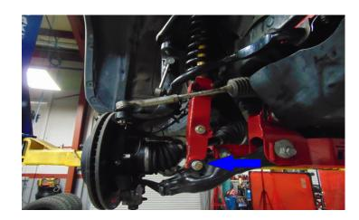
Protect the axle and ball joint boots with a wet rag or other suitable protection from grinding and welding sparks. Clean/grind off the paint/rust on the steering stop on the ball joint cradle. Weld the turn stop extension plates on their corresponding sides (match the contours of the stops) across the top and bottom.
