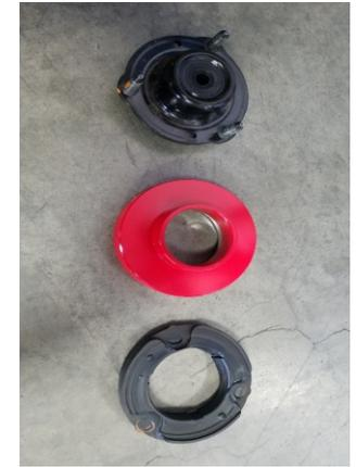
Release the spring tension and remove the factory top hat. Add the ReadyLIFT Spring spacer align the three relief pockets in the spacer to the studs on the top hat. Use the rubber isolator between the spring and aluminum spacer. **Realign the alignment marks** and compress the strut assembly. Reinstall the containment nut and torque to **35 ft-lbs**.
