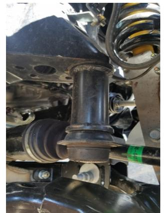
Make **alignment marks** on the strut assembly. Compress the strut and remove the **containment nut**. Do not use an air ratchet/gun for this and use a **clamp or correct size wrench to hold the top stud**. If the stud spins with the nut the shock shaft will unscrew from the shock body, resulting in the shock blowing apart and a new shock will have to be purchased.
