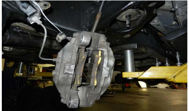
Remove the safety clip from the upper ball joint, cotter pin from the tie rod ends, and axle nut.
