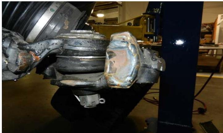
Install the axle bearing. The bearing is a bolt in press fit, start all four bolts, and tighten evenly. Torque to **75 ft-lbs**. Remove the axle dust shield from the OEM steering knuckle, reinstall on the ReadyLift steering knuckle.
