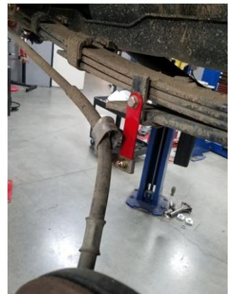
Install the ReadyLIFT rear **carrier bearing spacer** between the carrier bearing housing and the frame. Use the provided hardware. Torque to **35 ft-lbs.**
