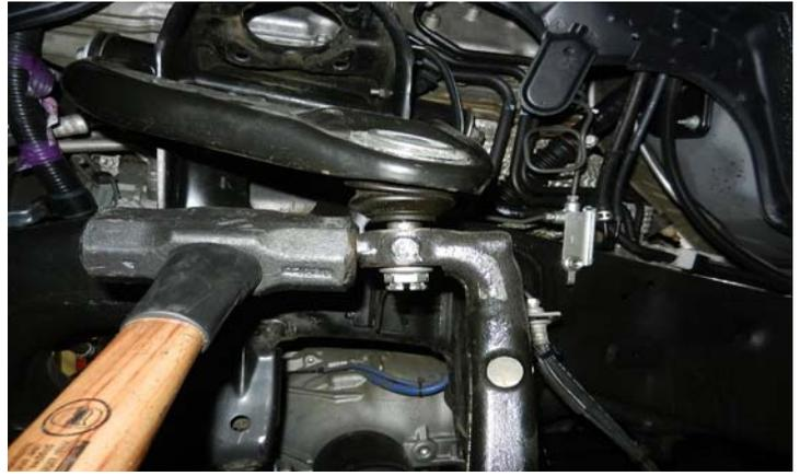
Separate the lower ball joint cradle from the knuckle. Separate the axle from the knuckle and use a S hook or hanger to support the axle. Remove the upper ball joint nut, then remove the knuckle from the vehicle. Note: Hold onto the "knuckle it" will fall during this step.
