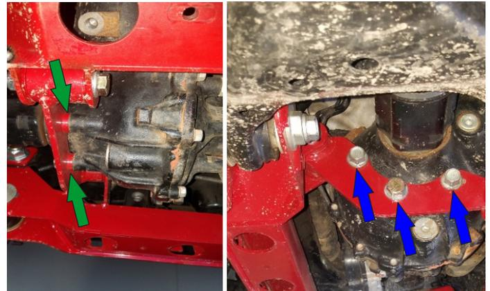
Align the driver side rear differential bracket to the **rear crossmember** mount, use provided hardware. Do not tighten at this time.
