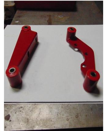
Install the passenger side ReadyLift differential bracket to the front and rear crossmember the pointed end of the bracket goes toward the front of the vehicle. Use provided hardware do not tighten at this time.
