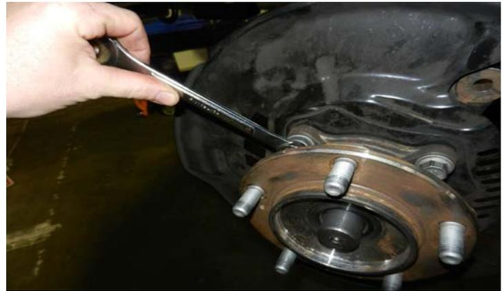
Remove the tie rod nut. Strike the tie rod boss with a hammer to dislodge the taper, and from the knuckle.
