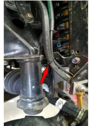
Reinstall the front gravel guard in it's original mounting location. Use factory hardware torque **15 ft-lbs**.
