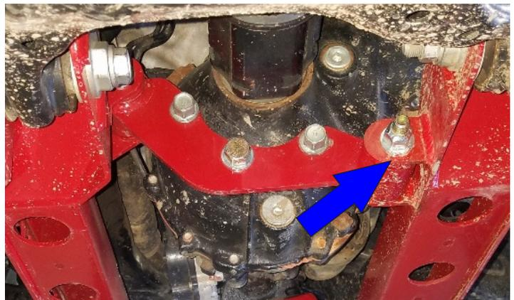
Reinstall the lower control arm to the ReadyLift crossmember use the original **factory hardware**. Do not tighten at this time.
