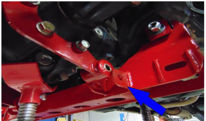
Lower the axle and differential down to the passenger side bracket start the original factory bolts, do not tighten. Rotate the driver side bracket to the differential add the **three laser cut washers** between the bracket and the differential use the original factory bolts to fasten. Do not tighten at this time.
