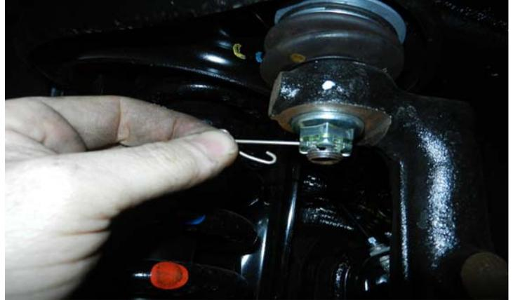
Remove the axle nut keeper and then remove the axle nut.
