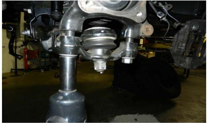
Remove **lower strut hardware**. Loosen the **lower control arm (LCA)** cams and let the LCA swing out of the way.
