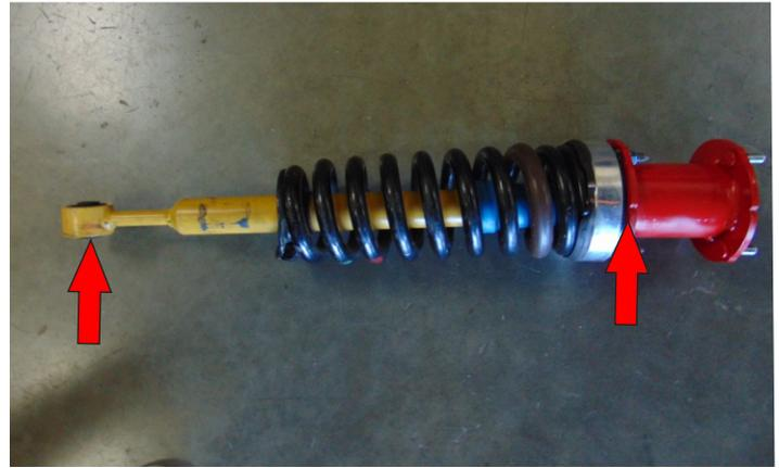
Reinstall the strut to the strut tower on the vehicle, making sure the alignment notches on the spacer face to the outside of the wheel well. Use provided hardware hand tighten only at this time.
