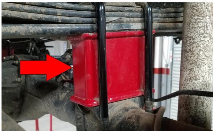
Install the provided **U-bolts, nuts,** and extended length shocks. Snug only at this time, wait until the vehicle is on the ground to torque.
