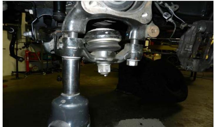
Align the **CV axle spines** with the bearing press it through, spin the hub to be sure you have proper alignment with the axle and bearing. Install the axle nut seat the axle by tightening the nut until the axle locks against the bearing. Torque the axle nut **180 ft-lbs** Reinstall cotter pin.
