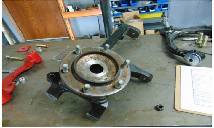
Reinstall the steering knuckle to the upper control arm use factory hardware torque to **67 ft-lbs** then tighten until the castle nut aligns with the cotter pin hole, insert cotter pin. Place the axle in the knuckle bearing block. Raise the lower control arm and reattach the knuckle cradle to the knuckle. Use factory hardware Torque **180 ft-lbs** with a drop of thread locker.
