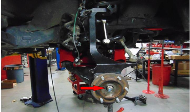
Install the **sway bar end links** to the ReadyLift knuckle. Using a 5mm allen wrench thread the stud through the knuckle. Torque to **50 ft-lbs** the nuts from the OEM knuckle can be discarded.
