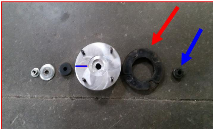
Remove the **rubber bushing** from the factory top hat. The inside bushing is glued in place and requires separation. Install in the same order as removed from the factory parts. Install the strut hat in the same orientation as the factory (**mark on the top of the top hat indicates outward same as factory top hat shown in blue on the picture**) using the **factory hardware**. Torque to **30 ft-lbs**.
