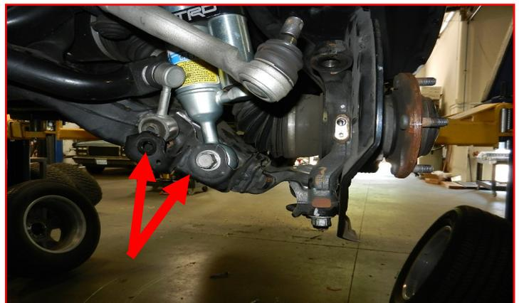
Remove the strut from the frame. Remove the ReadyLIFT strut extension. Make sure to mark them for reassembly later. These are driver and passenger side specific and must go back on their corresponding sides. Mark the spring location to shock body.
