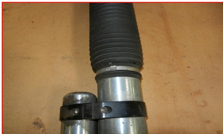
Remove the shock extension from the shock. Save the bushings and adapter sleeve from inside the extension.
