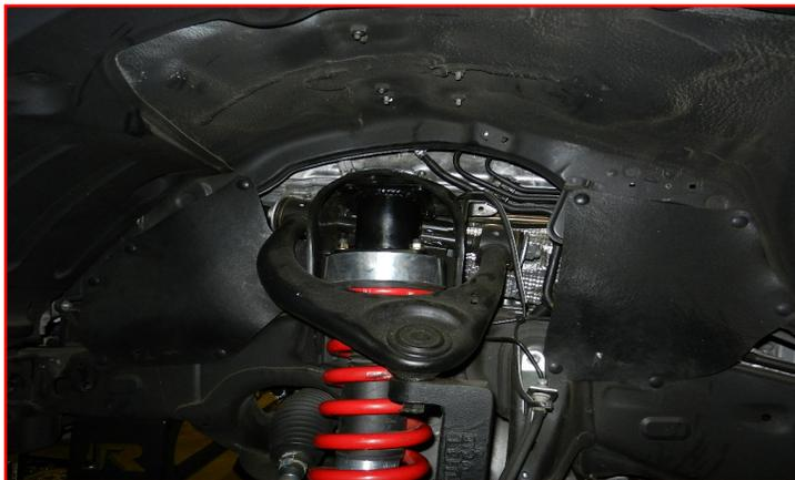
Raise the lower control arm up and install the lower ball joint cradle using the previously **removed hardware** and a drop of thread locker. Torque to **200 ft-lbs**.
