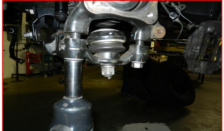
Remove the lower strut and sway bar hardware. Loosen but do not remove the lower control arm cams and let swing out of the way.
