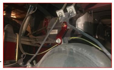
Install the parking brake brackets to the ReadyLIFT extensions (flat brackets) using 5/16" x 1" bolts, washers, and c-lock nuts. Install completed assembly to the axle using factory hardware. Torque all hardware to 5 ft-lbs.
