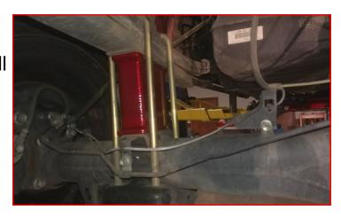
Install the provided u-bolts and nuts. Snug the u-bolt nuts but do not fully tighten at this time. Repeat steps for driver side.
