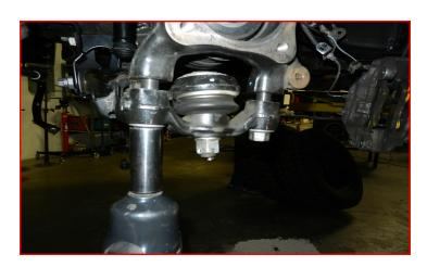
Remove the sway bar from the lower control arm and frame.
