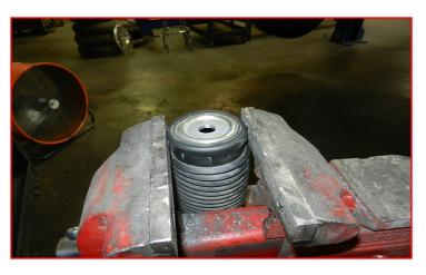
Use a suitable cutting tool and remove the tip of the shock to the first thread. Sand the cut to remove any burs.
