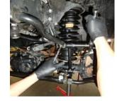
Install new 11" sway bar end links with provide hardware. Note: Head of bolt must face to the inside of vehicle.
