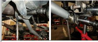
Install the new front lower arm on both sides of vehicle and tighten. The adjustable end should be mounted at the axle and the bend should Point to the center of the vehicle also badges should be legible. 19.
