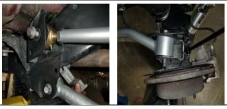
Install the new rear upper arms. Adjustable ends should be installed on frame side and the zerk fittings up on axle side.
