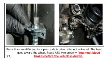
Unbolt rear brake line bracket from bottom of the cab. Bolt the stock bracket to the drop bracket with supplied hardware.
