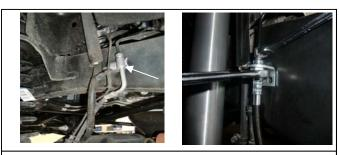
Unbolt the brake line and remove from vehicle. Remove old bracket and install the new Bracket. Bolt the bracket to the frame first, then install the line through bracket. Finish with the push on clip to hold brake line.
