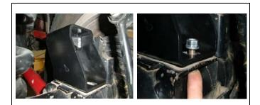
Install new bump with supplied hardware. 39. Bump stop pad should be leaning towards front of vehicle.
