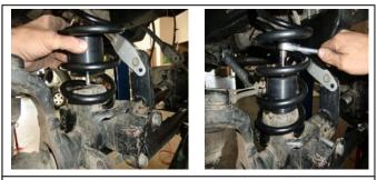
Slip bump pad extension in the coil spring and install as complete assembly. Then tighten the bump extension bolt down using the hardware provided. 21.
