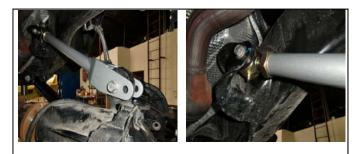
Install the new arm into frame and onto axle, then tighten down. You may need to un-bolt the passenger side to fit the Driver side arm due to length differences 15. from stock arm to ReadyLIFT® arm.
