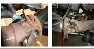
Re-install the front drive shaft to the differential using Locktight. Re-align marks to insure proper drive shaft alignment.
