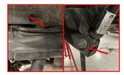
When installing the frame mount of the provided Falcon rear shocks make sure they are positioned in the correct orientation shown in the picture. The Falcon label should be facing the rear of the vehicle.
