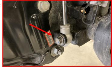
Support the rear axle and remove the factory rear shocks upper and lower mounting hardware.
