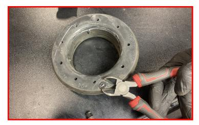
Place the spring isolator onto the provided lift springs.
