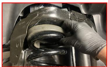
Make sure to align the end of the coil to the corner of the axle's spring perch to maintain the correct spring position.
