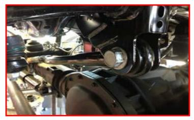
Loosen the rear radius arm bolt.
