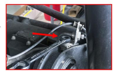
Remove the 13mm ABS and Brake line lower bracket bolt from the axle.
