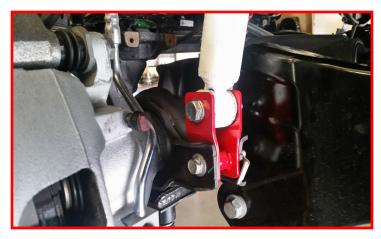
Remove stock rear shocks and install aftermarket rear shocks that are provided in this kit. Do not tighten hardware at this time.
