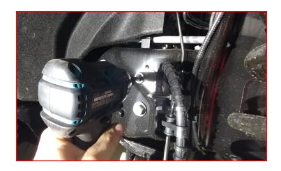
Remove the brake line bracket at the axle. Retain the factory hardware.
