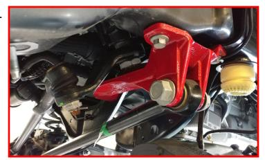
Install the provided sway bar drop brackets to the frame using factory hardware.
