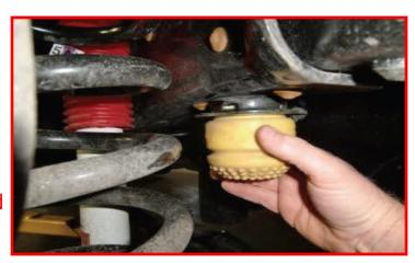
Mark a line parallel to the frame across the edge of the outer lip of the bump stop mount .
