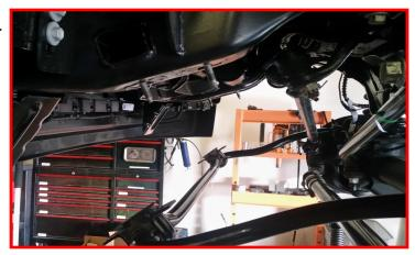
Lower the axle enough to remove the front springs. Install the replacement spring using factory rubber isolator. Raise the axle enough to hold the spring assembly in place.
