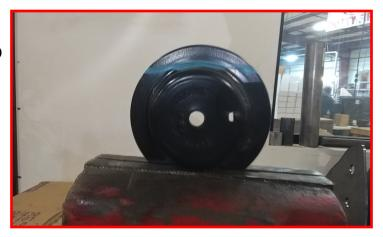
Using a suitable cutting tool, trim off the marked edge. Paint the cut surface to prevent corrosion.
