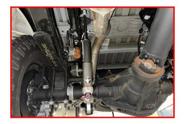
Install the wheels and lower the vehicle to the ground. Torque the lug nuts to the wheel manufacturers specs. Jounce the suspension a few times to settle to the new ride height.
