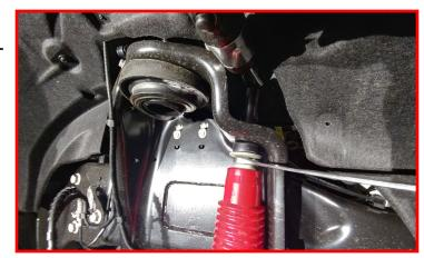
Remove the sway bar from the frame. Retain factory hardware.
