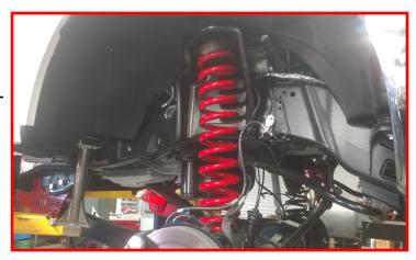
Remove track bar from the track bar bracket. Let the track bar hang out of the way. Retain factory hardware.
