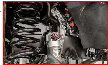
Remove stock rear shocks and install the Falcon rear shocks that are provided in this kit. Do not tighten hardware at this time.
