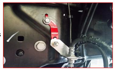
Remove the factory bump stop by pulling it out of its mount. Remove the mount from the frame and discard factory hardware.
