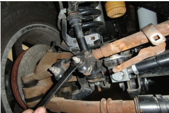
Loosen (2) collar bolts and lube threads of steering linkage
