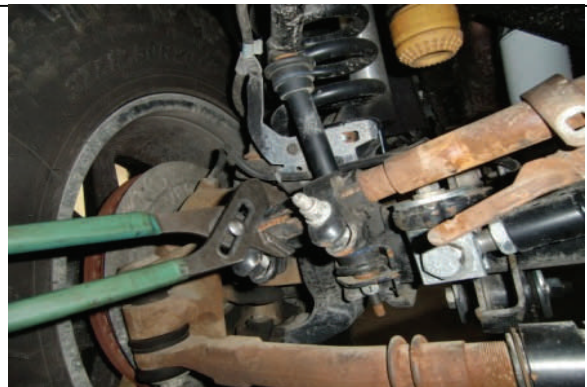
Adjust collar to straighten steering wheel
