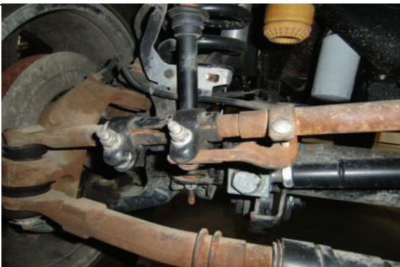
Tighten up hardware and replace keeper bolt
