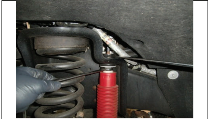
Remove front shocks. Note: Longer shocks required
