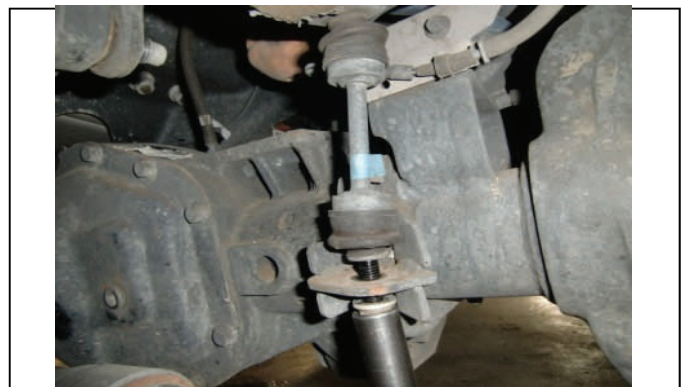
Disconnect both front sway bar end links
