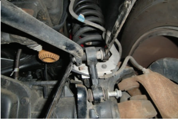
Lower vehicle, reconnect sway bar end links
