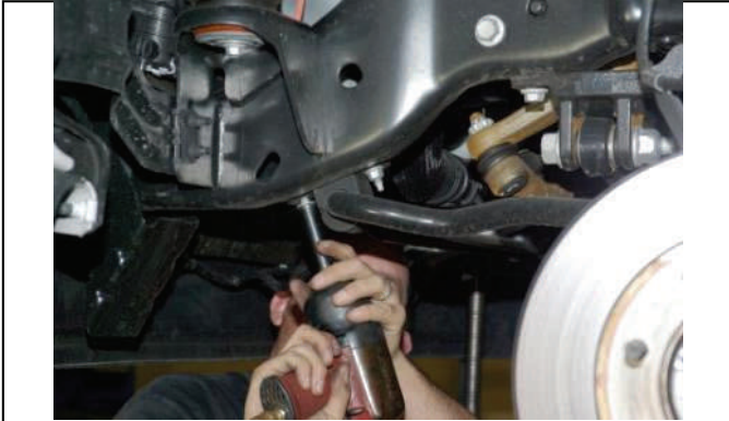
(11-up) Disconnect sway bar at frame and lower
