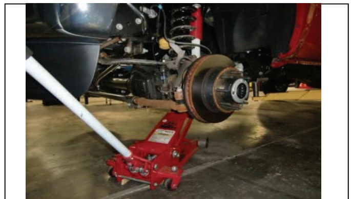
Support front axle with floor jack(s).
