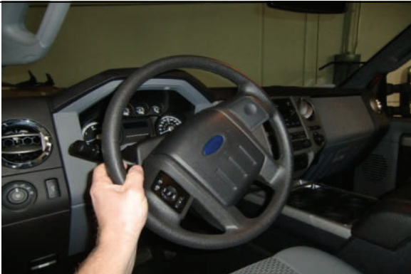
Straighten steering wheel steps, Unlock steering wheel
