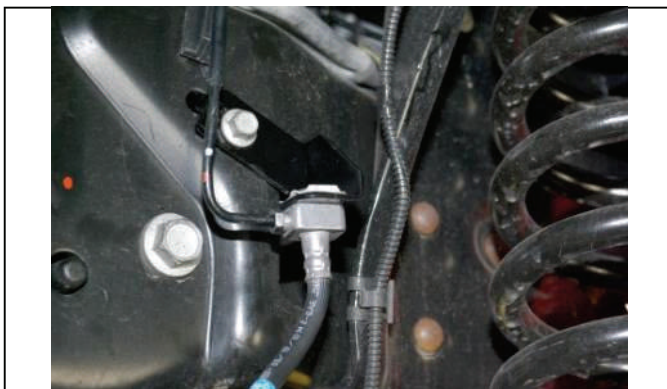
Reinstall block into bracket with retaining clip.
