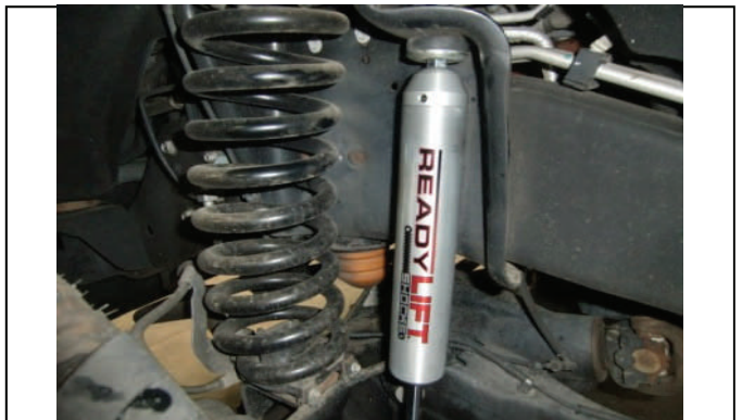
Install and tighten new shock kit 99-2095F
