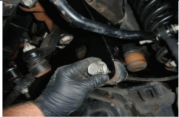
Reconnect track bar to new drop bracket w/ OE hardware.
