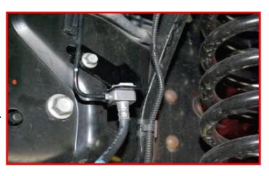
2017 - UP front brake line: Install the ReadyLIFT brake line bracket to the factory brake line using 5/16" x 3/4" bolts, washers, and nuts. Install the bolt facing outwards. Torque to 10 ft-lbs. Gently pull the metal brake line down while lining up the ReadyLIFT bracket to the original holes in the frame. Install using factory hardware. Torque to 5 ft-lbs.
