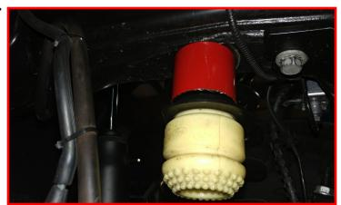
Install the provided shocks using the factory lower hardware and provided upper hardware. Do not tighten at this time.
