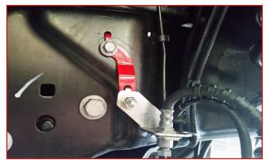
Remove the factory bump stop by pulling it out of its mount. Remove the mount from the frame by pulling it out of its mount.
