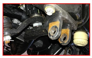
Install the ReadyLIFT track bar bracket to the frame using factory hardware. Torque to 95 ft-lbs. Install the track bar to the ReadyLIFT bracket using factory hardware. Lower the vehicle to the ground for torque. Torque the track bar hardware to 250 ft-lbs.
