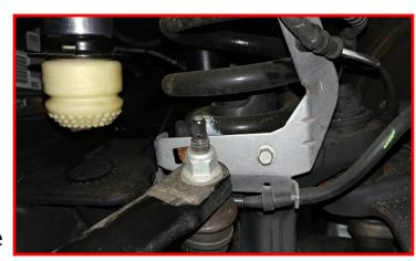
2011 - 2016 front brake line: Install the ReadyLIFT brake line drop bracket to the frame using the factory hardware. Torque to 5 ft-lbs. Note: The ReadyLIFT brackets look like the factory brackets except the locating flat is 180 degrees off. Install the brake line block using the factory clip. Reconnect the ABS line. Do not clip back to fender liner.
