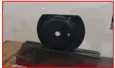
Install the supplied bump stop spacer and factory bump stop mount to the frame using M8 bolt and washer. Make sure the cut edge faces to the outside of the vehicle
