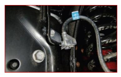
Loosen the metal line ferrule nut at the rubber brake line block. Rotate the fitting down 180 degrees from factory and tighten. Remove the bracket from the frame.
