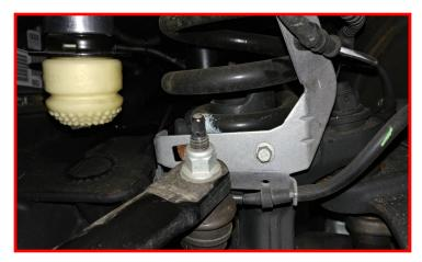
Install the supplies brake line drop bracket to the frame using the factory hardware.
