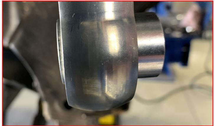
Swing lower control arm up into place and install the coil-over rod end into the control arm pocket using the factory strut hardware.
