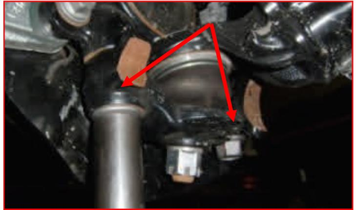
Remove lower strut mounting hardware. Retain the factory hardware.
