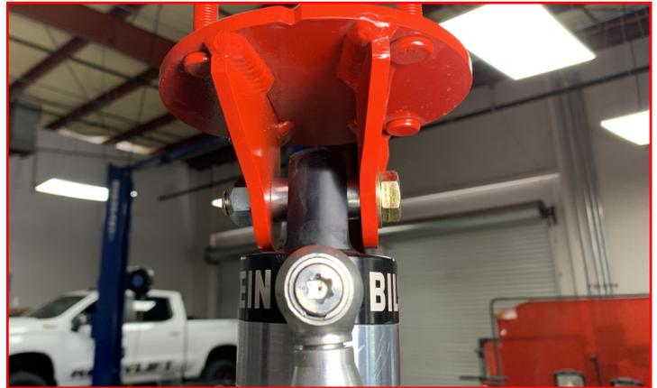
Note: Ensure that the top hat is installed with the notch facing the reservoir banjo fitting and the offset towards the frame (as shown in picture).
