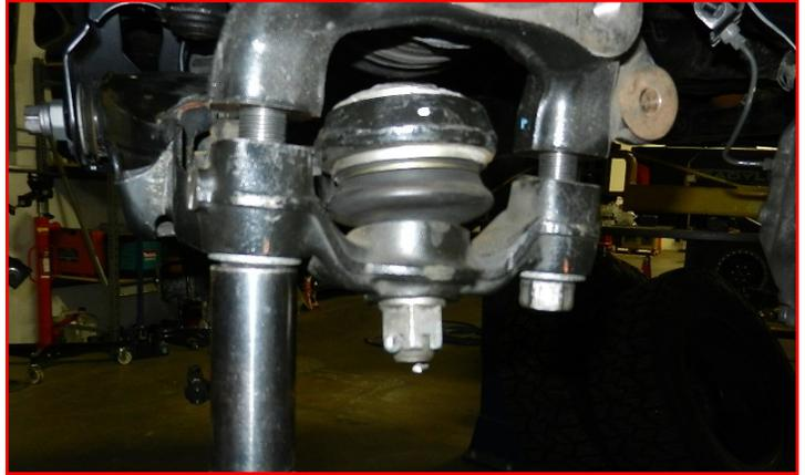
Install the outer tie rod end to the knuckle using the **factory hardware**.
