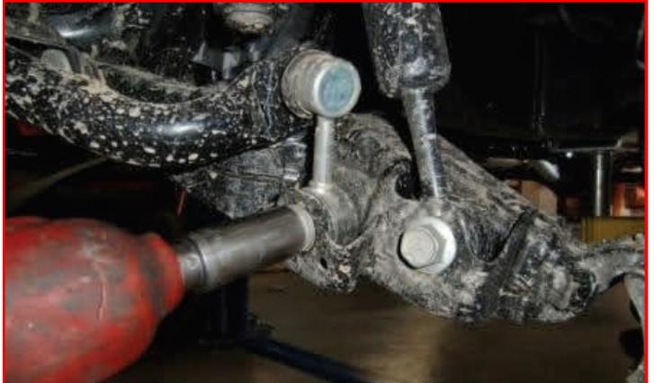
Remove the cotter pin and outer tie rod end nut. Strike the tie rod end boss with a dead blow hammer to dislodge the taper.
