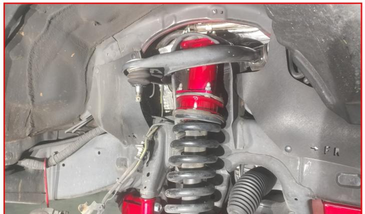
Notch the lower control arm strut pocket as shown. Radius the back edge following the pocket profile. This is for clearance on the coil-over rod end at full droop.
