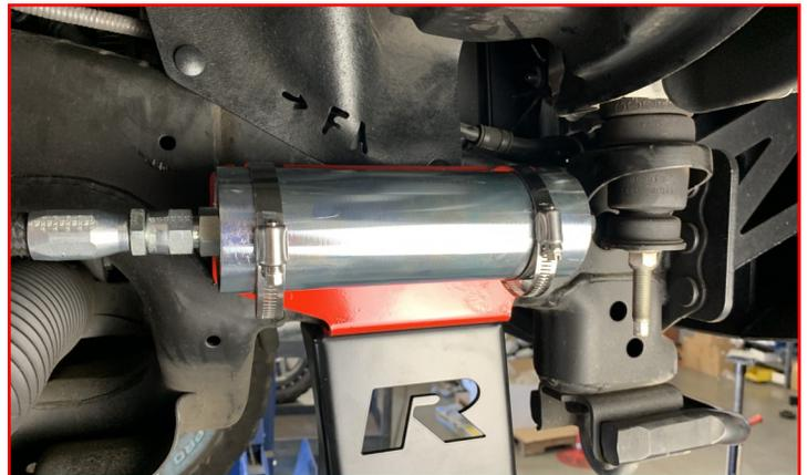
Install the lower ball joint cradle using the **factory hardware**. Add a drop of thread locker to the lower mounting hardware.
