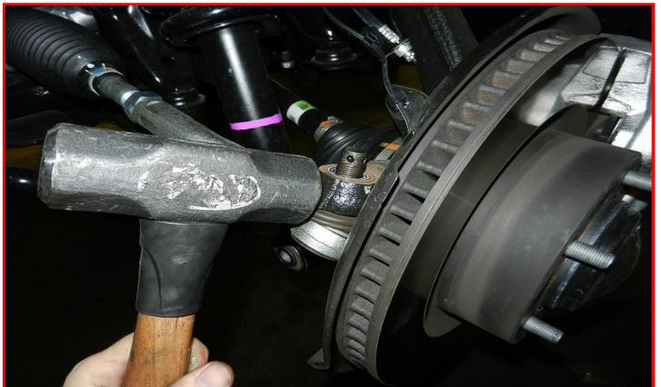
Support the lower control arm with a suitable jack. Remove the **lower ball joint cradle bolts** from the knuckle. Be sure to retain the factory bolts.
