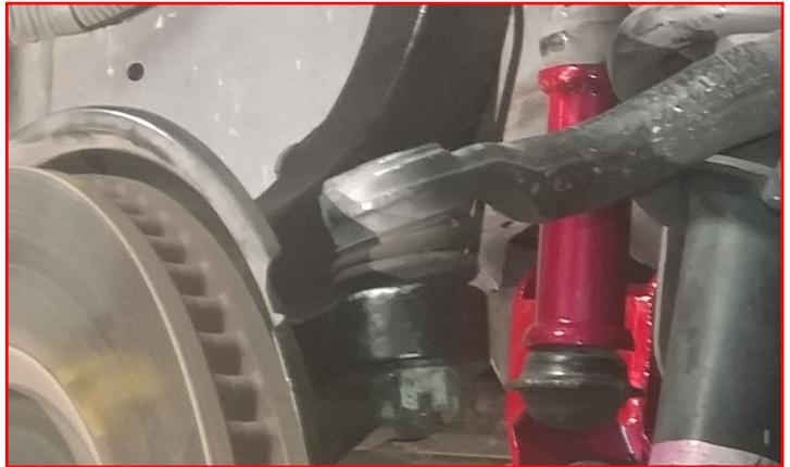
Install the sway bar links to the lower control arms using the **factory hardware**.
