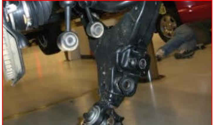
Remove the upper strut mounting hardware. Discard the factory mounting hardware.
