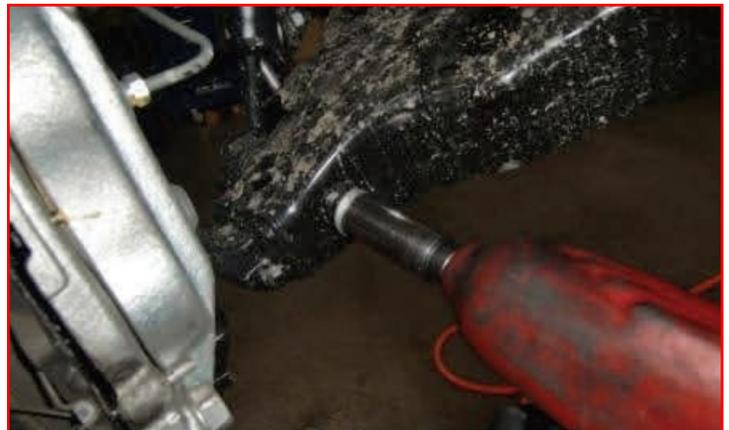
Support the knuckle/hub assembly with a suitable jack. Swing the lower control arm down and out of the way to aid in the removal of the strut assembly.
