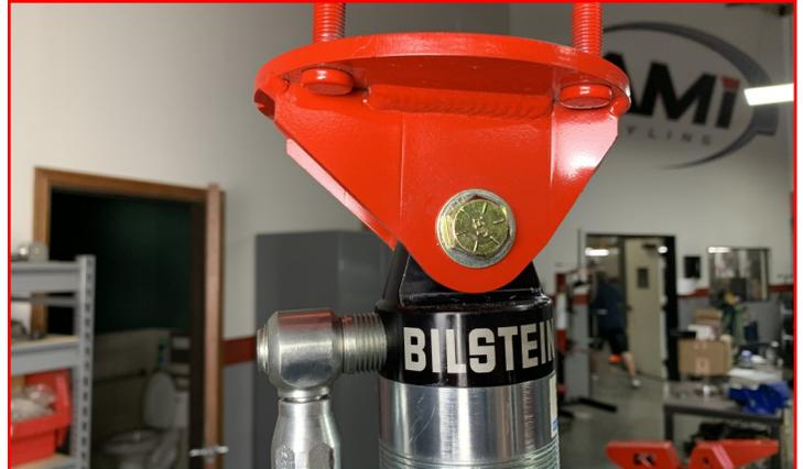
The coil-over come preset for the 8" kit. However, fine tuning may be necessary to achieve the correct right height.
