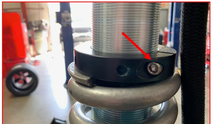
**Note:** If coil-overs are being installed on the 6" lift kit, the preload collar will need to be adjusted for that application.
