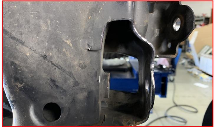
Install the supplied coil-over top hat adaptor using (2) coil-over top cap spacers, 1/2 bolt, locking nut and washers.
