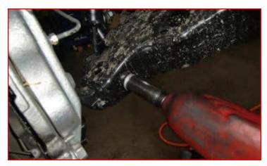
Support the knuckle/hub assembly with a suitable jack. Swing the lower control arm down and out of the way to aid in the removal of the strut assembly.
