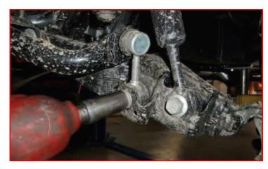
Remove the cotter pin and outer tie rod end nut. Strike the tie rod end boss with a dead blow hammer to dislodge the taper.
