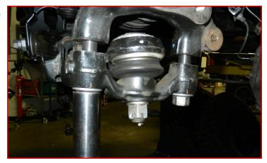
Install the outer tie rod end to the knuckle using the factory hardware.
