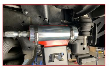
Install the lower ball joint cradle using the factory hardware. Add a drop of thread locker to the lower mounting hardware.
