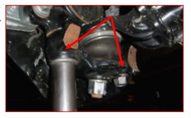
Remove lower strut mounting hardware. Retain the factory hardware.
