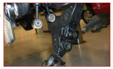
Remove the upper strut mounting hardware. Discard the factory mounting hardware.
