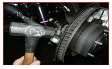
Support the lower control arm with a suitable jack. Remove the lower ball joint cradle bolts from the knuckle. Be sure to retain the factory bolts.
