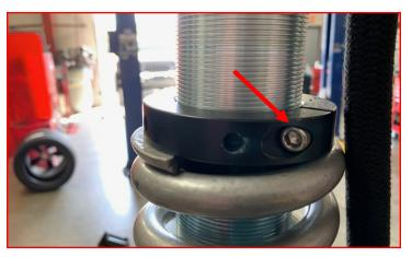
Note: If coil-overs are being installed on the 6" lift kit, the preload collar will need to be adjusted for that application.
