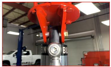
Note: Ensure that the top hat is installed with the notch facing the reservoir banjo fitting and the offset towards the frame (as shown in picture).
