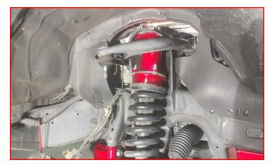
Notch the lower control arm strut pocket as shown. Radius the back edge following the pocket profile. This is for clearance on the coil-over rod end at full droop.
