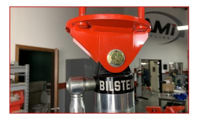
The coil-over come preset for the 8" kit. However, fine tuning may be necessary to achieve the correct right height.
