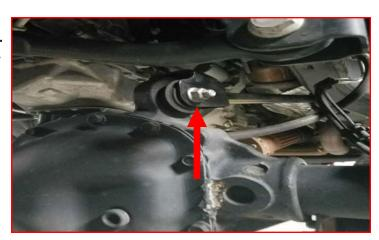
Loosen but do not remove the lower control arm bolt at the axle.
