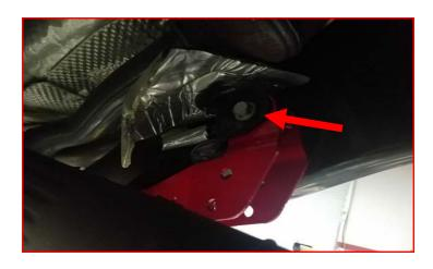
Install the ReadyLIFT control arm bracket to the lower control arm pocket using the factory hardware. Do not tighten at this time.
