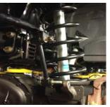
Install extended sway bar end links and adapter brackets.
