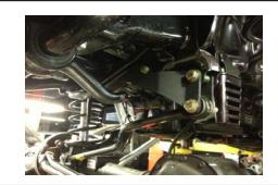
22. Install the track bar into the drop bracket.
