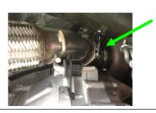
Once arms are installed, re-install the exhaust and tighten all corre-16. sponding mounting points and hardware.
