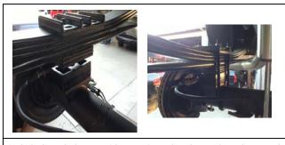
Unbolt the u-bolts one side at a time, then lower the axle enough to install the block. Install new u-bolts and torque down.
