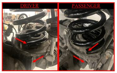
Remove the factory shocks upper mounting nut and install the provided Falcon front shock into the upper frame mount.
