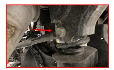
Loosen the rear track bar at the axle side.
