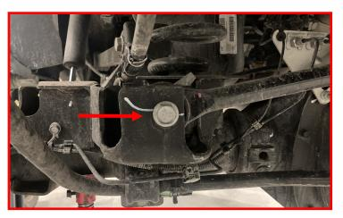
Remove the factory rear shocks upper and lower mounting hardware.
