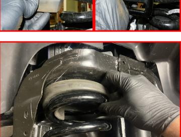
Make sure to align the end of the coil to the corner of the axle's spring perch to maintain the correct spring position.
