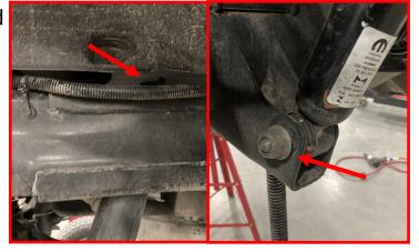
Lower the axle down until you have enough room to install the provided rear spring spacer.
