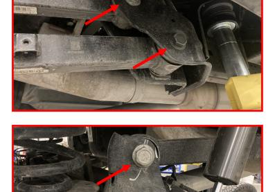
Loosen the rear track bar at the frame side.
