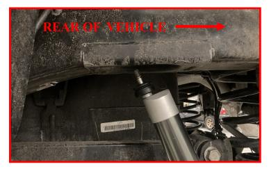
Install the rear Falcon shock into the axle mount using the factory hardware.
