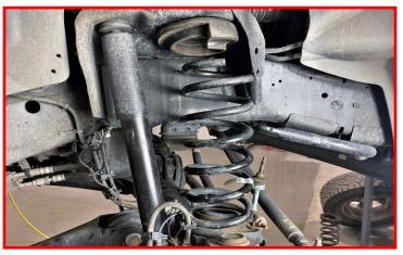
Remove the factory spring isolator.
